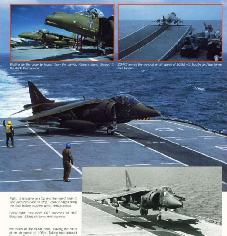
two-thirds of the 600ft deck, leaving the ramp at an air speed of 105kt. Taking into account the vessel's progress into wind, that represents a typical ground speed of around 70kt.
