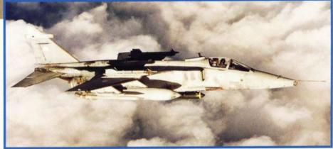
The Jaguar's self-defence armament has been provided by AIM-9L Sidewinders mounted on overwing rails since 1990.
