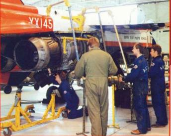
Jaguar T2A XX145 undergoing an engine change, with its starboard Adour about to be removed.
