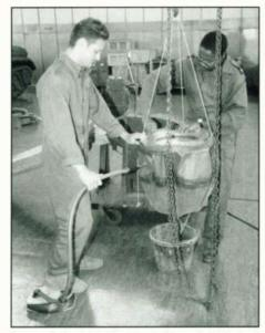
Corporal Paul Braithwaite (left) and SAC Andy Cole test a critical component, the 14-inch valve, for leaks. The valve is mounted above a bag of pressurised air and covered with a layer of water. Note the lino floor and soft shoes.
