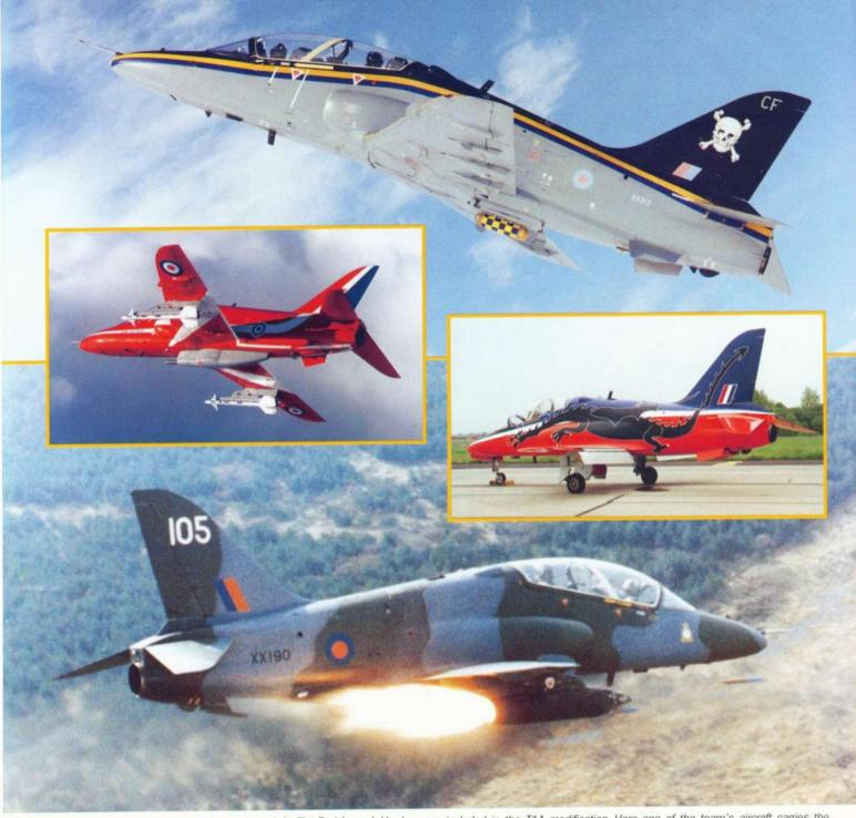
Top: No 100 Squadron Hawk T1A. BAe Inset left: The Red Arrows' Hawks were included in the T1A modification. Here one of the team's aircraft carries the centreline gun pod and AIM-9L Sidewinders. BAe Inset right: Specially painted Hawk T1A – St Athan Station Flight. PRM Above: Hawk T1A firing SNEB rockets. BAe
