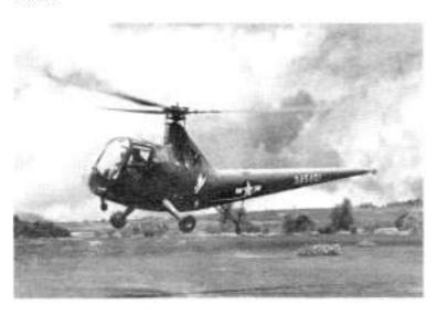
The R-6A entered production late in the war. It was slightly larger and more powerful than the R-4A. Its design was more refined. The R-6A had a gross weight of 2,623 pounds, could cruise at 65 knots, attain a speed of 82 knots, and carry a 589-pound payload. It was 38 feet, 3 inches long and had a 245-horsepower Franklin engine.
