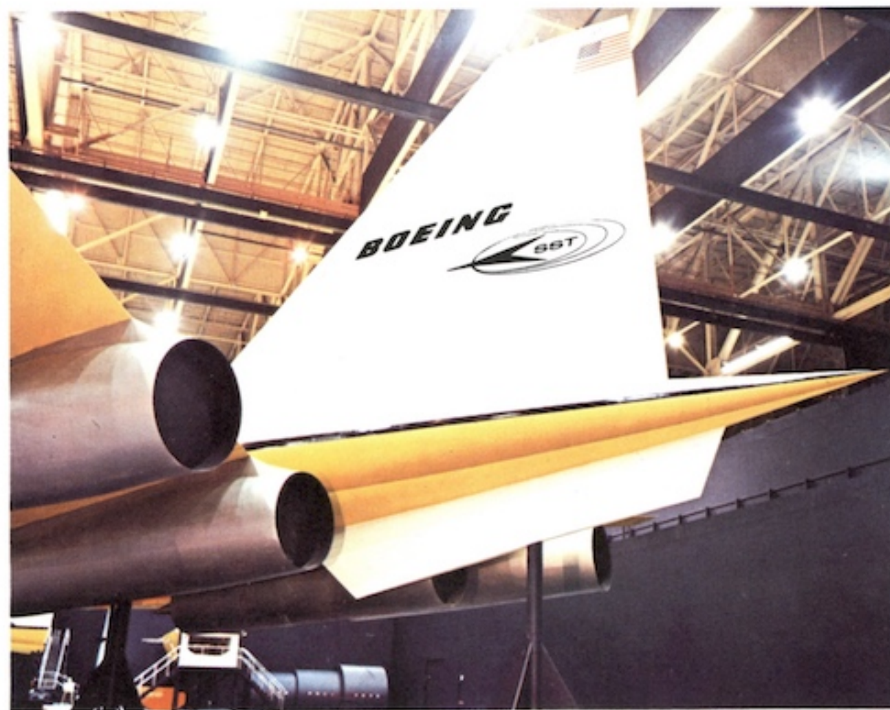
Giant tail section towers 53 feet above floor of high bay
