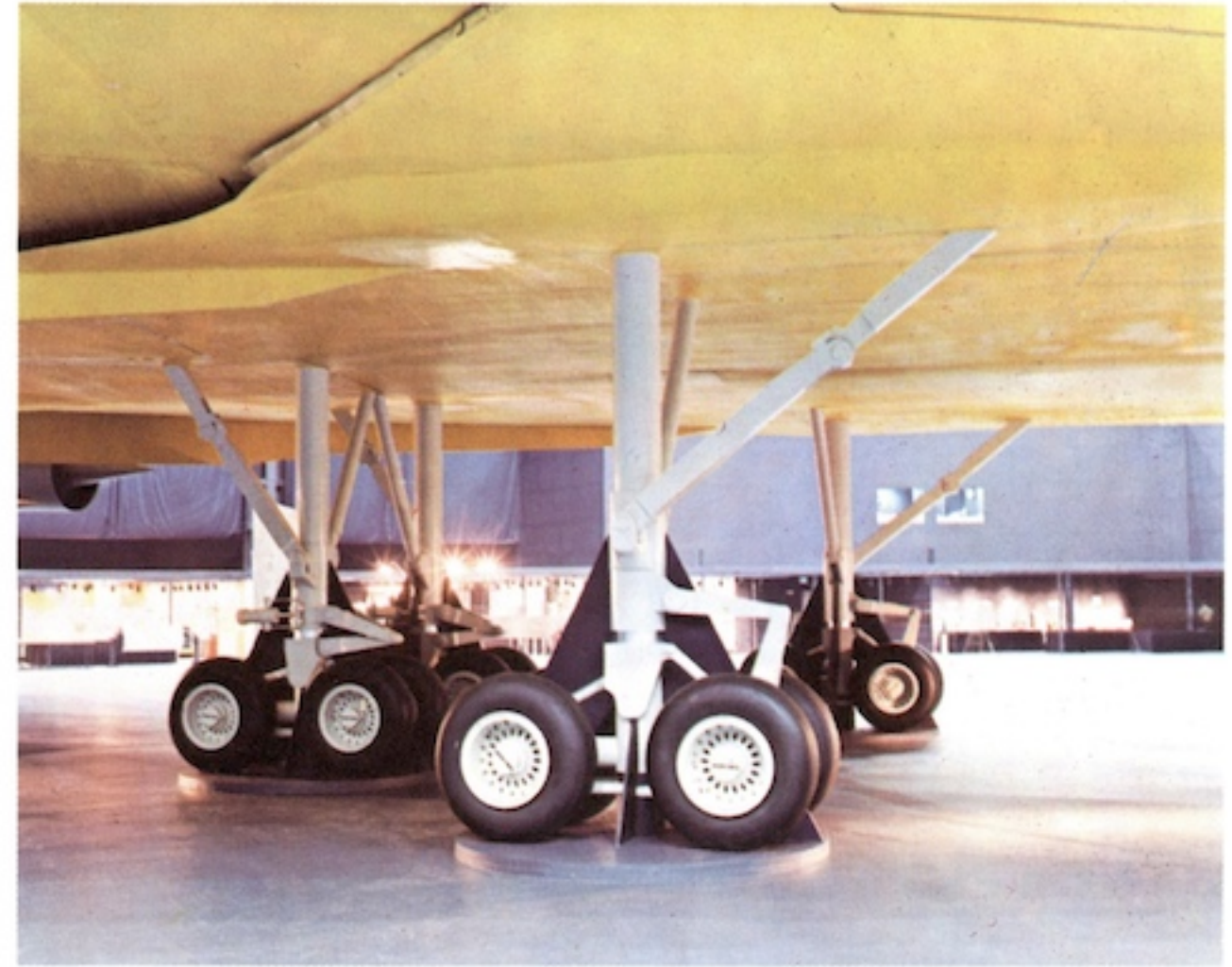
Four post main landing gear ride on 16 individual wheels
