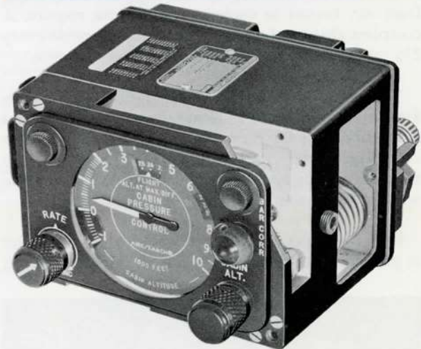
Above: Cabin pressure regulator outflow valve. Below: Cabin pressure regulator outflow control and indicator.
