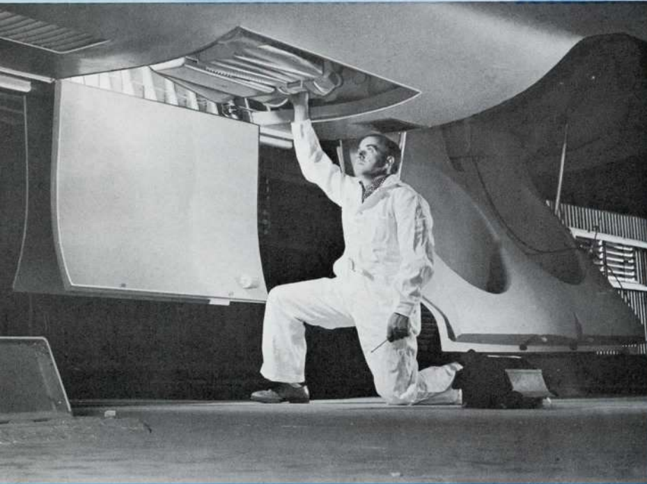
The entire Freon system is packaged so that it may be removed for servicing.
