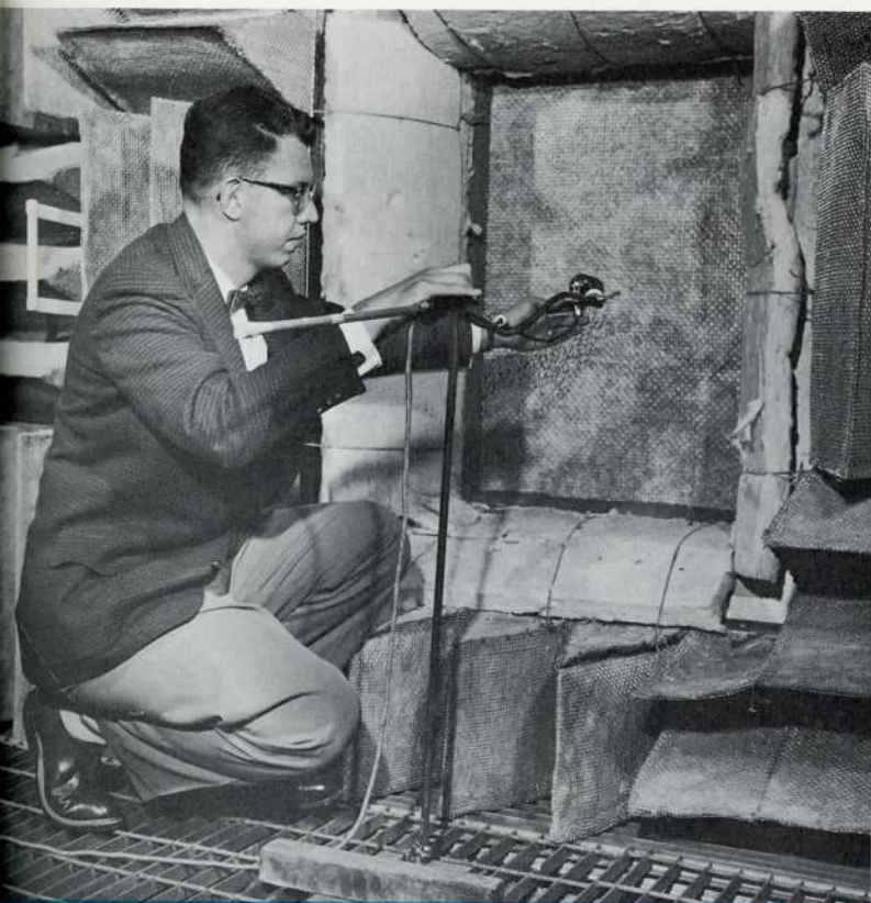
Noise escaping through a fuselage test panel is measured in the Acoustic Laboratory's anechoic chamber.
