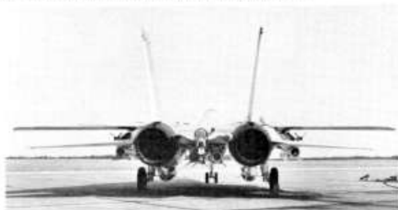
(Above) A Tomcat reveals its large intake area. The intakes are two-dimensional with a single mode of variable geometry through the use of compression ramps visible inside the tops of the intakes. (Below) The No 2 flight test aircraft, showing a spin chute housed between the tailpipes. In addition to six Phoenix and two Sidewinder missiles, this aircraft is carrying two fuel tanks under the engine nacelles.
