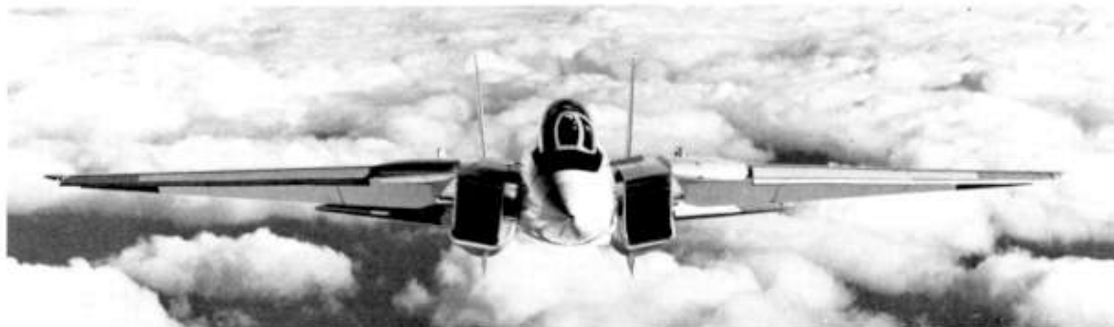
(Above) A Tomcat reveals its large intake area. The intakes are two-dimensional with a single mode of variable geometry through the use of compression ramps visible inside the tops of the intakes. (Below) The No 2 flight test aircraft, showing a spin chute housed between the tailpipes. In addition to six Phoenix and two Sidewinder missiles, this aircraft is carrying two fuel tanks under the engine nacelles.
