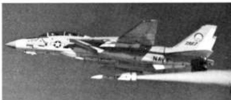
(Above) A fine portrait of the F-14A No 2 with its full armament load of six AIM-54 Phoenix missiles and two AIM-7 Sidewinders plus two drop tanks. (Below left) The No 4 Tomcat fires a Phoenix during early weapons trials at the Naval Missile Center, Point Mugu.
