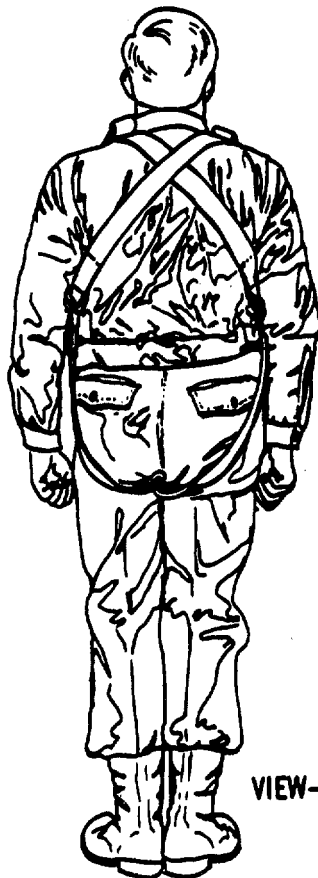
Figure 1-2. The 28-Foot Chest Personnel Parachute.
