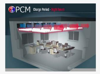
Passive cooling takes advantage of the naturally occurring temperature swing caused by day & night. The excess coolth available in the night can be stored in the PCM, which is then released during the day, absorbing internal and solar heat gains.
