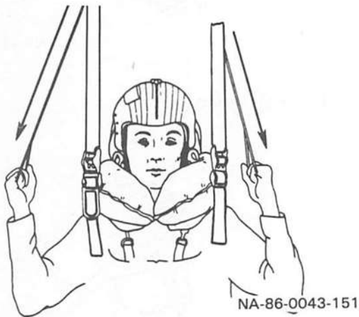
(a) To deploy four-line release, locate parachute control lanyards on the inside of rear risers and pull down sharply.
