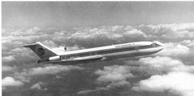
Continental Airlines' fleet of Boeing 727s are powered by Pratt & Whitney's JT8D engines, the most widely used engine in commercial aviation history.
