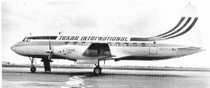
T.I.A.'s selection for the DC-3 successor was the Convair 600. This was basically the Convair 240, but re-engined with Rolls-Royce Dart turboprops. It is seen here in Texas International colors.
