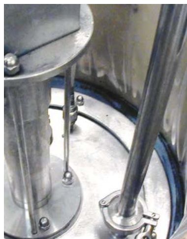
The Kecol Follower plate system will also work on 200 litre Open Top Drums fitted with an aseptic bag – wiping the bag clean
