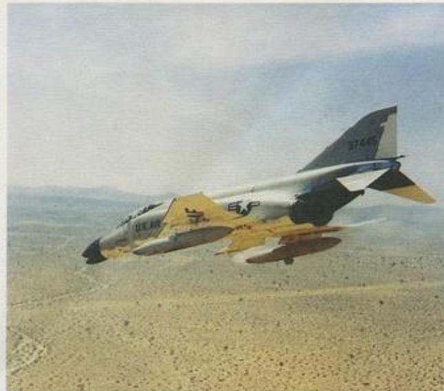
An early production F-4C (USAF serial number 63-7445) makes a strafing run with one of its pod-mounted M61 Vulcan rotary cannons. The Air Force developed these because the Phantom had no internal guns.
