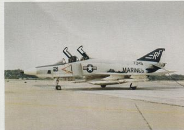
All RF-4Bs were recently reassigned to a single squadron, VMFP-3. One of FP-3's aircraft is seen here carrying several Elint and ECM pods.
