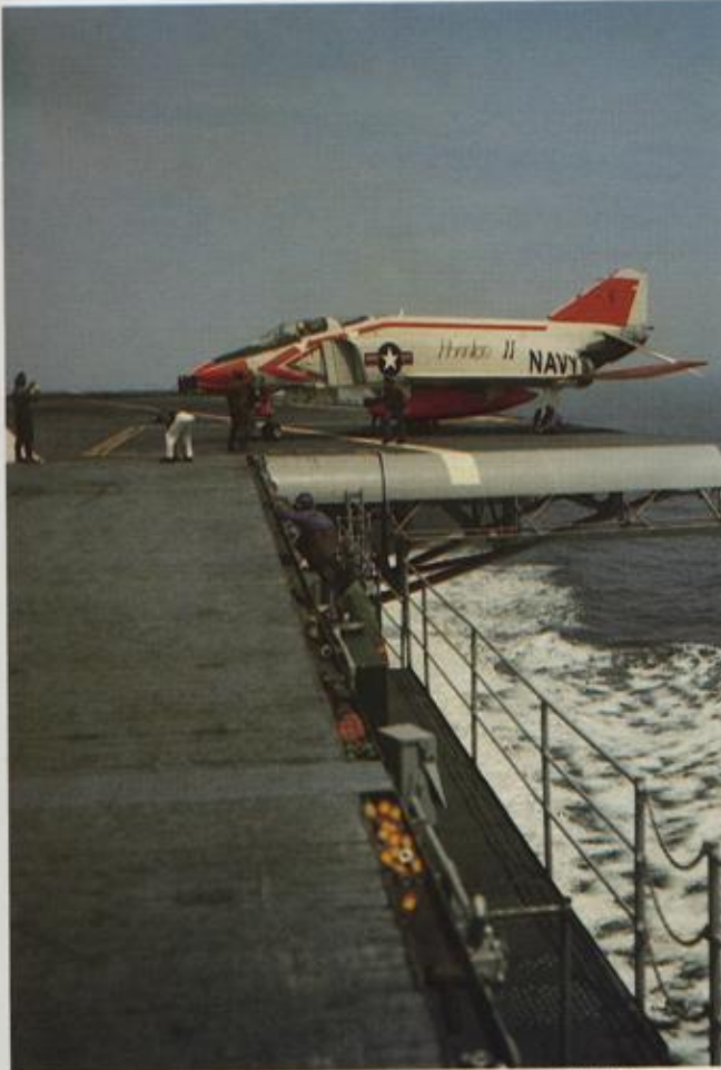
Carrier suitability trials were conducted with the sixth F4H-1 (Bureau Number 143391) aboard the USS Independence beginning 15 February 1960.
