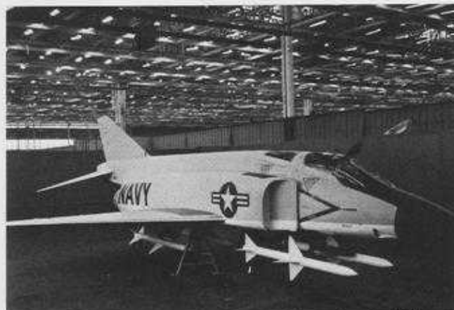
The mock-up after reconfiguration into the F4H-1, with revised inlets, second cockpit, and drooped stabilizer. Sparrow missiles were to be launched from extendable rails.
