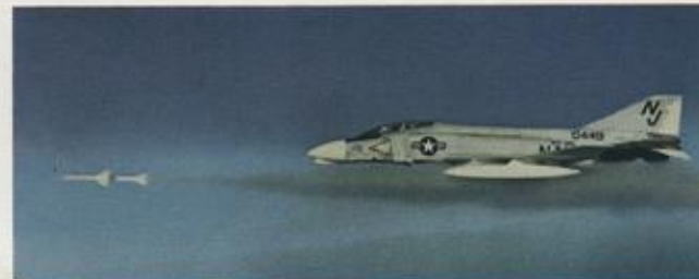
Primary armament of the Phantom in its original fleet-defense role has been the radar-guided AIM-7 Sparrow air-to-air missile.
