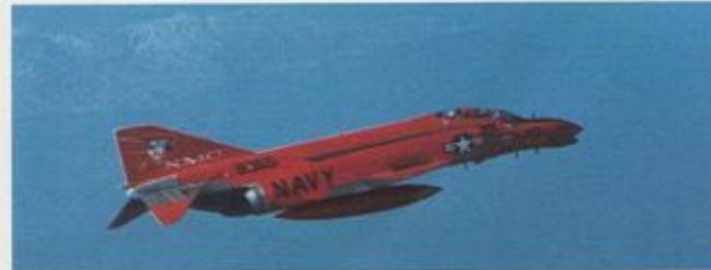
One recent development in the Phantom program was the conversion of several Navy F-4B airframes into QF-4B drones for use by the Naval Missile Center at Pt. Mugu, California.
