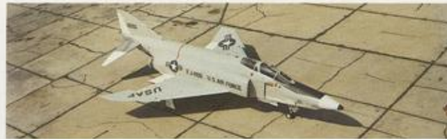
Number 266 entered production as a Navy F4H-1 airframe and was modified during construction into the YRF-4C reconnaissance prototype.
