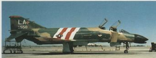
Several 58th Tactical Fighter Training Wing F-4Cs had bright stripes painted on fuselage and wings to add to visibility for training purposes.
