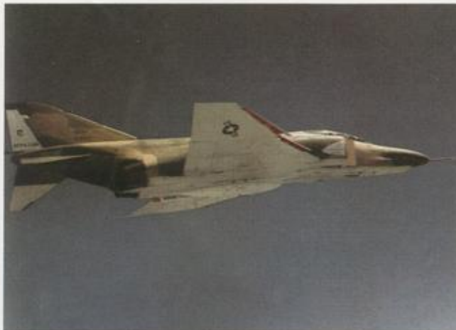
The next milestone for Number 266 was "Project Agile Eagle," the flight testing of leading edge maneuvering slats, beginning in June 1969. The success of these tests led to the installation of maneuvering slats on all F-4E and F-4F Phantoms. This aircraft also served as a test bed for a beryllium rudder.
