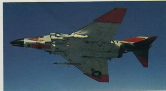
An early F4H-1, Bureau Number 146817, shows maximum air-to-air armament of six Sparrows during missile system evaluation.
