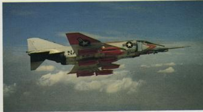
Number eleven F4H-1 (Bureau Number 145310) demonstrated the Phantom's prodigious weight-carrying abilities by lifting and dropping twenty-two 500-lb. bombs.
