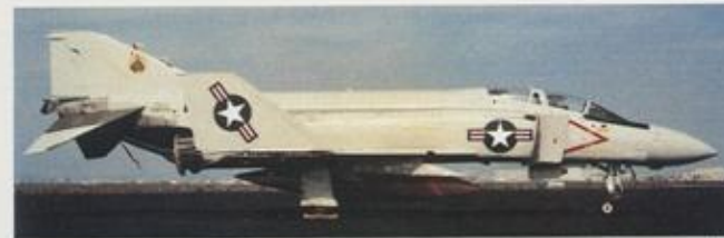
The Navy has begun a similar SLEP to modernize over 250 F-4Js, the first of which is shown here. This program will result in the F-4S model, equipped with leading edge maneuvering slats.
