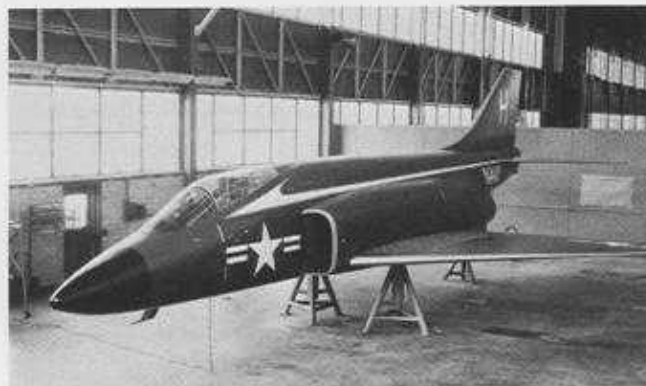
McDonnell's company-financed mock-up of the Phantom-to-be, then identified as the F3H-G. Note particularly the single cockpit, the unbroken lines of the wing, and the undrooped tail.
