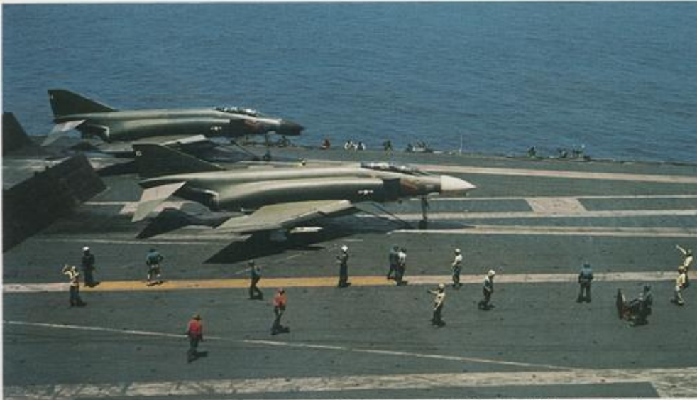
Adorned in experimental camouflage paint, two VF-213 Phantoms, an F-4G and an F-4B, prepare for launching from the USS Kitty Hawk off Vietnam in 1966. Twelve Navy F-4Bs were modified into "G" models by incorporation of a two-way digital data link and an approach power compensation system, both standard in the later F-4J.
