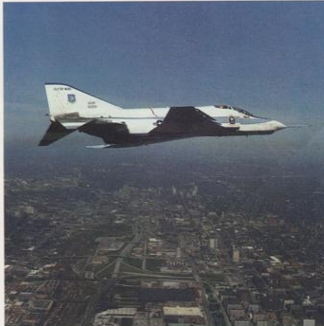
A "Fly-by-Wire" control system was installed in Number 266, and a distinctive color scheme was applied to the airplane for this flight test program, which commenced on 29 April 1972.
