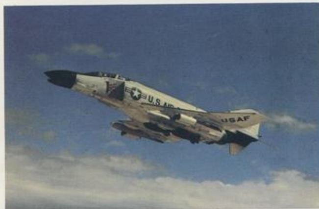
One of the F-110As successfully evaluated by the Air Force displays a variety of air-to-ground ordnance — bombs, rockets, and napalm.
