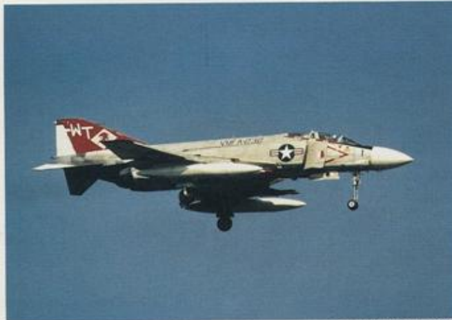
Among the numerous USMC squadrons to operate the F-4J is VMFA-232. The F-4J, featuring uprated J79-10 engines, aerodynamic improvements, and a new, integrated missile control system (AWG-10), superseded the "B" in production for the Navy in 1966.
