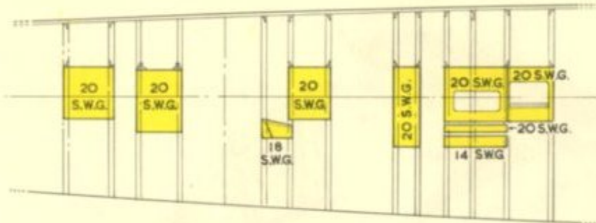
BOMB BAY INTERNAL SKINS BETWEEN BOMB ARCHES
