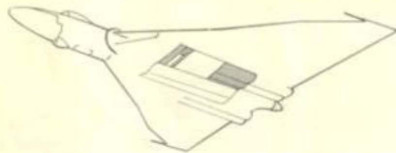
Fig. 323A. Centre section skinning - Bottom surface
