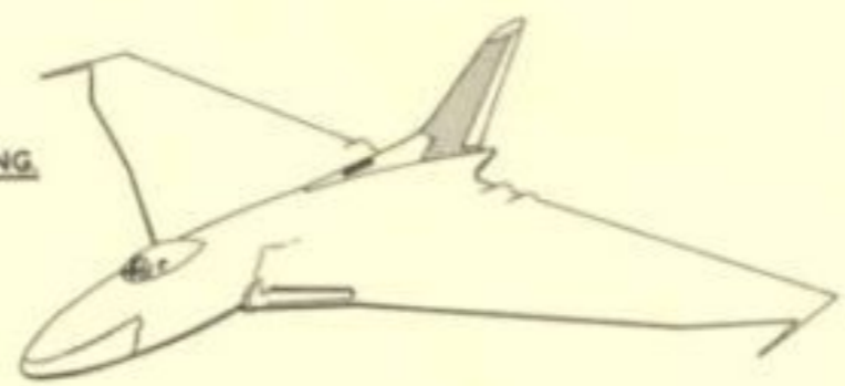
Fig.404 - Fin skinning RESTRICTED
