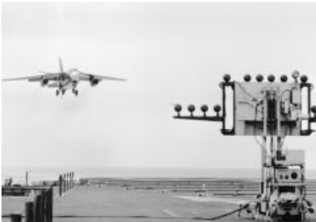
Equipment development encompasses all phases of Naval Aviation, mirror landing system brings in A3D 698382
