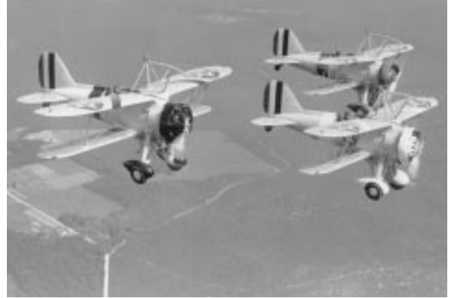
Curtiss F9C-2s with airship hoop-on gear 441982
