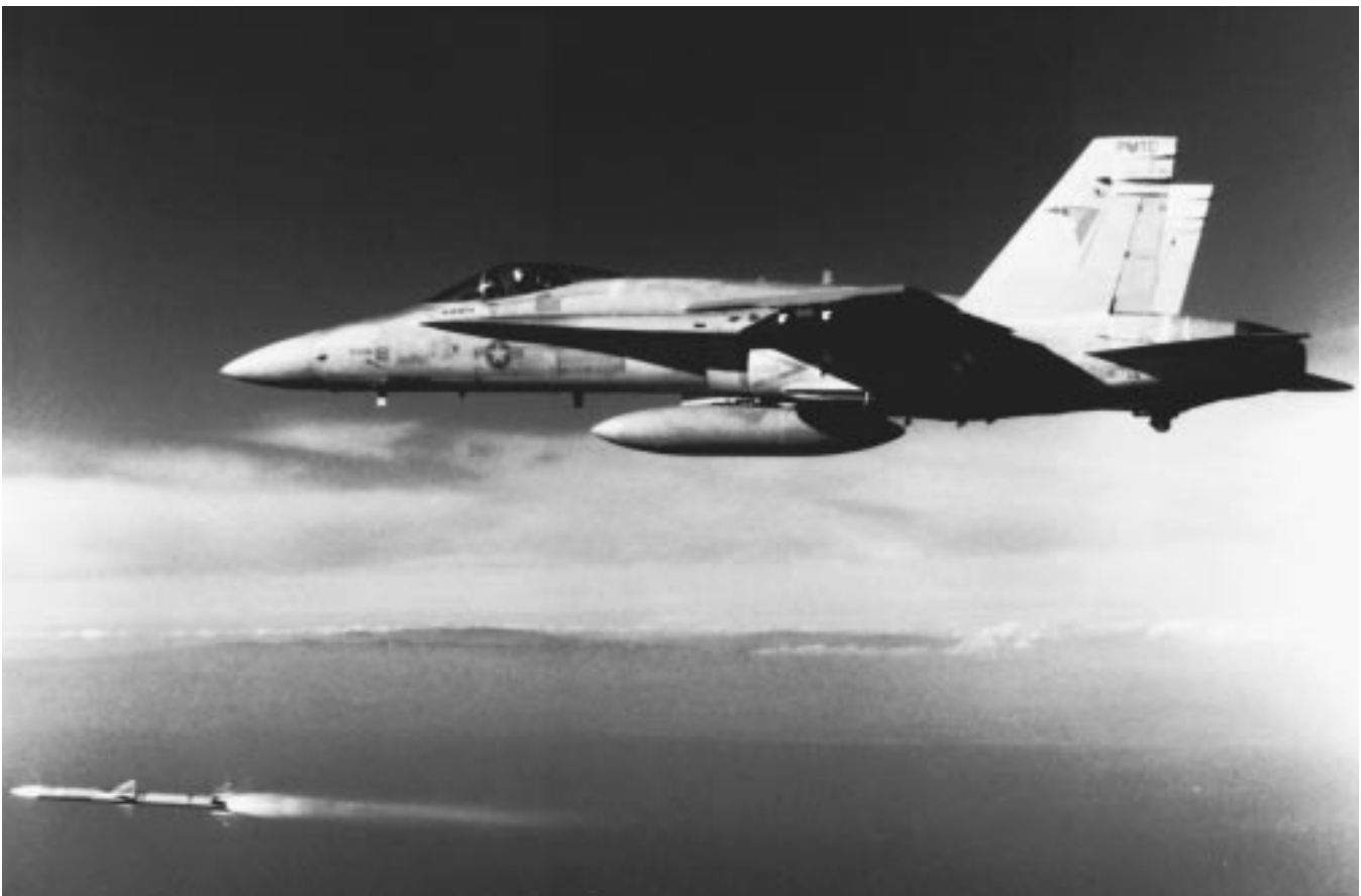
After a launch from an F/A-18 Hornet, the AMRAAM streaks toward its target during testing at Pacific Missile Test Center, Point Mugu, Calif.
