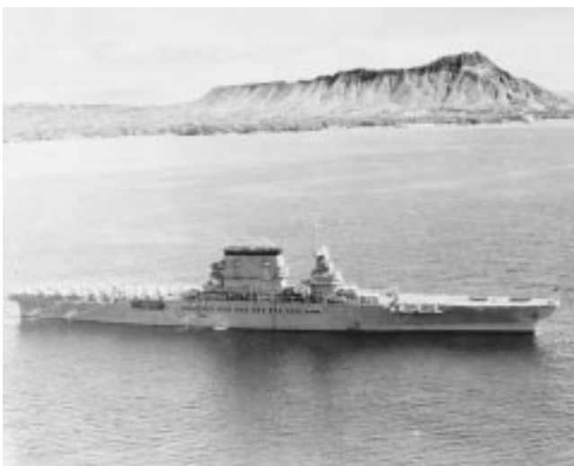
Lexington off Diamond Head. Lexington and Saratoga were constructed on battle cruiser hulls 416531
