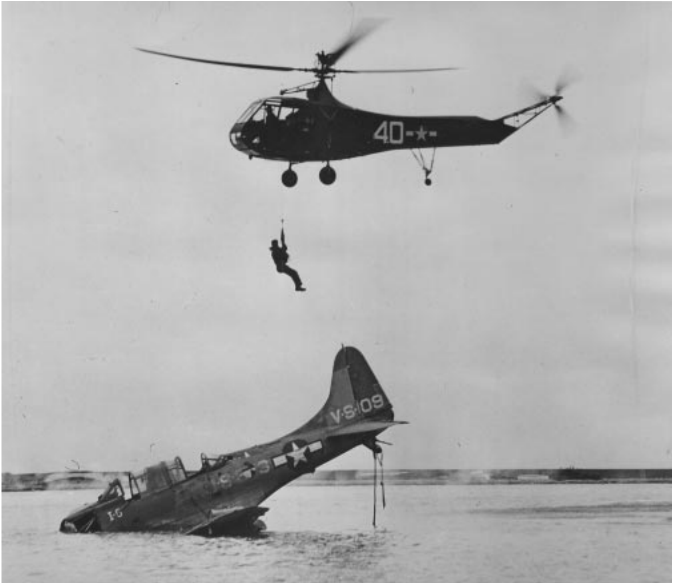
The Navy and Marine Corps early helicopter, the HNS-1, demonstrates its air-sea rescue capabilities by retrieving a pilot from his ditched SBD, CG-3649.
