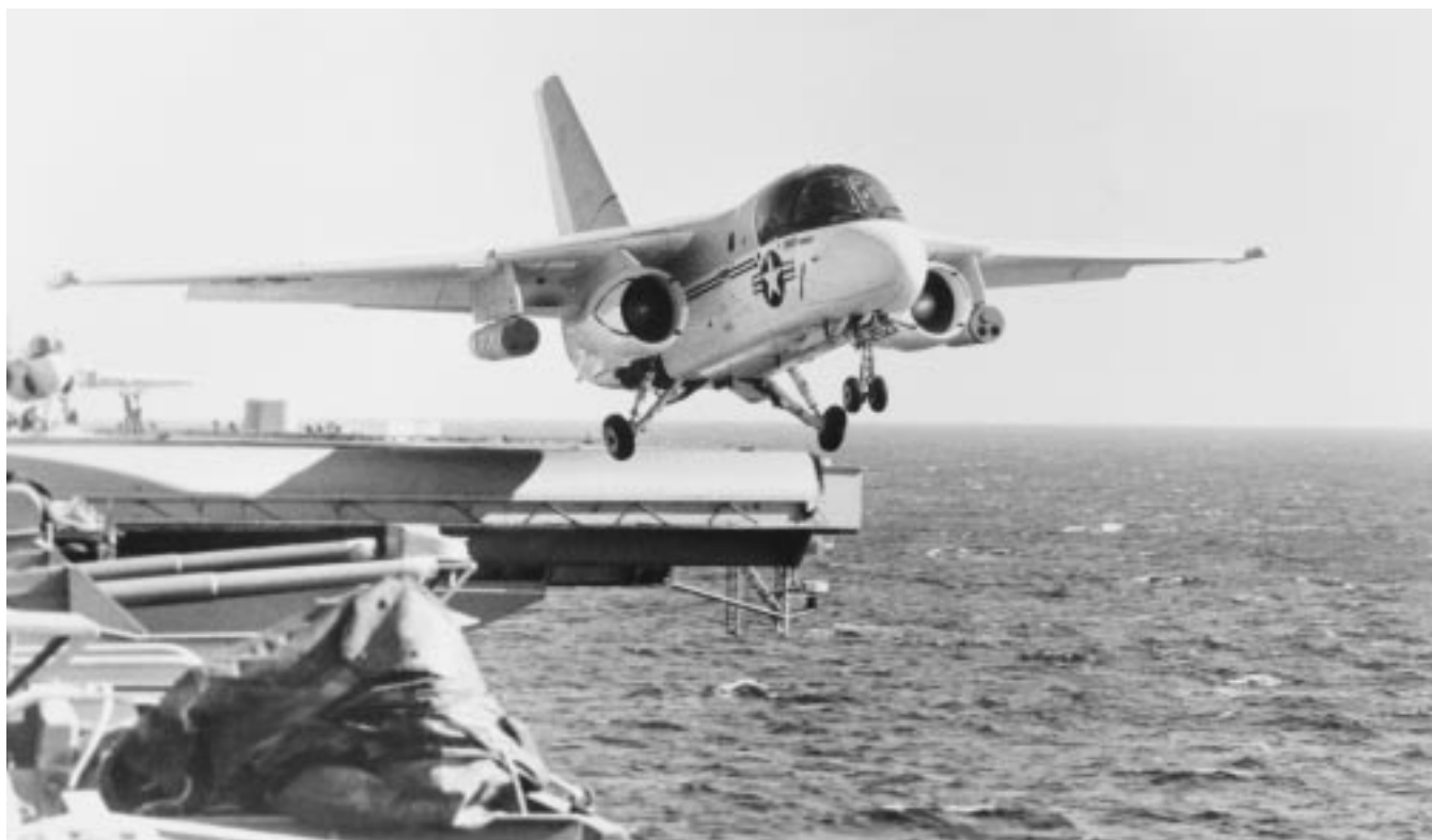
The S-3A Viking making its first catapult launch from Forrestal as part of its initial carrier suitability tests C121073
