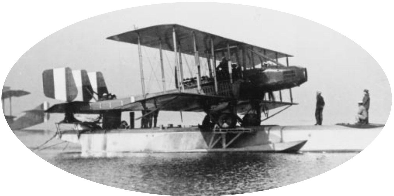
Sea sled, high speed boat for transport and launch of bombers, Caproni landplane on board, November 1918 229907
