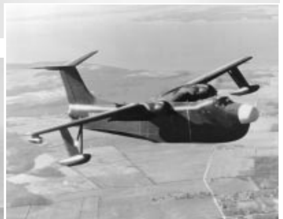
The P5M-2 Martin Marlin features a "T" tail 1053791
