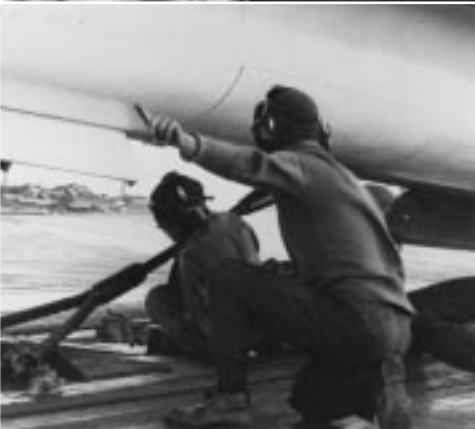
Old way, launching with catapult bridle 1110446
