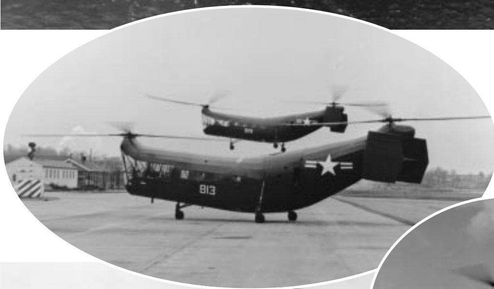
HRP-1, Tandem rotor transports of Marine Experimental Helicopter Squadron 1, take-off from Quantico 1053788
