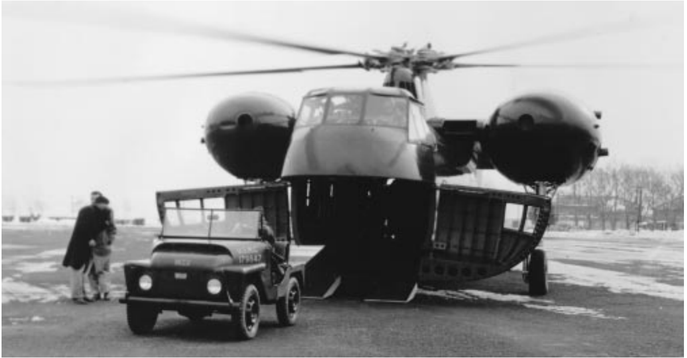
HR2S assault helicopter can lift three jeeps USMCA 150310
