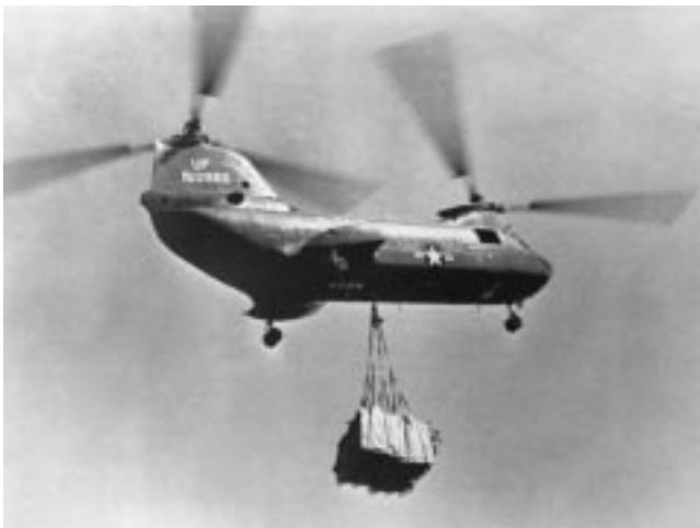
CH-46A during vertical replenishment NH 69969
