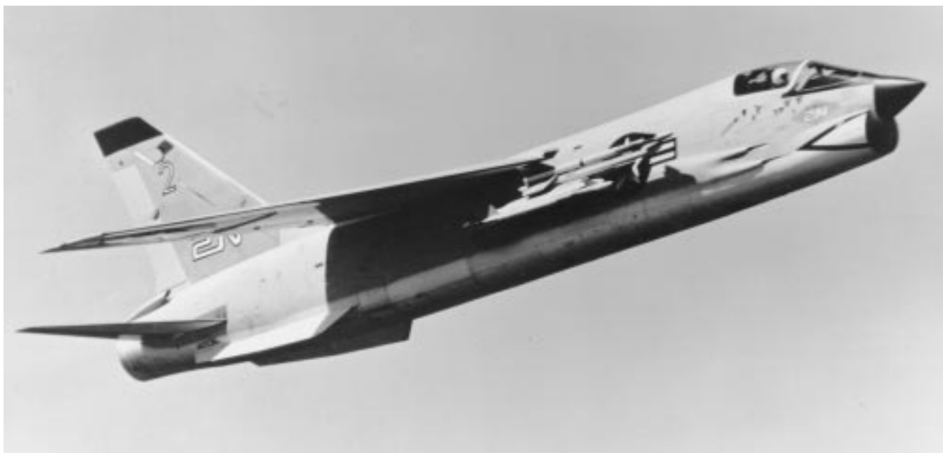
Vought F8U-2N Crusader, all-weather fighter is equipped with heat-seeking air-to-air missile Sidewinder 1061492
