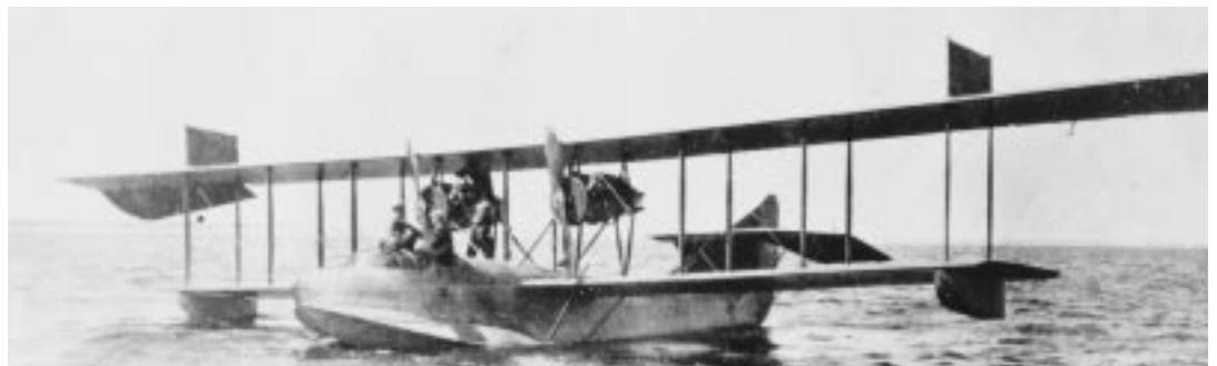
The Curtiss H-12, a twin engine flying boat, represented an early World War I step in aircraft development NH 60768
