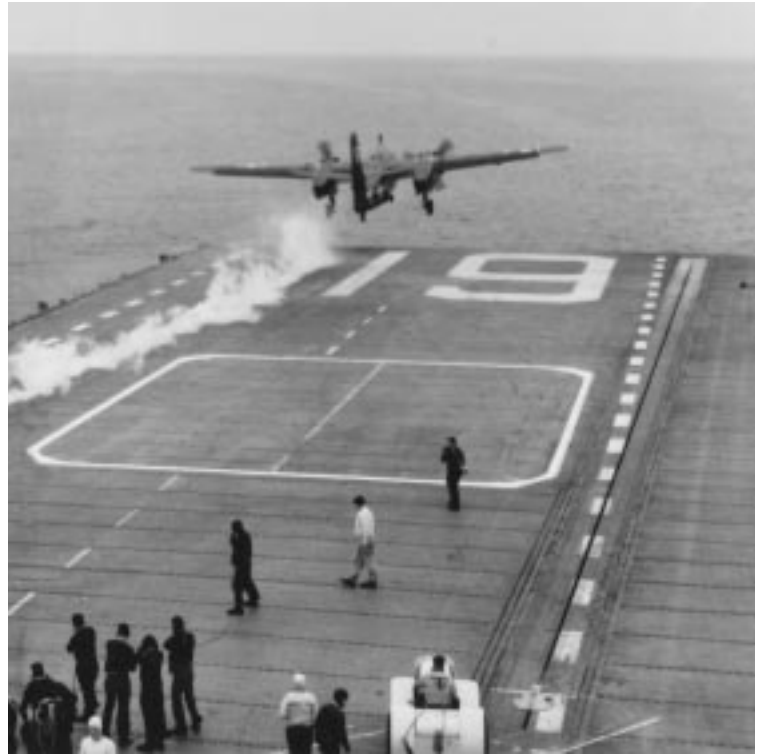
First operation of steam catapult, Hancock launches an S2F-1 638785
