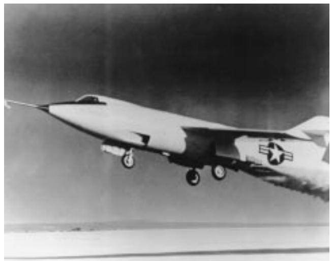
D-558-2, high speed research aircraft in which LtCol. Marion E. Carl made flights at 1,143 mph and 83,235 feet 651837
