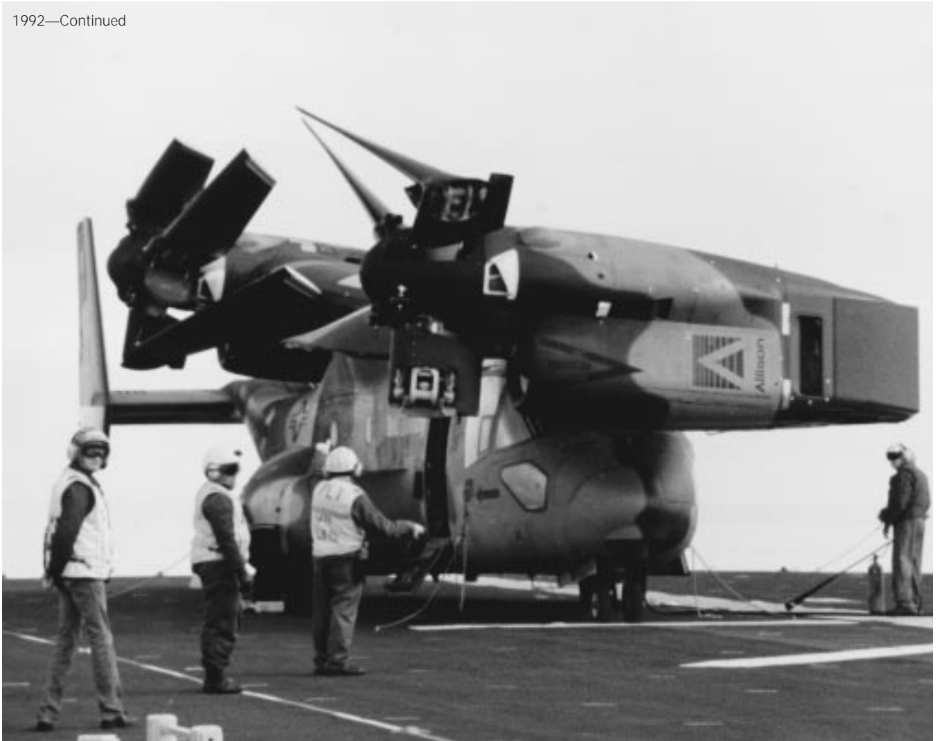
The complex wing and rotor folding arrangement of the MV-22A Osprey.
