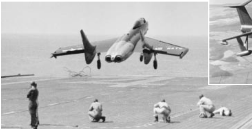
XF7U-1 Cutlass, Vought's tailless twin-jet fighter, taking off from Midway during carrier evaluation 432148
