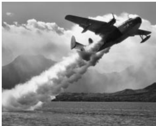
Launching a PBM Mariner, a dramatic demonstration of the utility of newly developed jet-assisted takeoff (JATO) 415346
