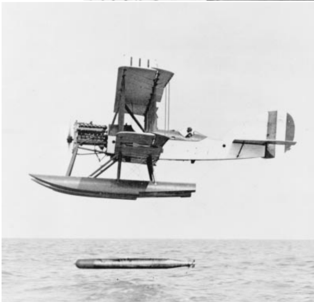
Launching torpedo from R-type aircraft, a means of increasing Naval avia- tion's offensive power 1061481
