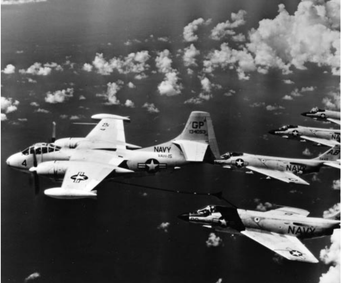
The F3H Demon being refueled in the foreground has double 00s on the nose of the aircraft. Aircraft with double 00s indicates they are assigned to an Air Group Commander (CAG). The other F3H Demons in the formation are from one of the fighter squadrons assigned to the Carrier Air Group. The refueling aircraft is an AJ tanker from VAH-15. NAH 000211
