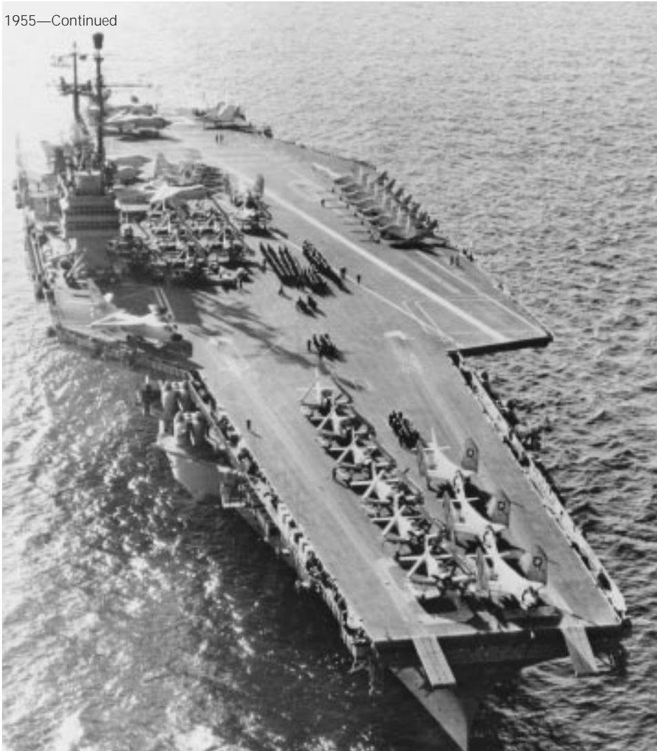
First carrier of a new class, Forrestal, was designed especially for operation of jet aircraft 709972
