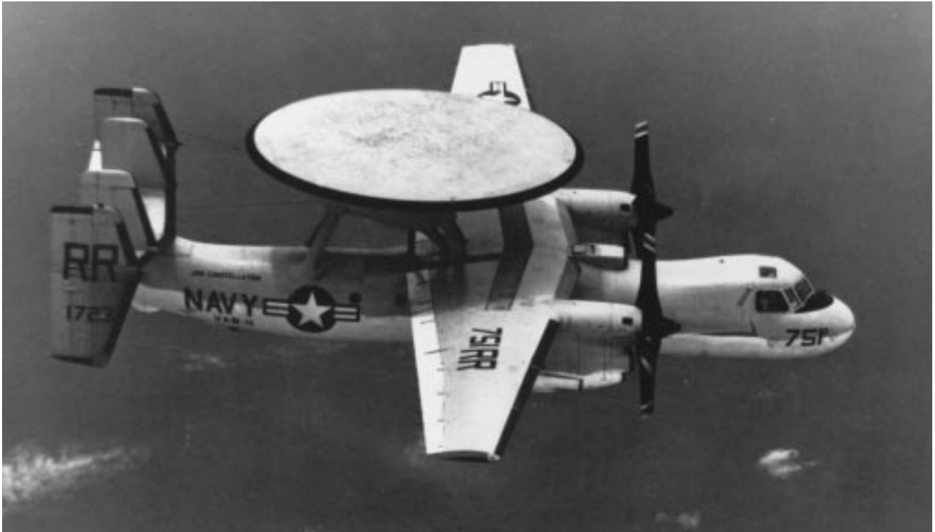
E-2A is used for early warning and to control tactical aircraft 1143451
