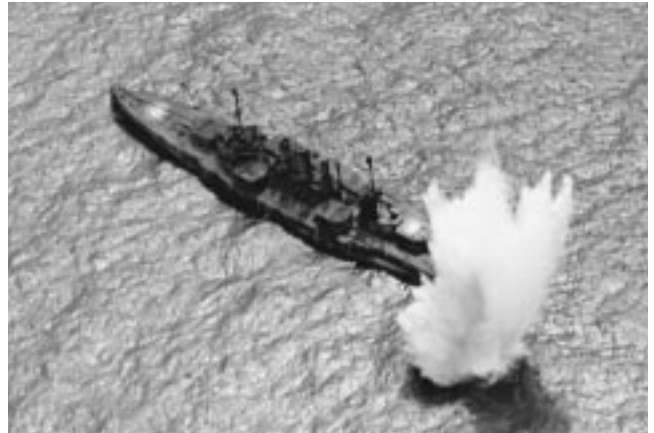
The Ostfriesland under attack in 1921 Army-Navy bombing test. Mining effects of hits like this sank her 161903
