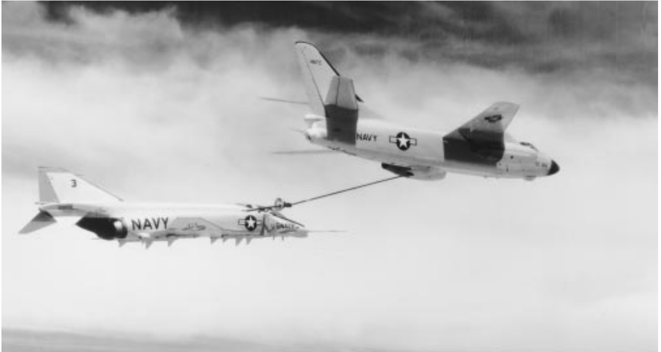
An A3D-2 aerial tanker, refuels an F4H-1 1042033
