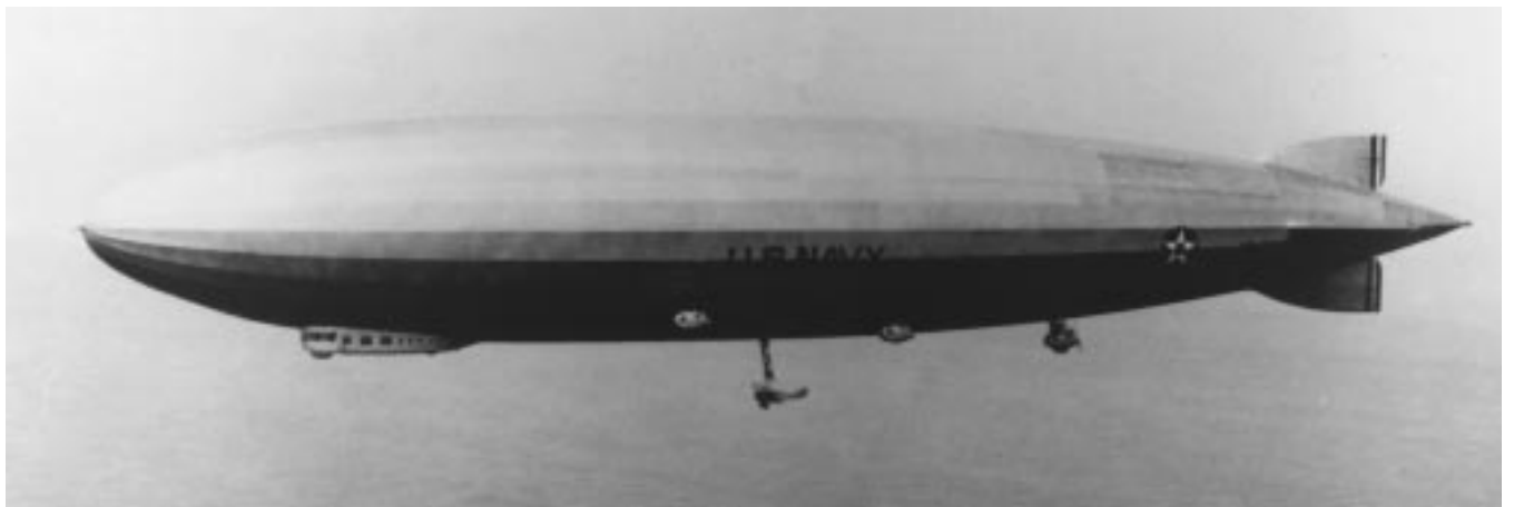
Lieutenant A. W. Gorton flying a Vought UO-1 makes hook-on landing on Los Angeles, a German-build rigid airship. 461642
