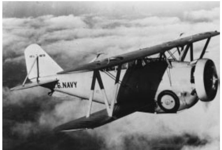
FF-1, first fighter with retractable landing gear 1061485
