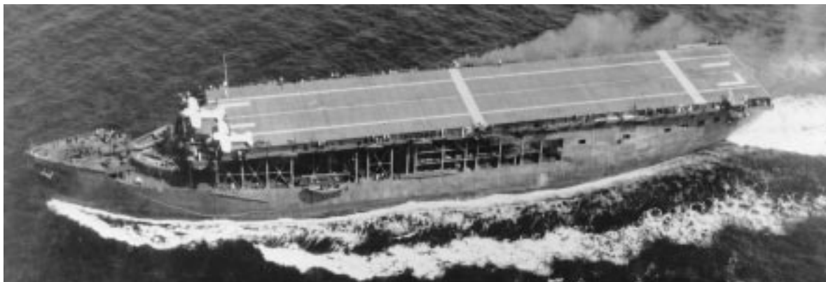
Long Island, first escort carrier of the U.S. Navy, was converted from the cargo ship Mormacmail 26567
