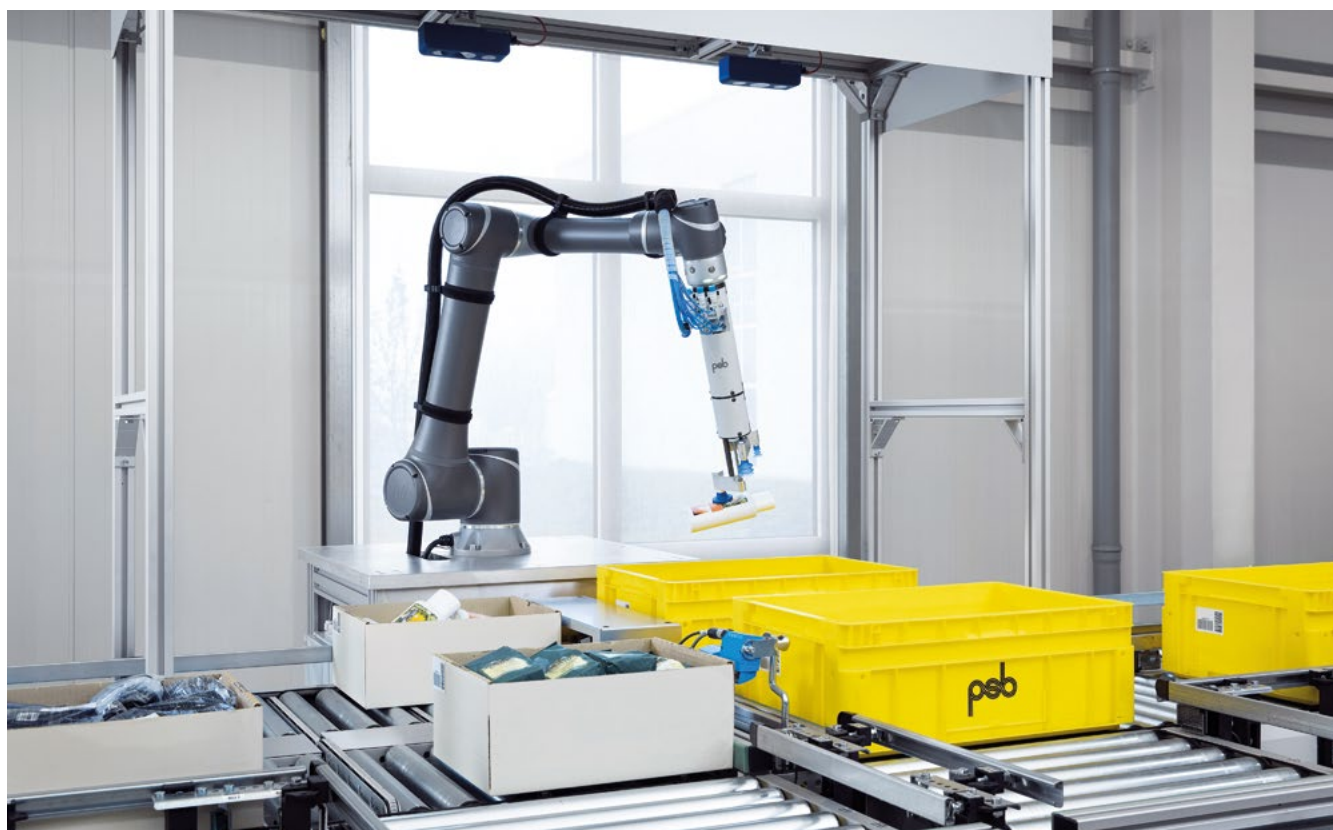
The robot picks up unknown products from bulk material and places them in the target container - 300-500 parts/h depending on the gripping object
