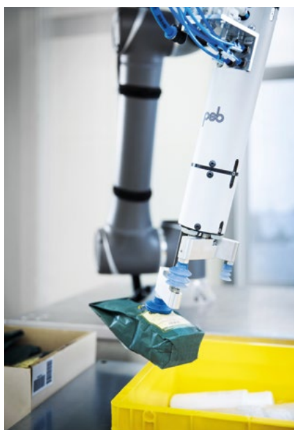
Multifunctional vacuum cups ensure gentle gripping of a wide variety of items
