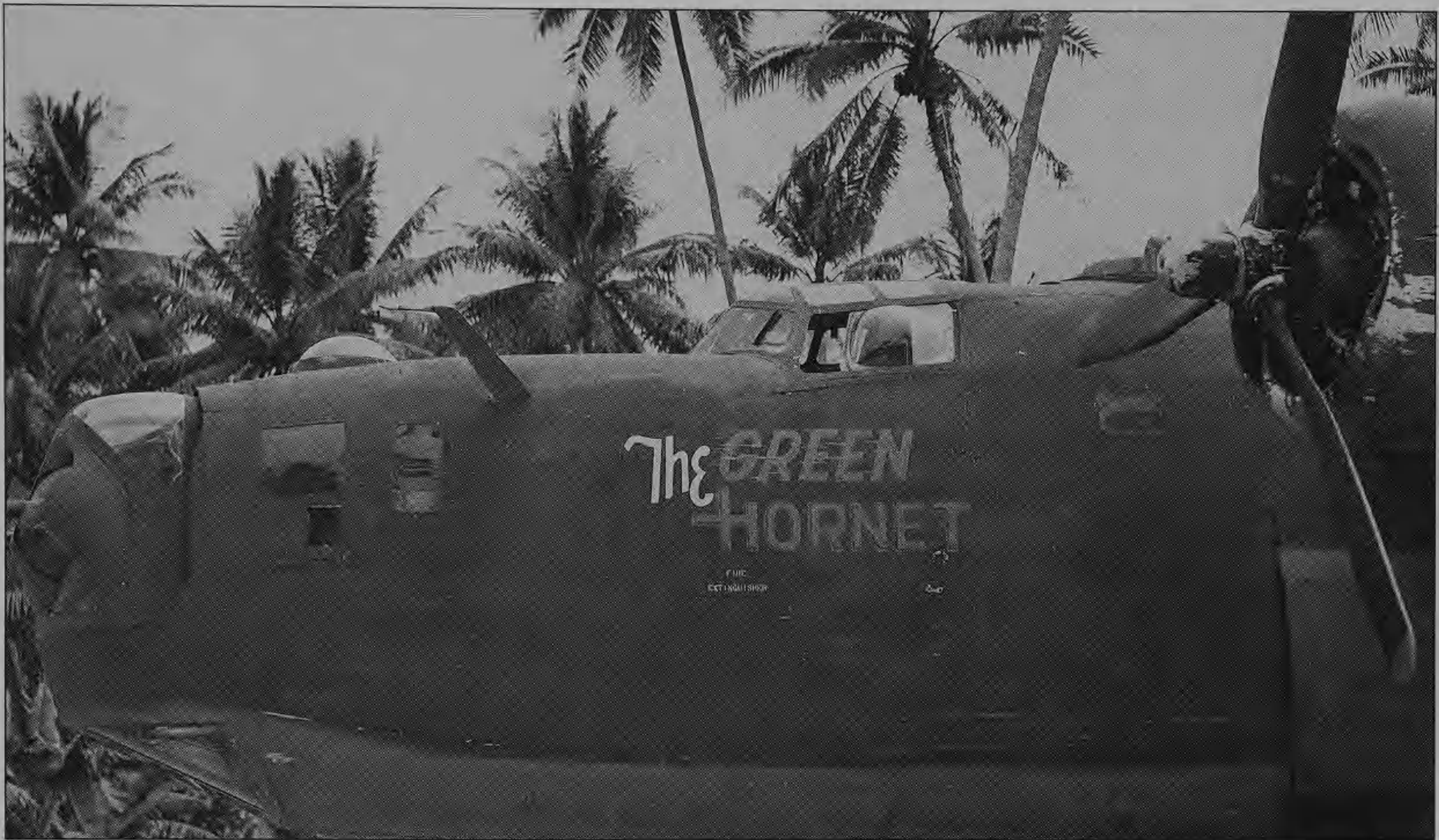
The installation of a Convair tail turret in the nose position was a standard measure on B-24D Liberators in the Pacific until the arrival of Liberators with production nose turrets. Here, the Convair turret has been installed in the nose of B-24D The Green Hornet of the 7th Bomb Group, 10th Air Force at Fanafuti Island, Ellis Group, in April 1943.
