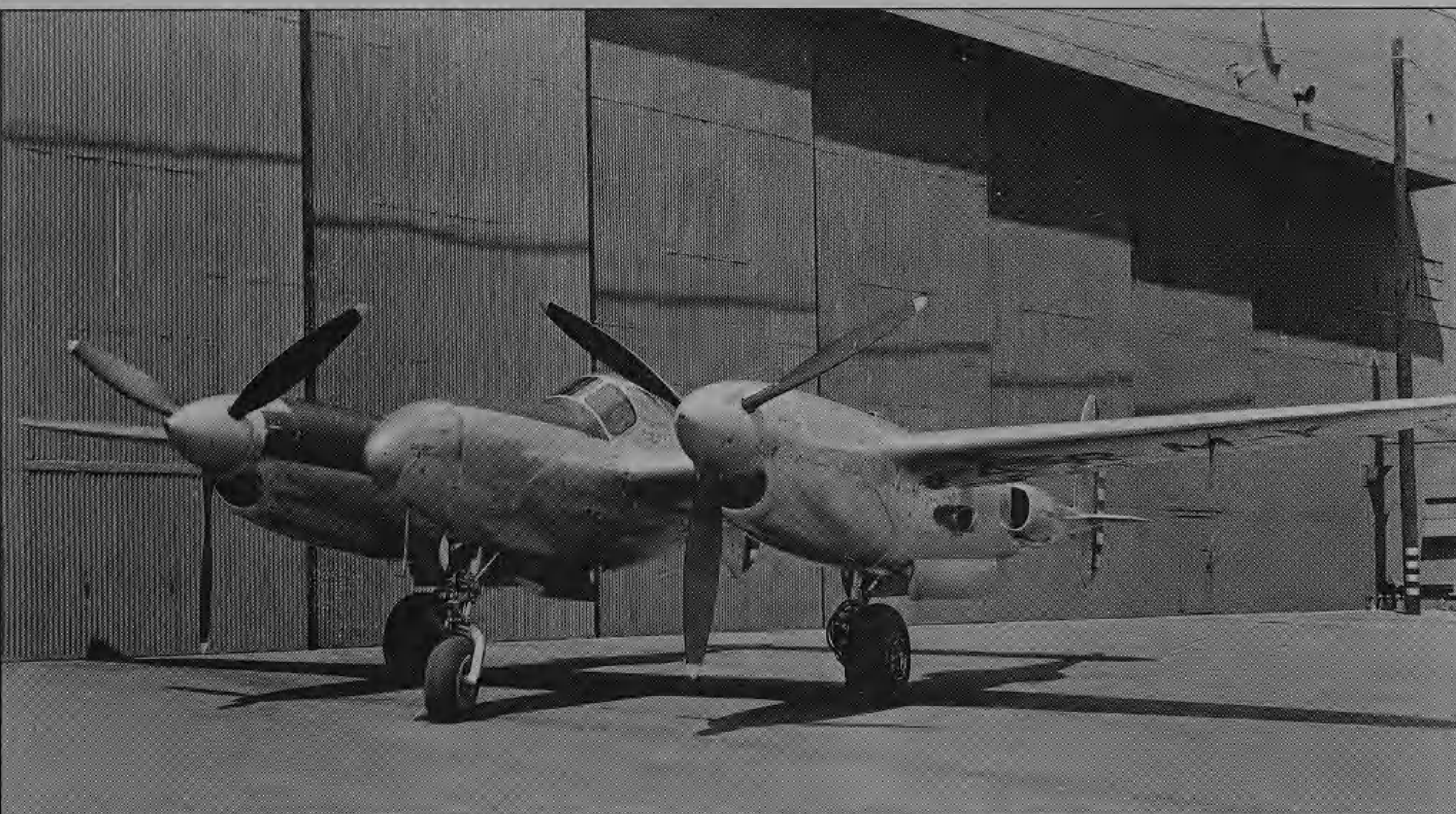
XP-49 40-762 stratospheric research aircraft regularly flew above 40,000 ft. This P-38 (Model 522) first flew in November 1942 and was used for high-altitude research and pressure-cabin development.
