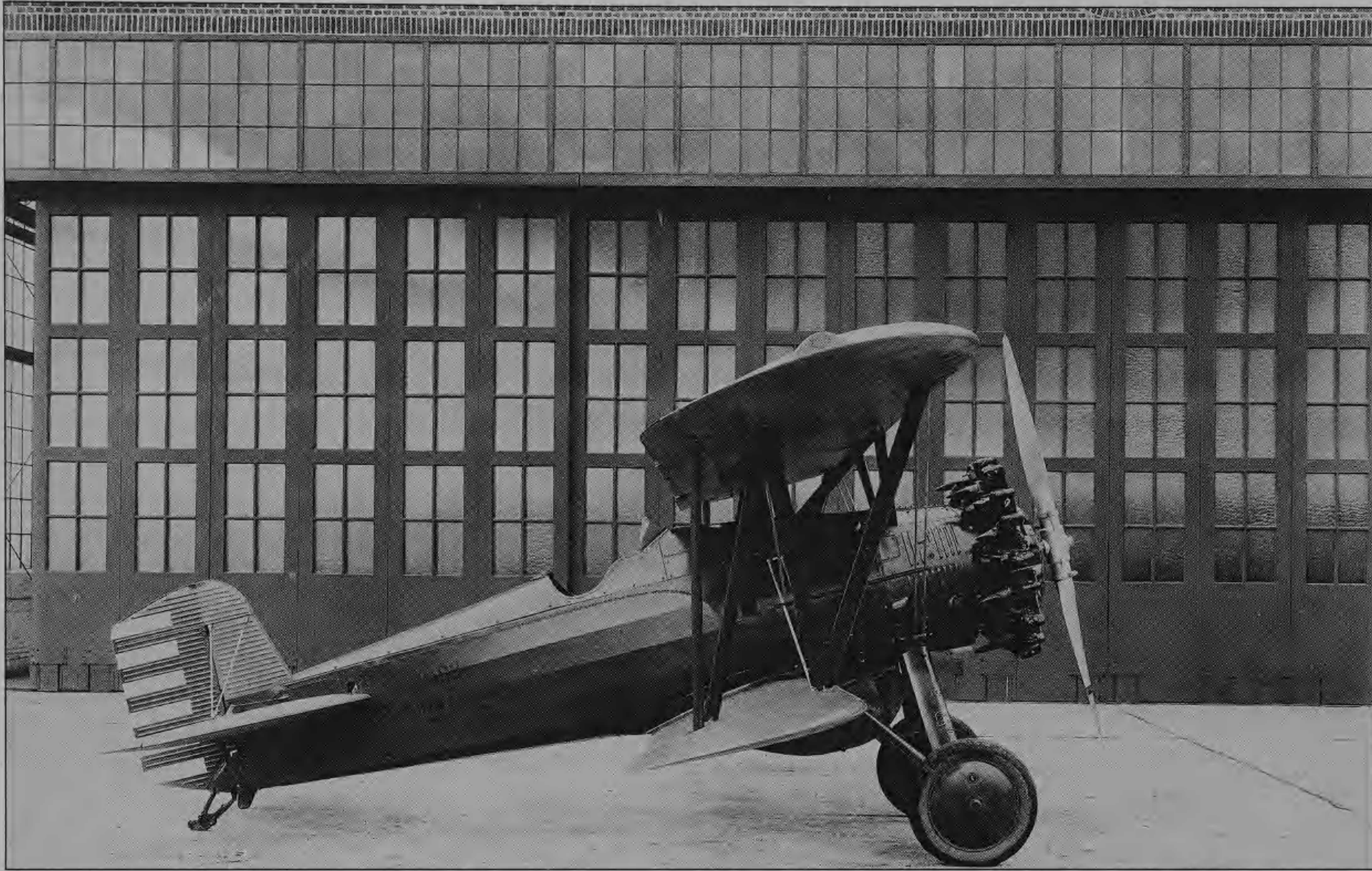
In 1929 ninety examples of the Model 102B (P-12B) (29-333 is seen here) were ordered, the largest single Army order for fighters since 1921. The optional 55-gallon auxiliary fuel tank is fitted under the belly.
