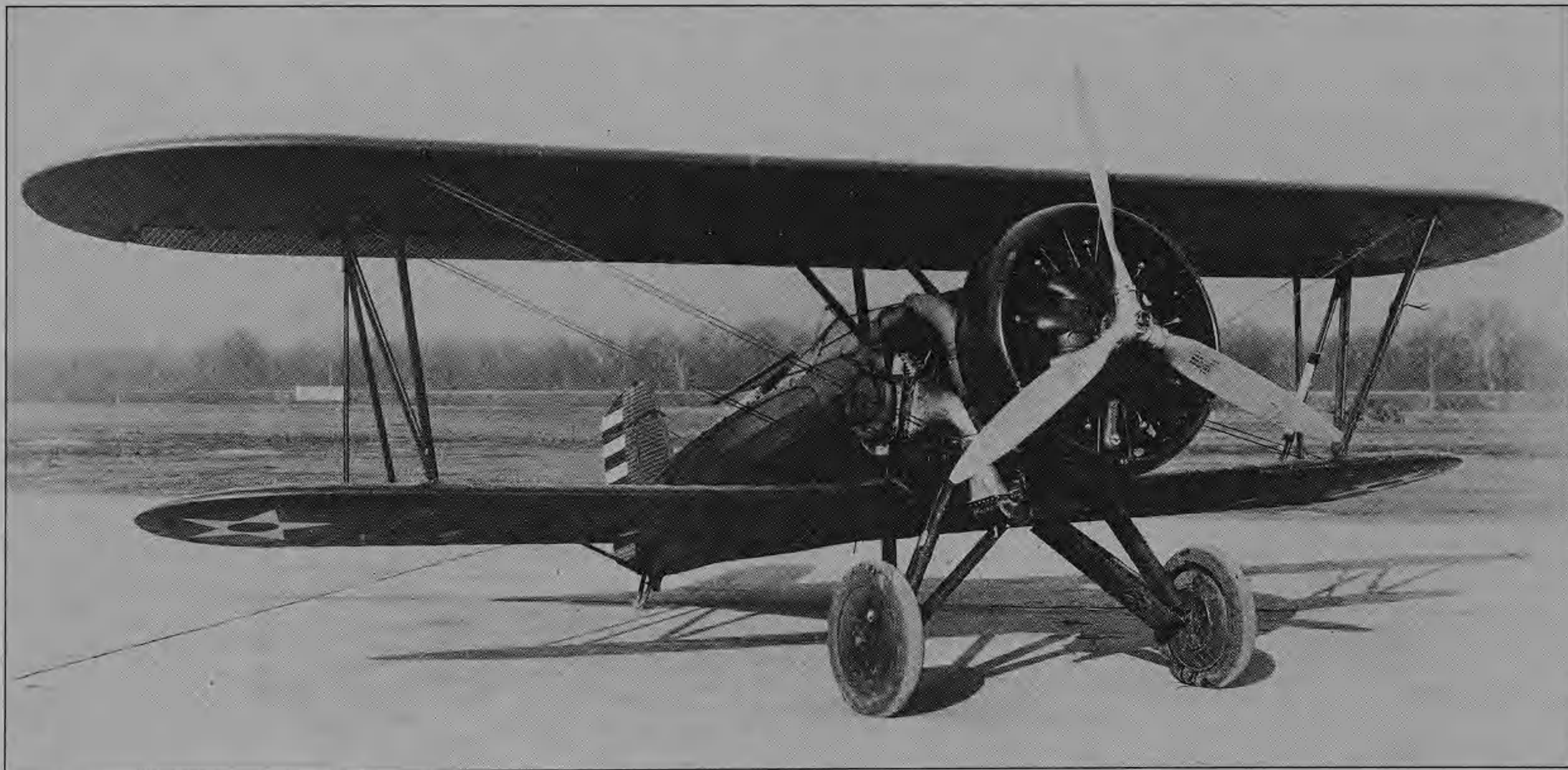
AAC 29-329, the first P-12B, was modified by the AAC as XP-12G to test turbo-superchargers and ring cowlings, and fitted with a three-bladed prop to absorb the additional power, before reverting to P-12B.
