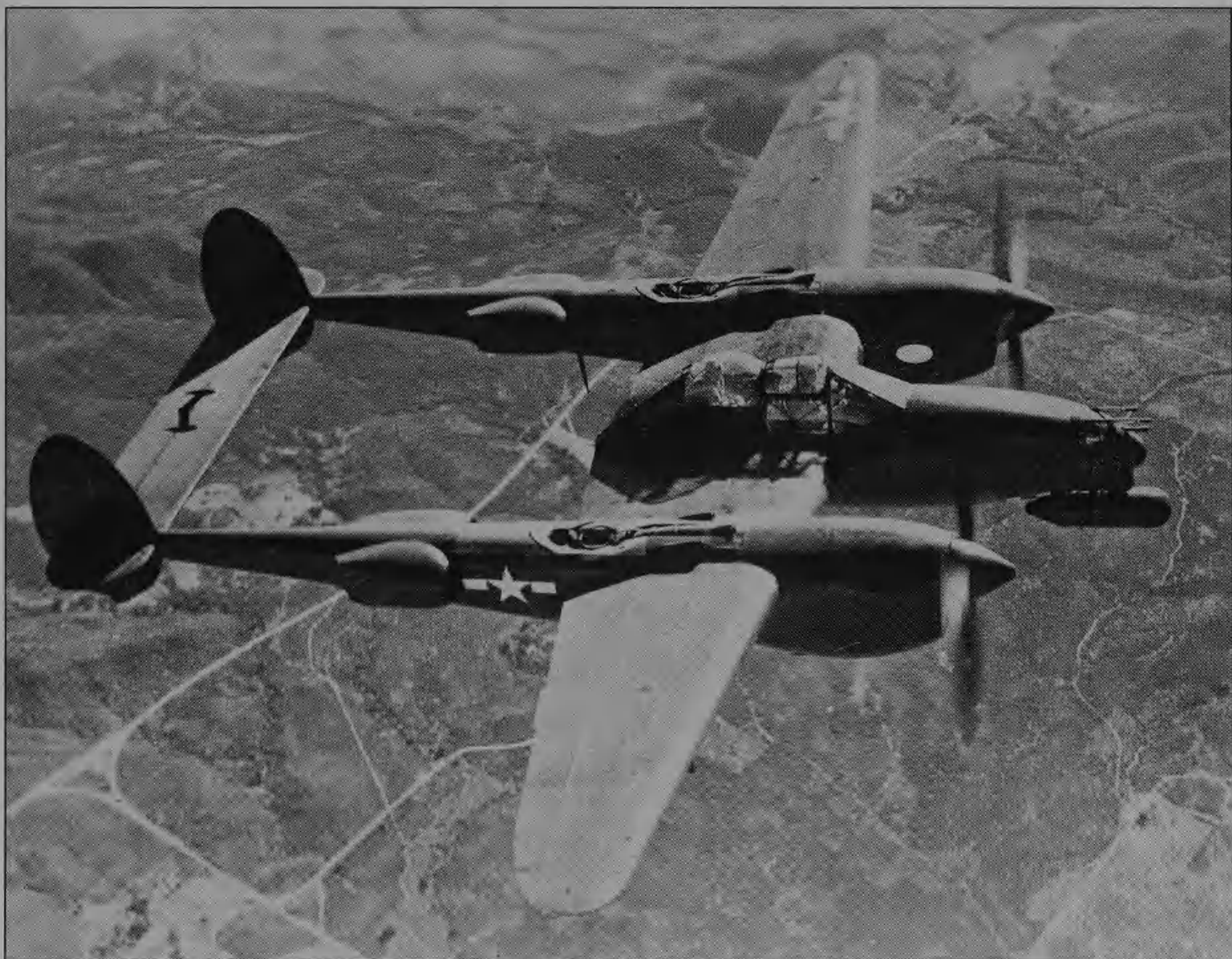
Another late arrival in the Pacific before the end of the war was the P-38M two-seat Night-Lightning (P-38M-5-LO 44-27234 is seen here), seventy-five of which were built from existing P-38L airframes. The P-38M was equipped with a SCR540 radar in a nose radome operated by an observer in a raised seat behind the pilot. In addition to the two 20-mm cannon and four .50-in machine-gun armament retained from the P-38L, the Night-Lightning also had launching racks for HVAR rockets beneath the wing.
