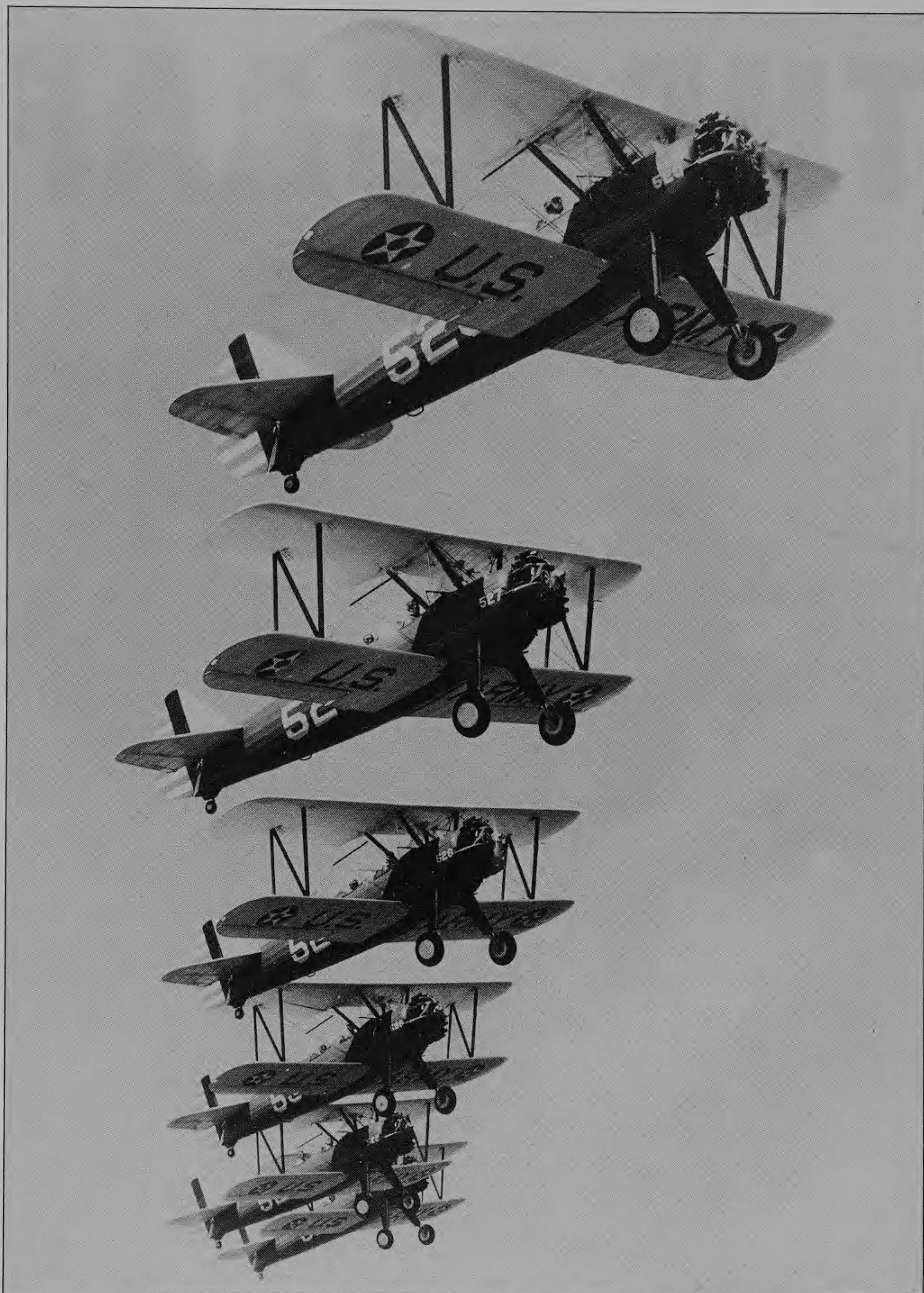
Training for war – magnificent flight of Model 75 PT-13 Stearmans, 1936. The PT-13 was the first in a long line of primary 'Kaydet' trainers, the Army placing its first Stearman order for twenty-six PT-13s in July 1935. The production PT-13 flew for the first time in April 1936, and deliveries were made between June and December 1936. Stearman operated from Wichita, Kansas, until 1 April 1938 when Boeing Aircraft acquired the company and created its Stearman Aircraft Division.
