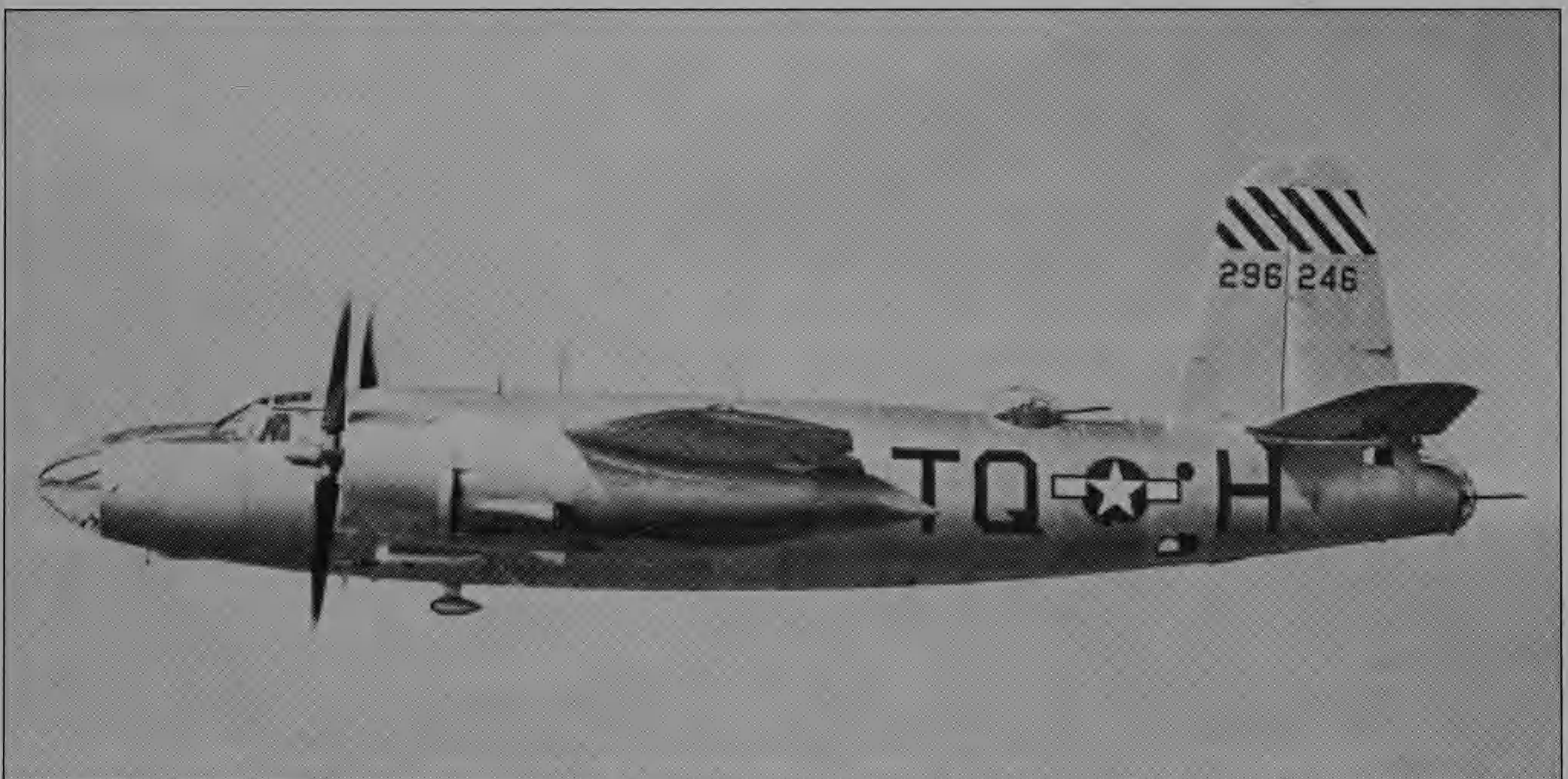
Martin B-26F-1-MA 42-96246 TQ-H of the 559th Bomb Squadron, 387th Bomb Group (Medium), 8th Air Force, which transferred to the 9th Air Force in October 1943. The B-26F had the wing incidence angle increased slightly in an effort to further improve take-off performance. Some 300 Fs were built, of which 200 went to the RAF and SAAF, before minor internal changes altered the designation to B-26G. Some 893 Gs were built before deliveries ceased in March 1945. Altogether, 5,266 Marauders were built, of which 1,585 were built in Omaha, Nebraska, and 3,681 in Baltimore.
