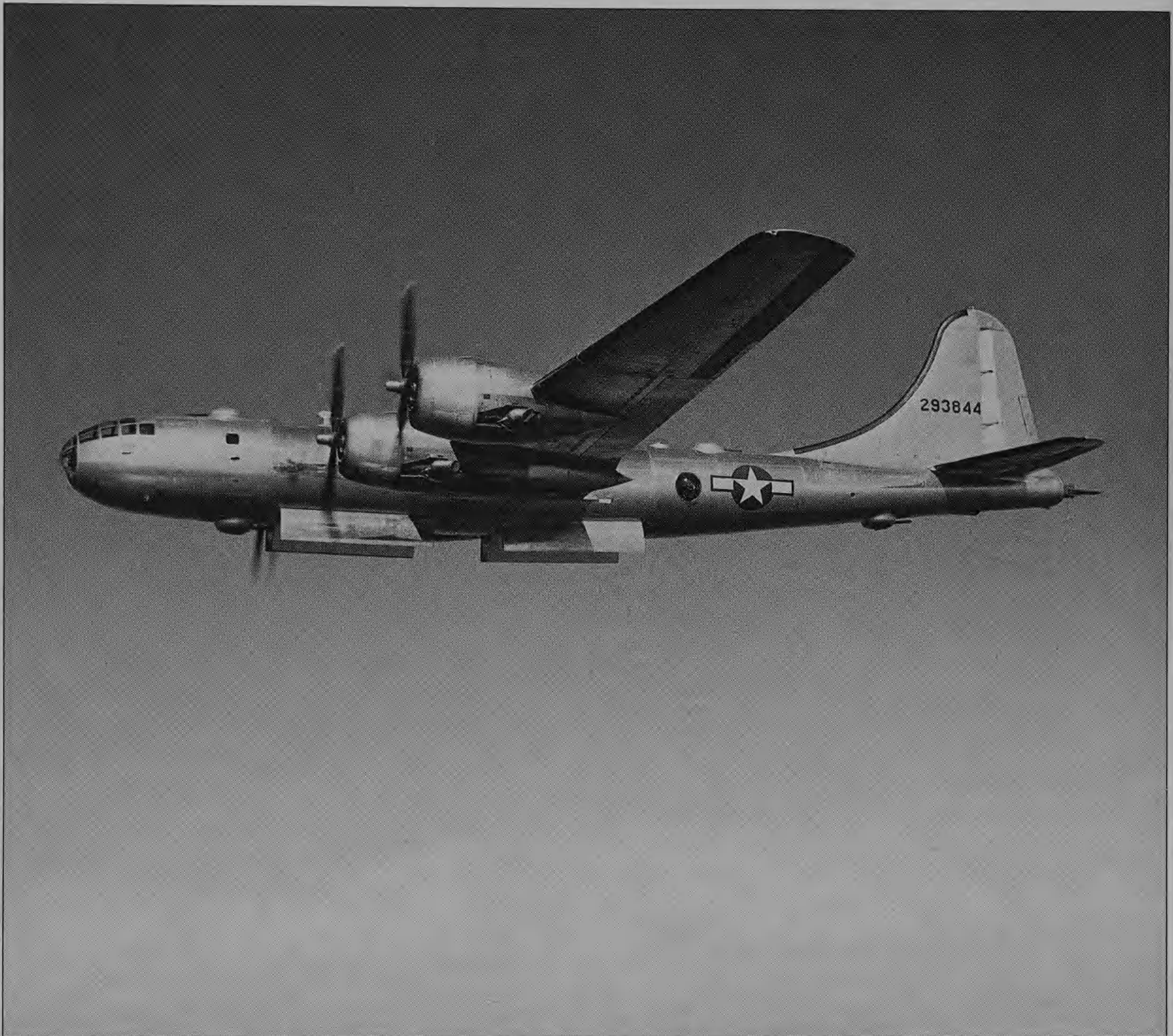
B-29A-BN 42-93844, with both sets of bomb-bay doors open, 1944. Renton-built articles differed only in having four guns instead of two in the front turret.
