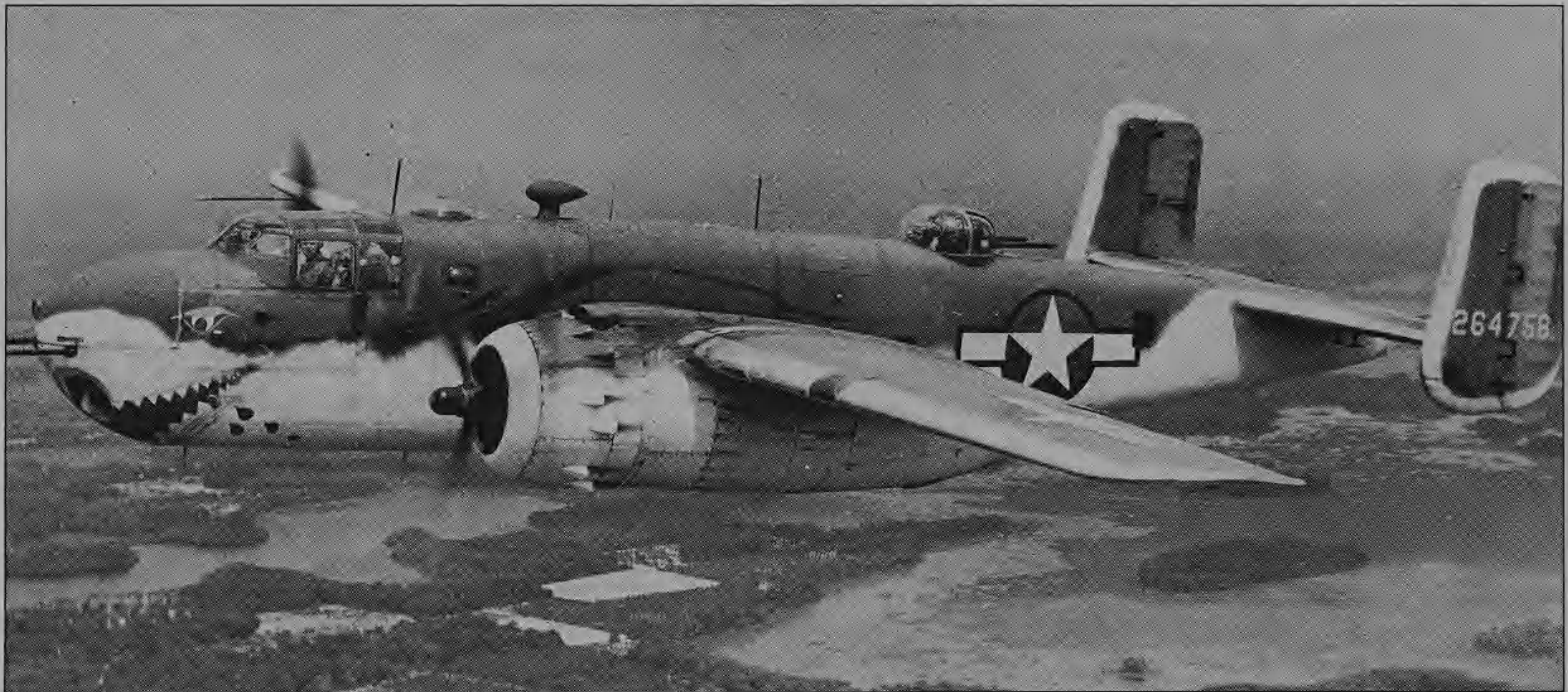
B-25C-25-NA 42-64758 in early USAAF maritime scheme, one of a hundred built that completed production of the C model at Inglewood, California, in May 1943. It has been retrofitted with a 75-mm M-4 cannon in the lower left side of the forward fuselage below the two fixed .50-calibre nose guns. This cannon was tested in the XB-25G on 22 October 1942 and five B-25C-15s were completed as B-25G-1s, the first flying on 16 March 1943. The M-4 was hand-loaded with twenty-one rounds from the loading tray behind the pilot. The last of 400 B-25C-25s completed as B-25Gs were finished by August 1943.
