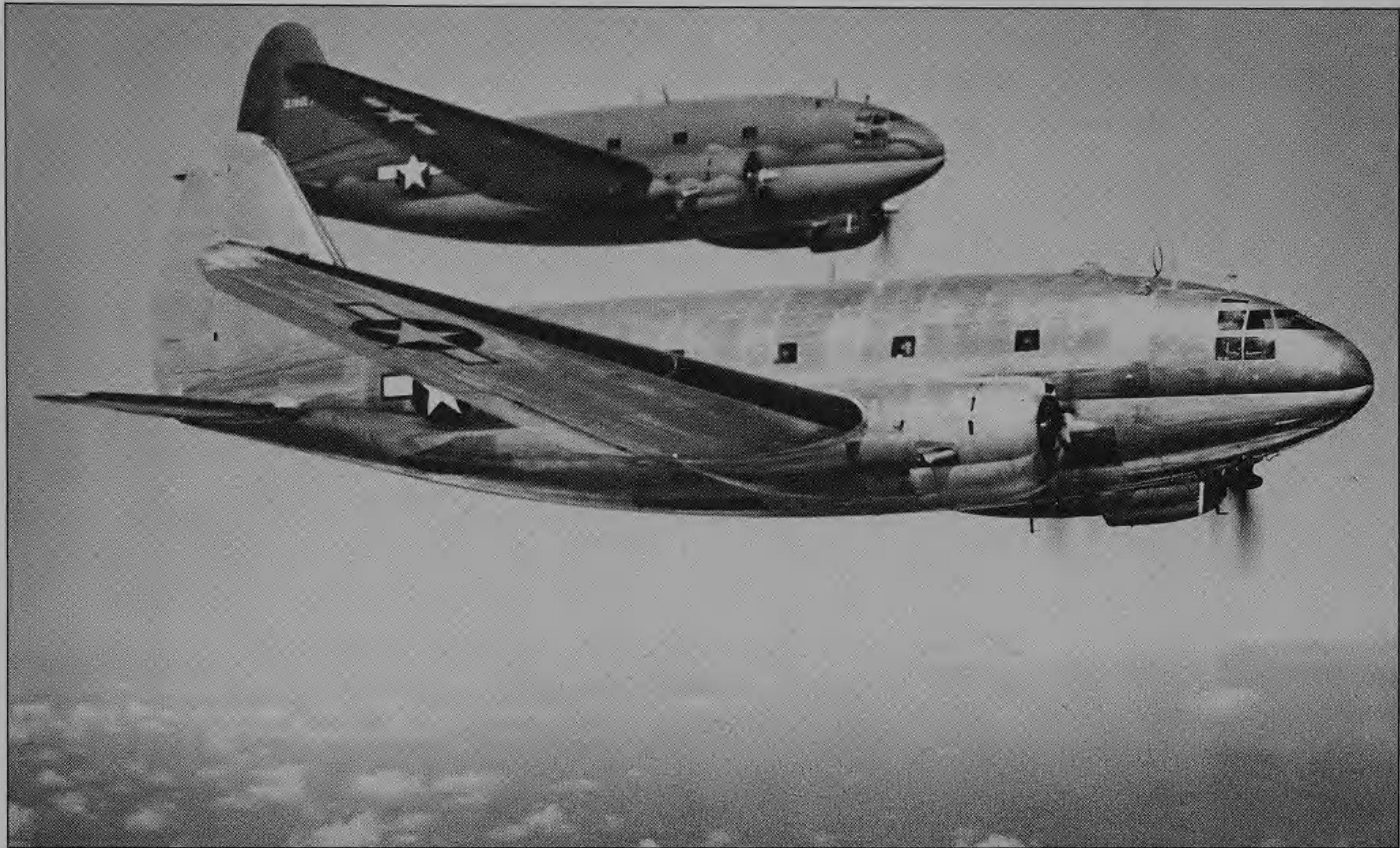
Curtiss C-46A Commandos in formation, 1944. The design originated in 1937 as a 36-seat commercial transport, but in the Second World War the C-46 was widely used as a troop and freight carrier for the AAFs. The Commando operated primarily in the Pacific theatre because of its greater load-carrying capability and better performance at high altitude than the C-47. Its most famous theatre of operations was the supply of war material to China from India over the 'Hump'. Altogether, 1,491 C-46s were built and many remained in service after the war.
