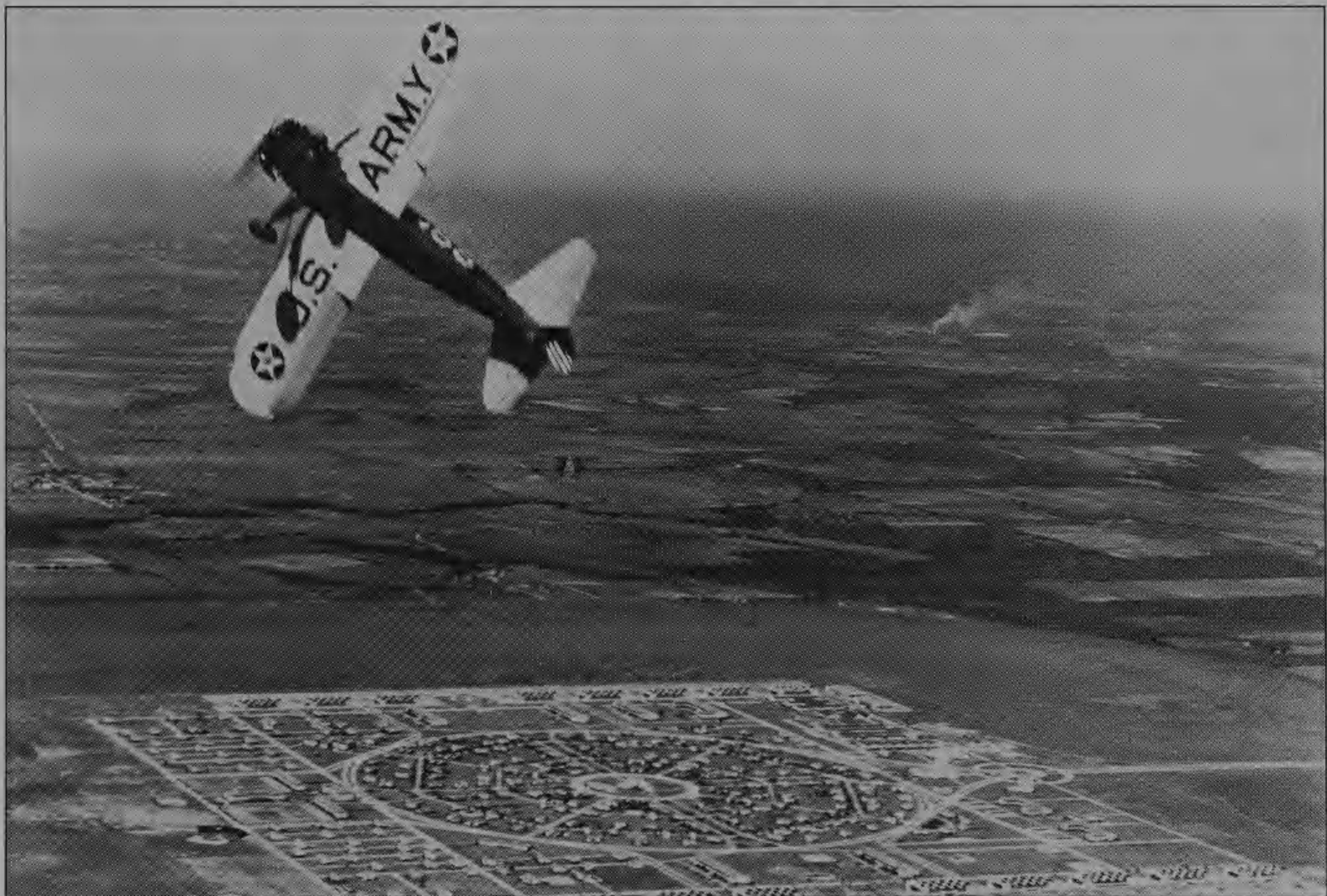
PT-13A aerobating over Randolph Field, 15 January 1938. Three separate orders for ninety-two A75 (PT-13A) aircraft fitted with 220hp Lycoming R-680-7 radials, improved instrumentation, landing light, blind-flying hoods and electrical systems were ordered for Army service and these were delivered between April 1937 and June 1938. Altogether, 3,769 A75N1s would be built, including 2,942 for the AAC. The first Stearman came off the production line at Wichita in February 1945. All told, some 8,585 Model 70/76 Stearmans were built between 1933 and 1945.
