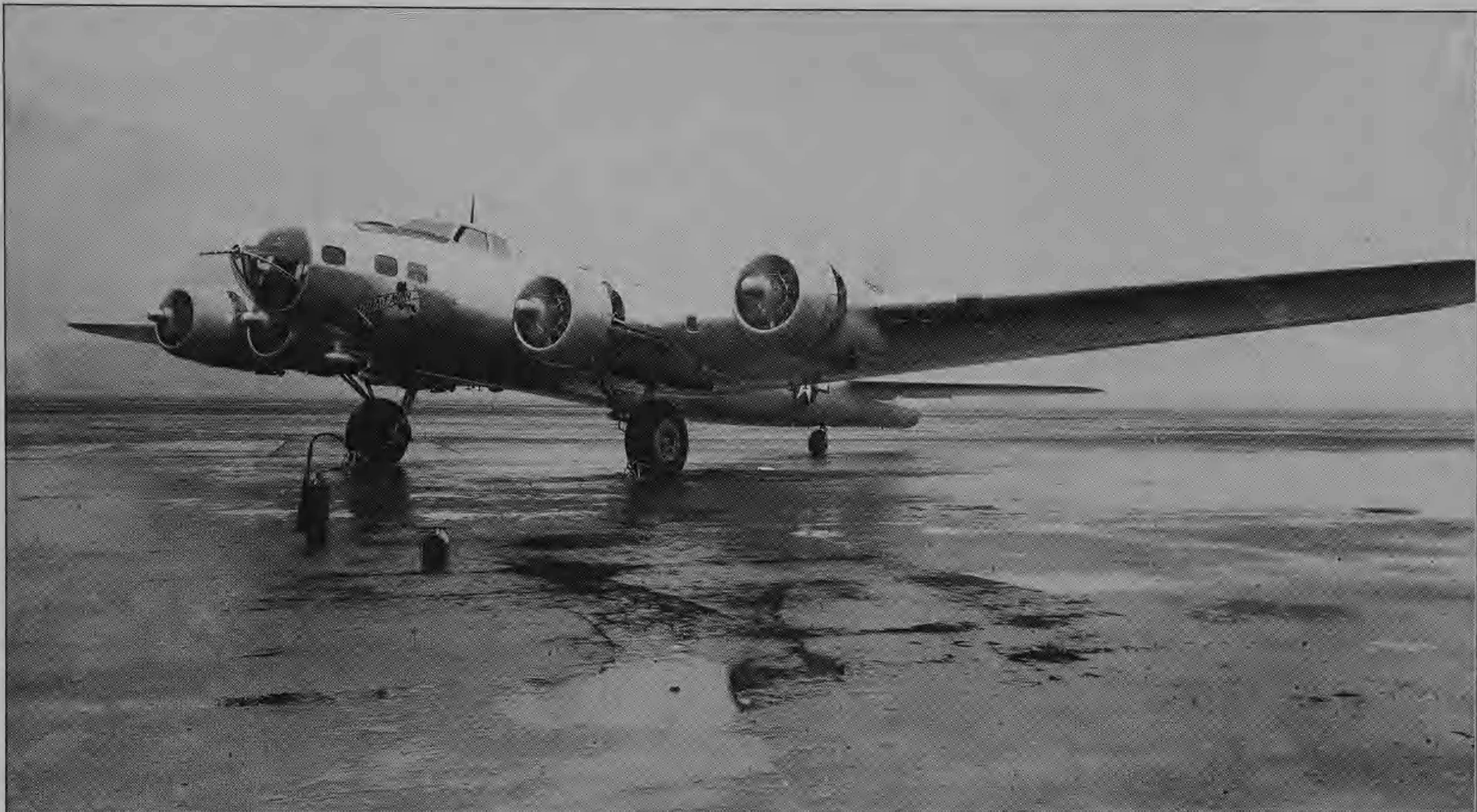
General Douglas MacArthur's B-17E-BO (XC-108) 41-2593 Bataan , 29 November 1943. It was one of four B-17E and Fs specially converted into transports under the C-108 designation in 1943. Although an E, Bataan had a 'blown' B-17F style Plexiglas nose with a single .50-calibre gun with chromed barrel (the only armament carried) and a navigator's astrodome added to the aircraft. A five-man crew and up to eleven passengers could be carried on the XC-108.
