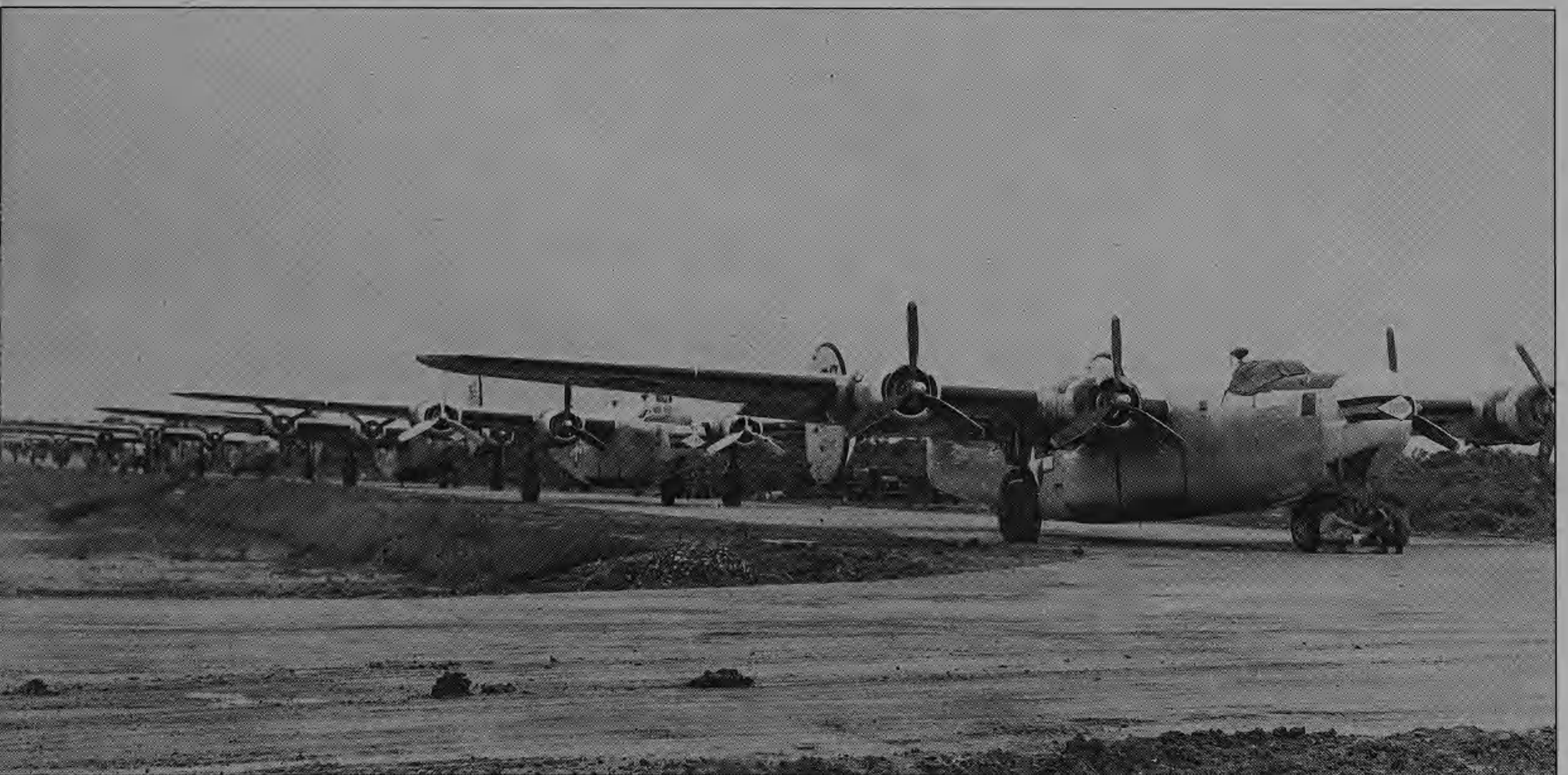
A fleet of C-109 'Flying tankers' operated by Air Transport Command in India, used to support B-29 operations in the CBI, 1944. All C-109s were conversions of B-24J and L models with the turrets deleted, and were fitted with seven specially designed fuel tanks in the bomb bay, and one more in the nose, to give a fuel-carrying capacity of 2,900 US gallons.
