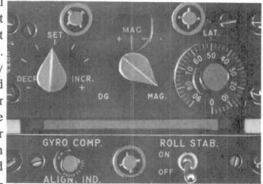
Figure 1-12 Compass Indicator Control Panel
