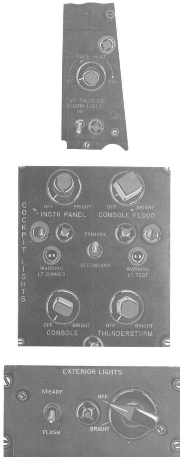
Figure 1-11 Lighting Panel Front Cockpit
