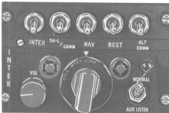
Figure 1-15 Intercom Control Panel
