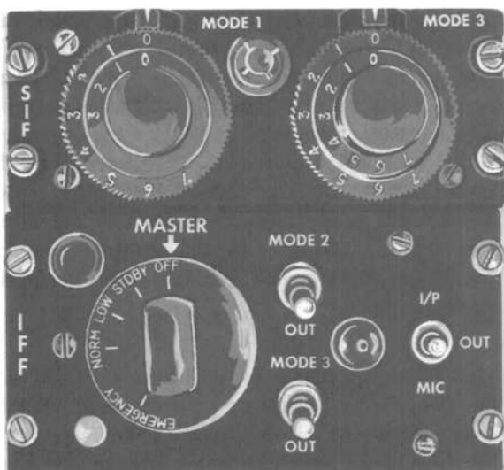
Figure 1-13 IFF/SIF Control Panel
