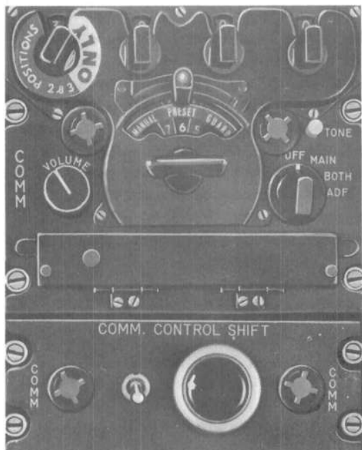
Figure 1-16 UHF Control Panel
