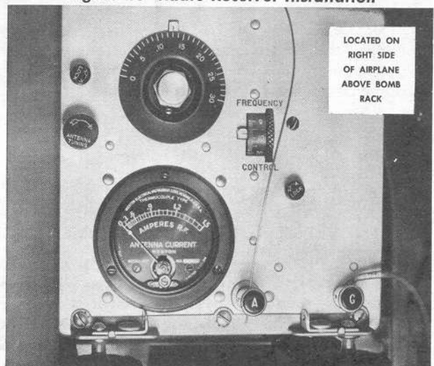
Figure 49—Radio Transmitter Installation
