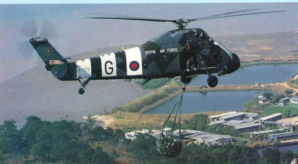
The Wessex can carry useful loads underslung on a hook, in this instance food and ammunition. Photographs Sue J. Bushell unless otherwise credited.
