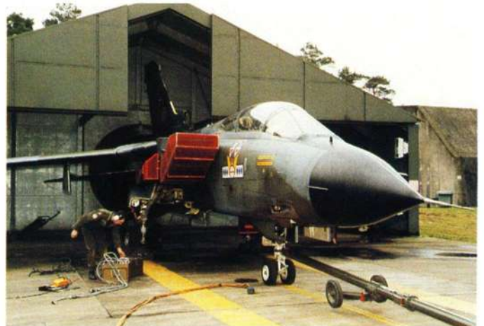
After engine testing, the GTB is disconnected but the intake safety guards remain in position.
