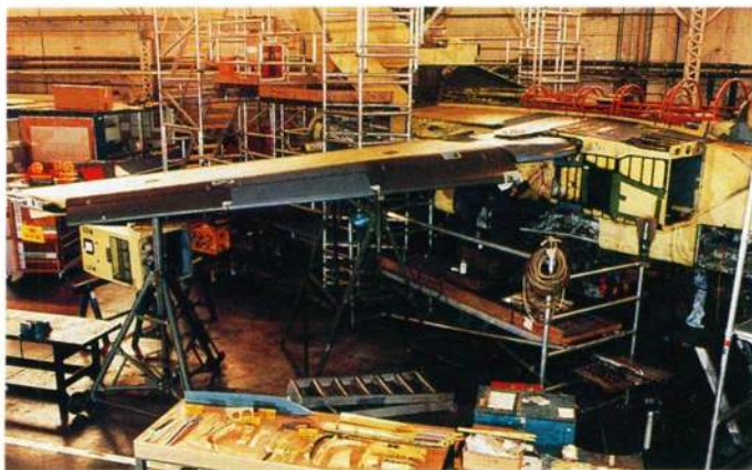
The combined Major and 5FI service underway, showing 'before' and 'after' side panels during the 5FI element. RAF St. Athan
