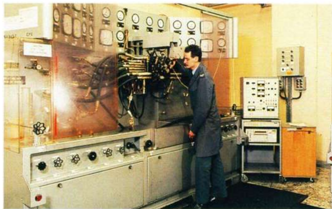
Tornado high-lift wing sweep control unit is set up for testing by No 9 Squadron. RAF St. Athan
