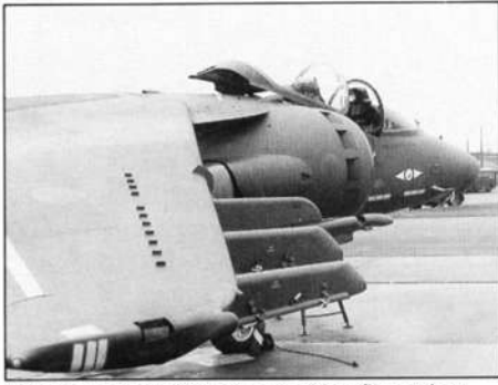
This view shows the large carbon-fibre wing and armament pylons. Paul Jackson
