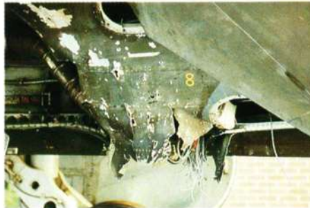
Above top: A major problem facing personnel engaged in Battle Damage Repair work is the lack of modern aircraft on which to practise techniques. This Canberra rear fuselage section is being used as a suitable subject for panel and rib repair. Photographs Sue J. Bushell.
