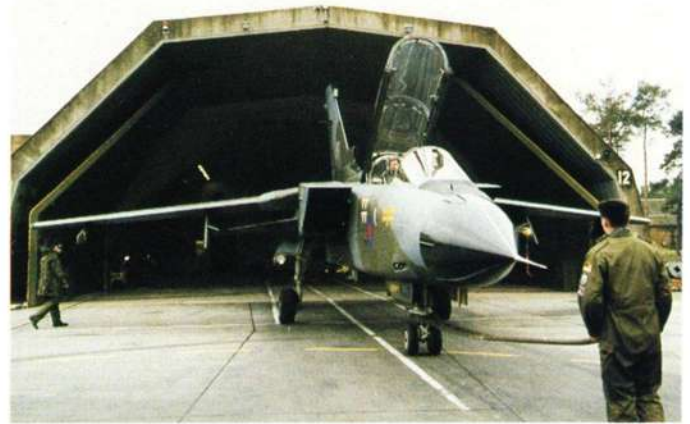
After engine testing, the GTB is disconnected but the intake safety guards remain in position.
