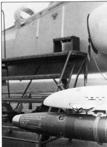
The head of an inert practice missile which gives all the indications of a missile firing without actually leaving the aircraft. The missile fins are removed during normal training.
