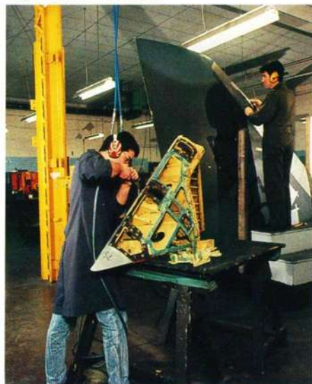
In the Structures Bay, No 7 Squadron personnel work on a Tornado wing nib and taileron leading edge repair. RAF St. Athan
