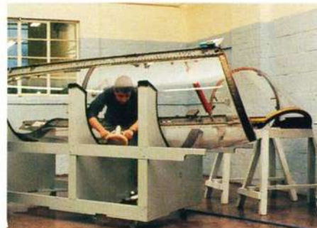
In the Structures Bay, No 7 Squadron personnel work on a Tornado wing nib and taileron leading edge repair. RAF St. Athan
