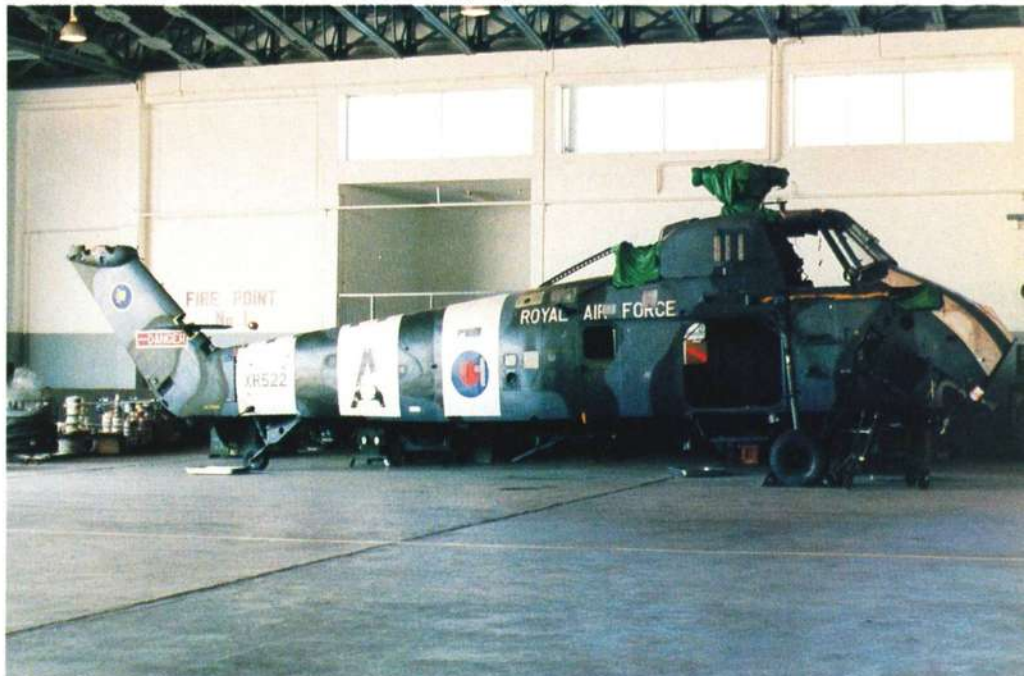
At any one time, a Wessex will be in pieces undergoing deep maintenance.
