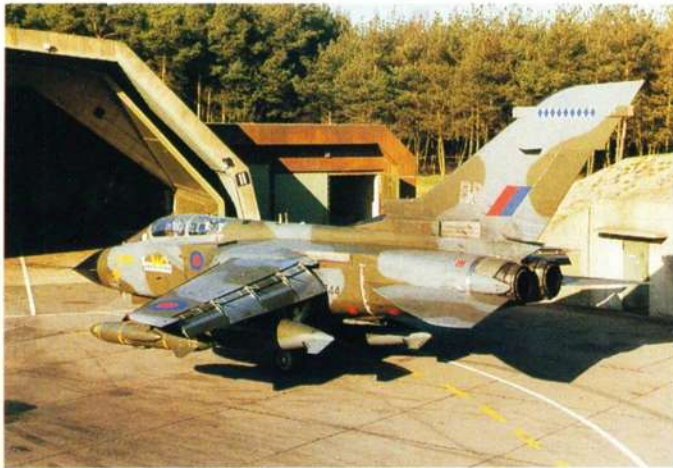
There is little room to spare with a Tornado in the HAS. A drop-tank rack occupies the right hand corner.
