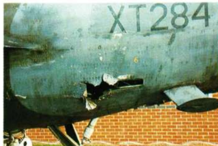
Shell damage to a Buccaneer undercarriage bay. This damage was inflicted at RAF Abingdon to provide a realistic repair scenario. Fragments of the shell travel a long way inside the aircraft, and all damage will have to be made good.
