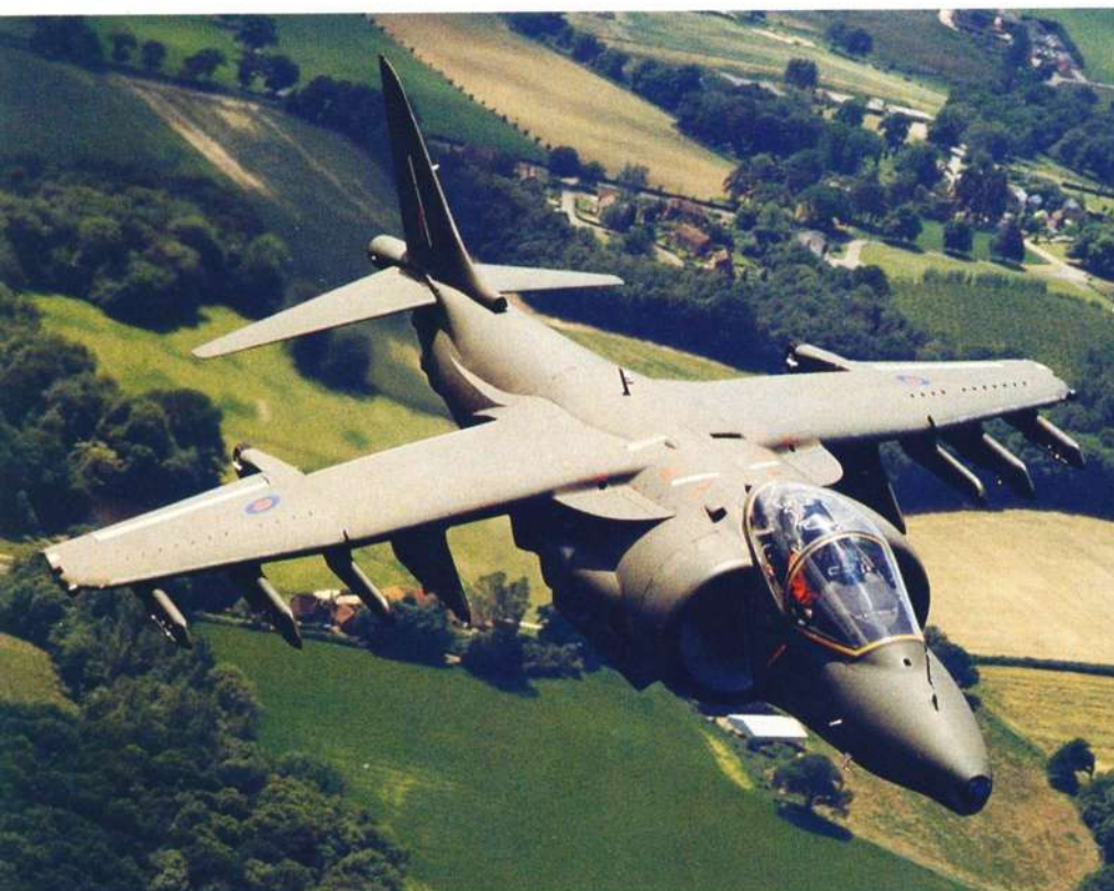
Above: The higher-perched cockpit is one of the key recognition features of the Harrier GR5 – it also has four extra weapons pylons, leading edge root extensions and re-positioned outrigger wheels. BAe
