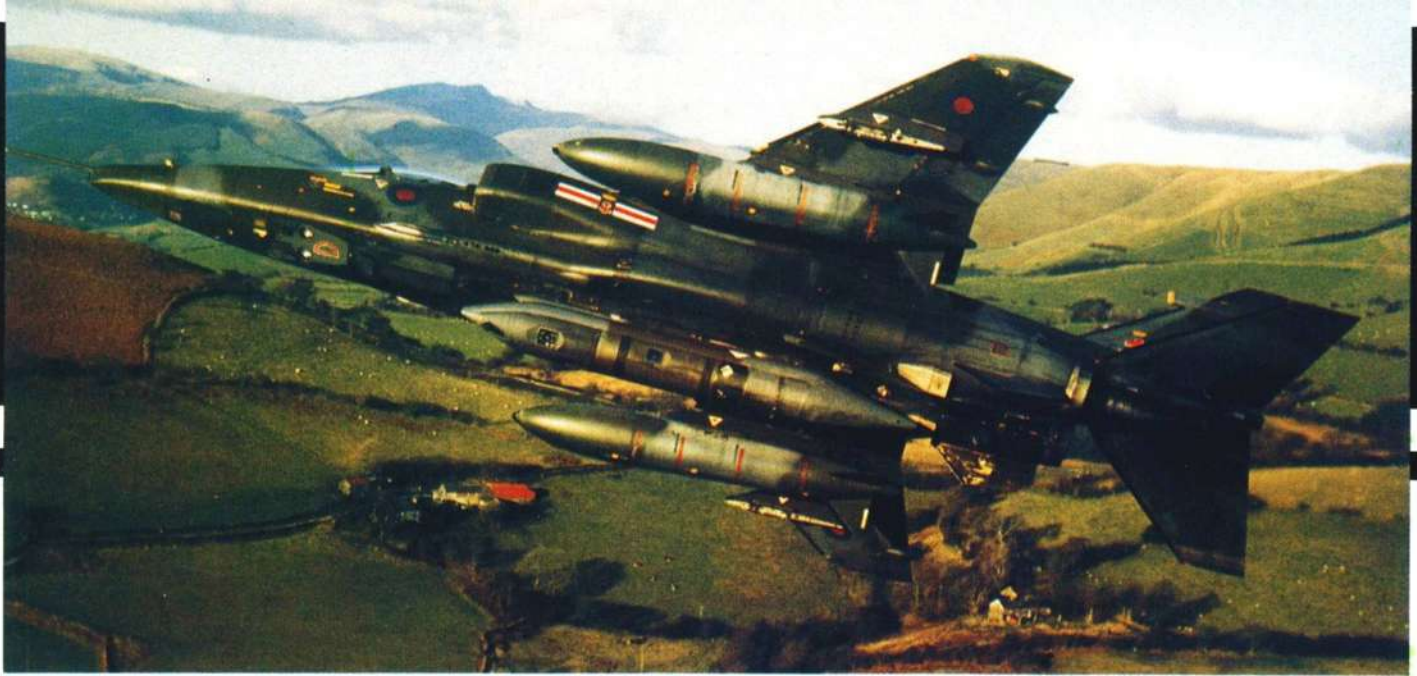
The camera pod is clearly visible as the Jaguar banks away. Three camera ports may be seen, as can the IRLS sensor, towards the rear of the pod. The silvery object directly ahead of the port ventral fin is an AN/ALE-40 chaff/flare dispenser. Lindsay Peacock
