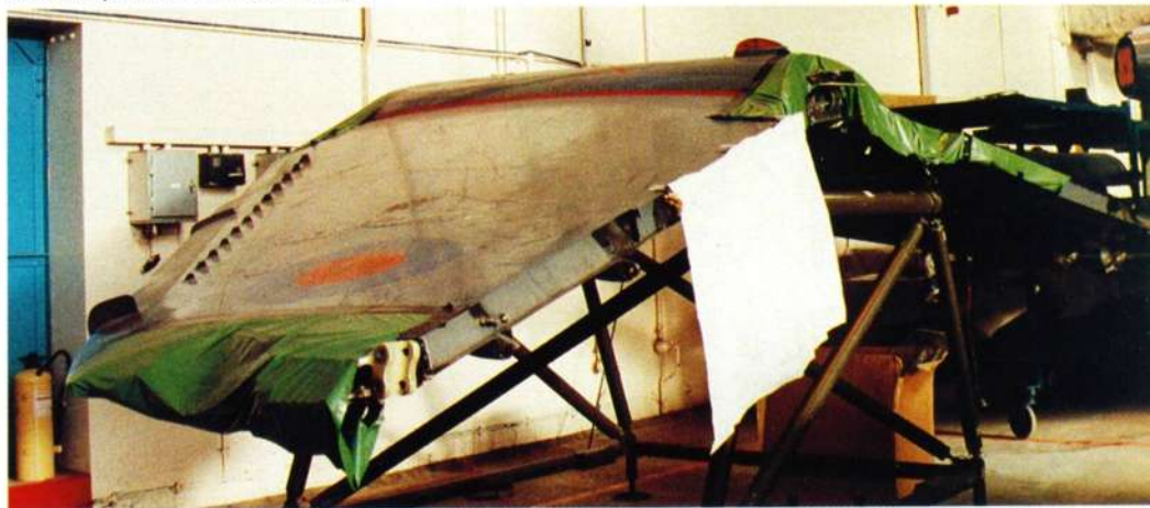
Below: Another repair being undertaken at Abingdon, this time on a Sea Harrier wing section. The RSS is responsible for all fixed-wing service aircraft repairs throughout the world, with the sole exception of mainland Europe.
