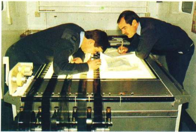
With the aid of a light table, Reconnaissance Intelligence Centre personnel analyse the imagery that results from a single Jaguar sortie. Lindsay Peacock.
