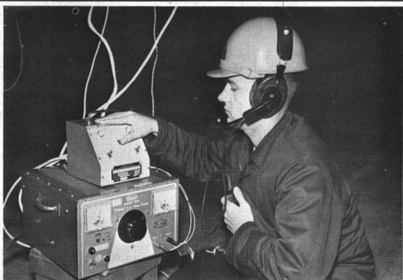
METERS are used to check destruct system during simulated countdown.
