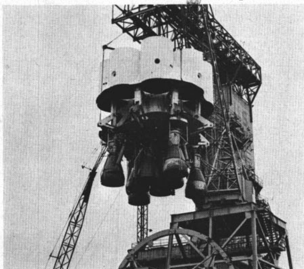
KING-SIZE —Full-scale model of Saturn rocket's power plant is suspended from test tower during NASA testing.
