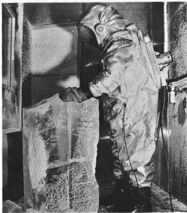
EXPERIMENTAL air-conditioned suit maintains about 80-degree inside temperature in extreme heat and cold tests.
