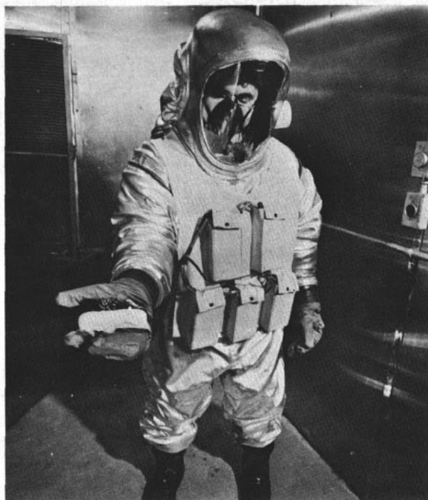
EXPERIMENTAL air-conditioned suit maintains about 80-degree inside temperature in extreme heat and cold tests.
