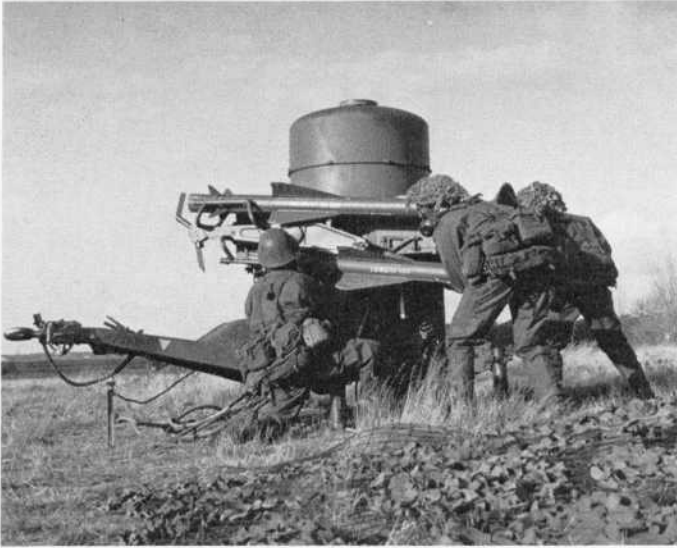
Personnel of No 16 Squadron, RAF Regiment at Wildenrath, reload a Rapier surface-to-air missile fire unit with fresh rounds.
