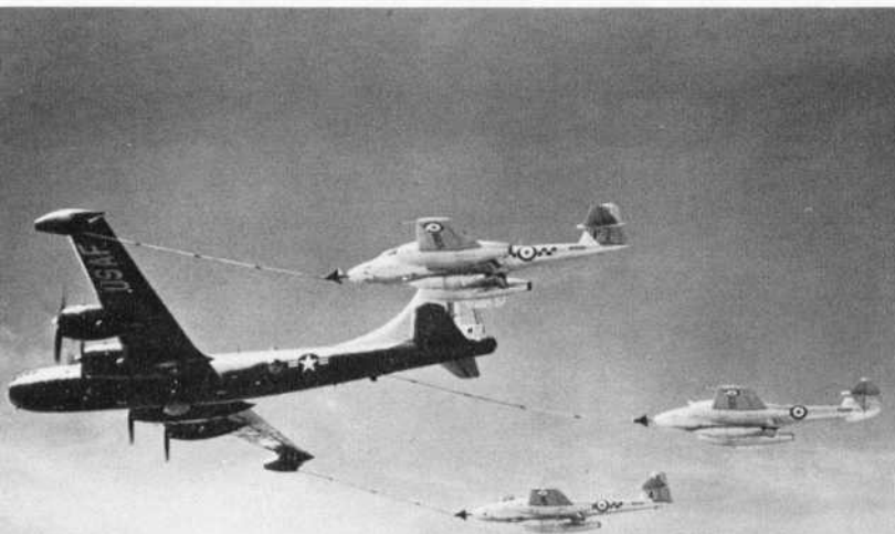
The looped hose method used until 1948 was obviously unsuitable for use by single-seat fighters. Largely at the instigation of the USAF, Flight Refuelling Ltd developed instead the "probe and drogue" method illustrated below. (Right) A trials Meteor 4 with nose-mounted probe approaches the drogue trailed from a tanker and (left) the Boeing YKB-29T, the world's first triple-point tanker, refuels three Meteors, including two Mk 8s of the RAF trials unit, No 245 Squadron, in 1951.
