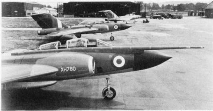
In 1960, two squadrons of Gloster Javelin FAW Mk 9s became the first in Fighter Command to use flight refuelling routinely. As this illustration clearly shows, the probe installation was an inelegant addition to the Javelin's forward fuselage.
