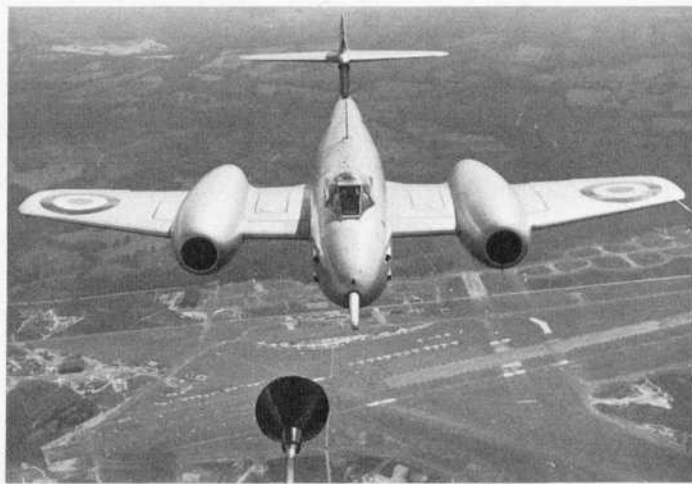
The looped hose method used until 1948 was obviously unsuitable for use by single-seat fighters. Largely at the instigation of the USAF, Flight Refuelling Ltd developed instead the "probe and drogue" method illustrated below. (Right) A trials Meteor 4 with nose-mounted probe approaches the drogue trailed from a tanker and (left) the Boeing YKB-29T, the world's first triple-point tanker, refuels three Meteors, including two Mk 8s of the RAF trials unit, No 245 Squadron, in 1951.
