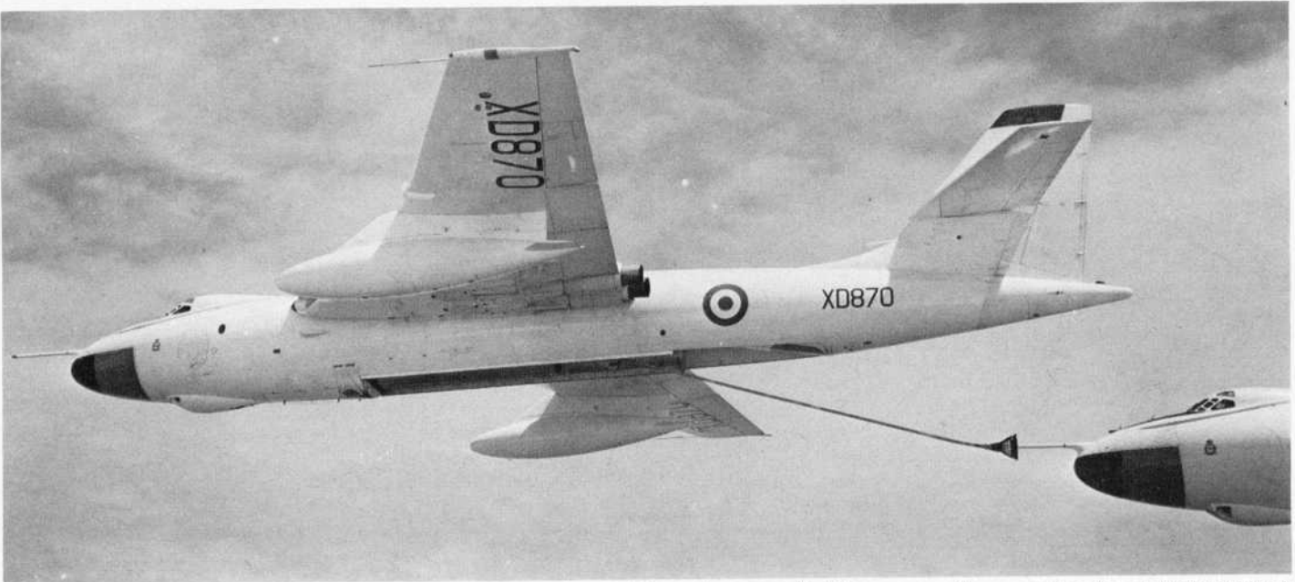
In-flight refuelling was adopted by Bomber Command as an essential complement to its V-Force operations, nearly a decade before Fighter Command was committed to its use. The first tanker for RAF squadron service was the Valiant, converted from the bomber rôle as the BK Mk 1. This photograph shows the single-point refuelling system; a Valiant is also the receiver.
