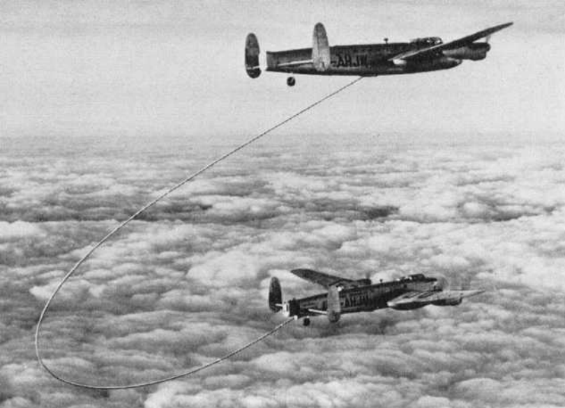
The use of flight refuelling by Lancasters of the Tiger Force to bomb Japan in 1945 was rendered unnecessary by the progress of the war, but the technique that would have been used is shown by this photograph of post-war trials over the South Atlantic. The tanker is the upper aircraft and the refuelling hose has been drawn into the receiver after making contact by means of the ejector method developed by Flight Refuelling Ltd.
