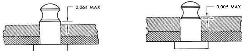
LIMITS FOR POSITION OF SELF BROACHING SHOULDER PRIOR TO INSTALLATION OF COLLAR
