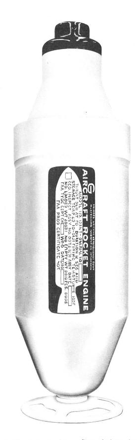
Figure 1-1. 15KS-1000-A1 Aircraft Rocket Engine
