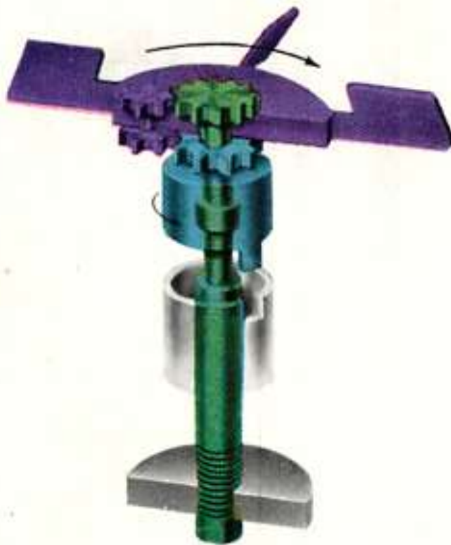
Figure 66. FUZE, bomb, AN-Mk. 219 (nose) — method of arming.
