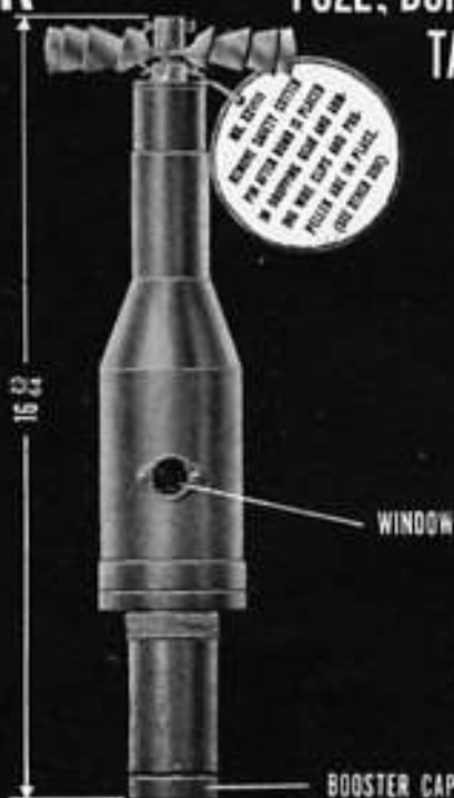
Figure 18 ① and ②. Two Navy tail fuzes, similar in appearance (bottle-shaped) but different in function. AN-Mk. 228 is a vane type, detonator-safe fuze for armor-piercing bombs. It arms after 150 revolutions of the vane, detonates the bomb .08 second after impact.
