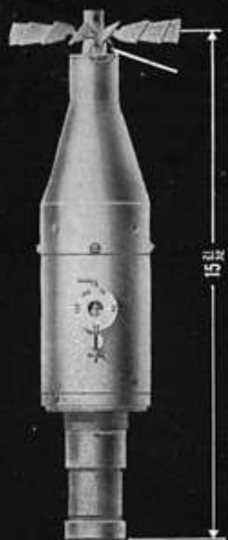
Figure 18 ① and ②. Two Navy tail fuzes, similar in appearance (bottle-shaped) but different in function. AN-Mk. 228 is a vane type, detonator-safe fuze for armor-piercing bombs. It arms after 150 revolutions of the vane, detonates the bomb .08 second after impact.
