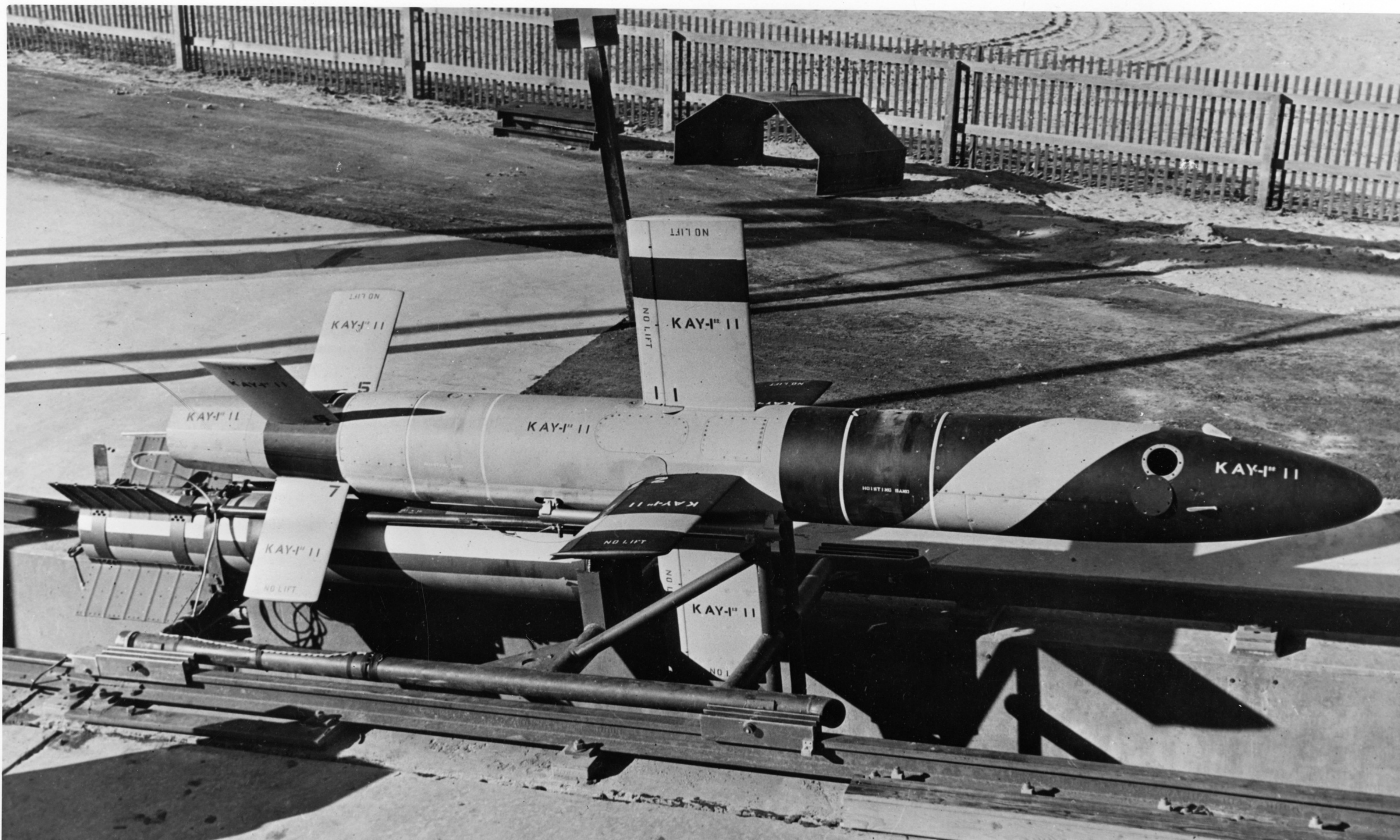
AIRCRAFT SERIAL NO 11 IN FIRING POSITION ON NOTS 450FT @ 8 DEGREES INCLINED RAMP - SIDE VIEW
