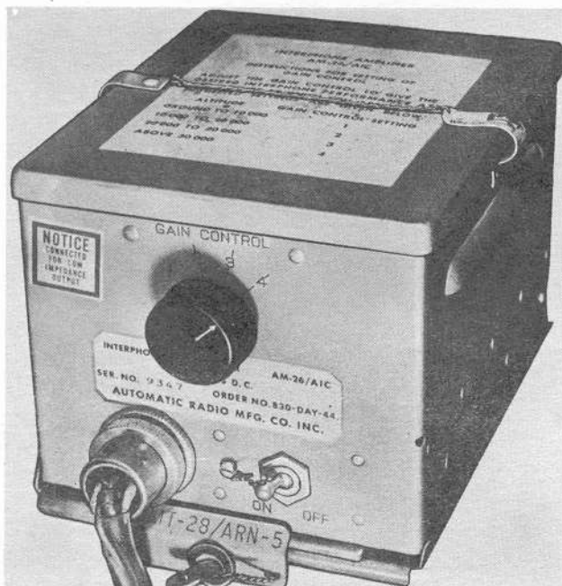
Figure 44 — AN/AIC-2A Interphone Amplifier
