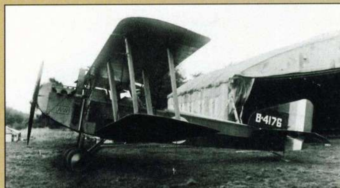
Armstrong Whitworth FK8: Powered by the 160 hp Beardmore engine, the two-seat FK8 served alongside the RE.8 with RFC and RAF squadrons and gave a good account of itself as a sturdy and reliable machine. At the time of the formation of the Royal Air Force, there were five FK8 squadrons on the Western Front.
