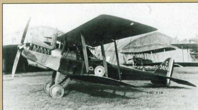
Royal Aircraft Factory RE8: A hard working and unglamorous two-seater, powered by a 140 hp RAF 4A engine, the RE8 equipped more squadrons than any other type on the Western Front at the time of the formation of the Royal Air Force. The RE8 was employed on reconnaissance, artillery observation, photography and bombing work.
