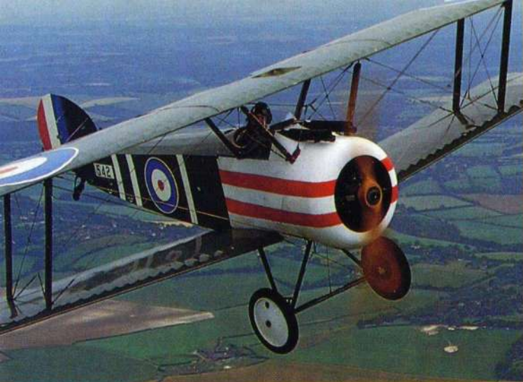
Sopwith Camel: This legendary scout, or fighter, first became operational on the Western Front with the RNAS in July 1917; it soon became notorious as an unforgiving machine, very quick in reaction to control and, thus, highly manoeuvrable in experienced hands. Powered by the 130 hp Clerget, 110 hp Le Rhône, or the Bentley BR.1 of 150 hp. PRM
