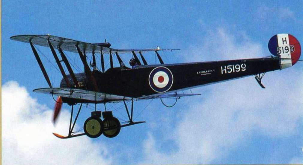
Avro 504K: One of the greatest training aircraft that has ever been produced, the Avro 504K first appeared at Hendon in September 1913 and, virtually unaltered, remained in production throughout the war. In RFC and RAF service, it eclipsed all other types, remaining on charge until the mid 1930s. The Avro 504K had the engine mounting modified so that any contemporary rotary engine could be installed, e.g. Gnome, Le Rhône, Clerget, etc. PRM
