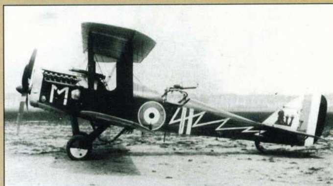
Airco DH.4: Sometimes described as the equivalent of the de Havilland Mosquito of WW2, the DH.4 high-performance day bomber was fitted with various engines but achieved the pinnacle of its success with the 275/375 hp Rolls-Royce engines later named Eagle.
