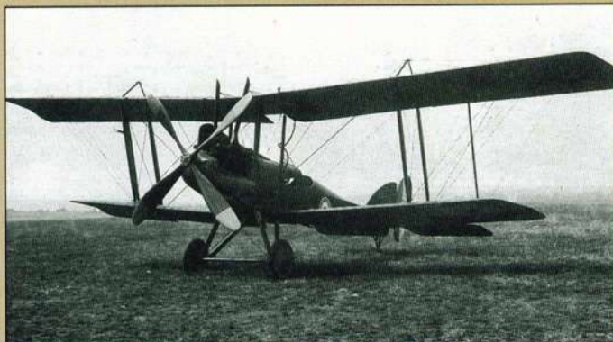
Royal Aircraft Factory BE.12A: To turn the BE2 series of biplanes into a more potent weapon, the more powerful (140 hp) RAF.4A engine was installed and the aircraft entered production as the BE.12 single-seater, with a gun firing through the airscrew. The improved BE.12A was followed by the BE.12B with a 200 hp Hispano-Suiza engine.
