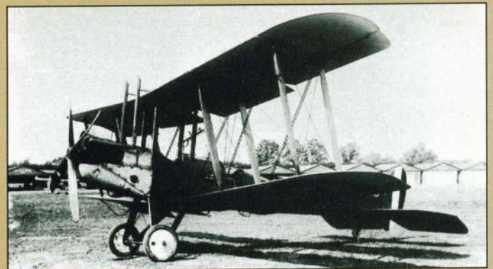
Royal Aircraft Factory BE.2C: An old design, the BE.2C had first served in France in January 1915, and received undue criticism during the period in which the Fokker Monoplane was introduced – this was largely due to exaggerated reports of its 'inherent stability' which made it difficult to throw about.
