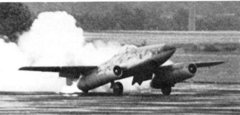
The first Me 262 to fly on jet power alone was the Me 262 V3, seen (above) on its first take-off on 18 July 1942 and (below) landing back at Leipheim, with unburned fuel igniting in the hot jet pipes and spilling onto the runway.
