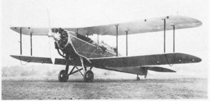
While the RAF standardised on the Wapiti IIA, numerous other variants were developed by Westland for export or special rôles. Above left is the long-fuselage Panther-engined demonstrator for South America while, above right, is the Jaguar-engined Mk IV with split axle undercarriage for China. The four-bladed metal Leitner-Watts propeller on Wapiti J9728 gave the author problems because of its inertia.
