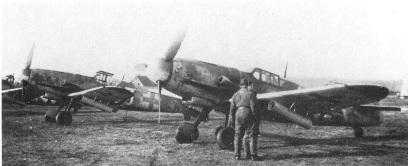
One of the German developments to counter the Allied bombing formations, and especially those of the USAAF's 8th Air Force, was the "Pulk-Zerstörer" (Formation Destroyer), a Wfr.Gr.21 mortar. The Bf 109G-6/R2s (above) carry one of these weapons beneath each wing; the Bf 110G-2/R3 of 9.Staffel of ZG26 (below right) has two beneath each wing.
