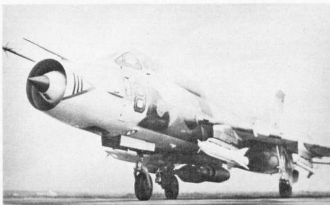
(Above and immediately below) The Sukhoi Su-17 Fitter-H attack aircraft, the example below having a centreline reconnaissance pod which appears to incorporate forward-facing panoramic cameras, an infra-red linescanner and possibly side-looking radar. Some 800 of the variable-geometry Fitter are in Soviet service, together with a similar number of the very much more capable Sukhoi Su-24 Fencer (below right) two-seat deep penetration interdicator and strike aircraft.
