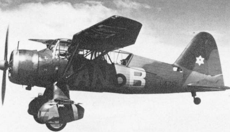
(Above) A pre-war photograph of a Lysander, in its Mk II version with Perseus engine, serving with No 13 Squadron after the adoption, at the time of the Munich Crisis, of squadron code letters. (Below) One of the several Lysander variants was this long-range variation of the Mk III, used to ferry agents beyond enemy lines.
