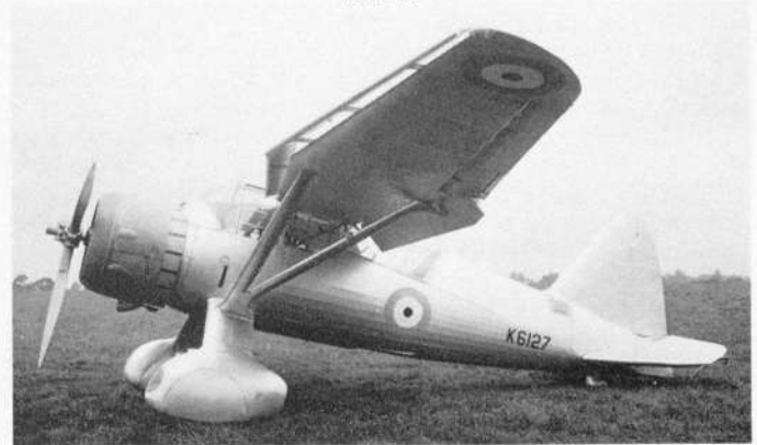
Photographs of the prototype Westland Lysander, for the flight development of which Penrose was responsible. In its first form, above, the tailplane was not adjustable, leading to some handling problems on the approach; after a period of intensive investigation, the tailplane was made variable through a large angle, as shown below.
