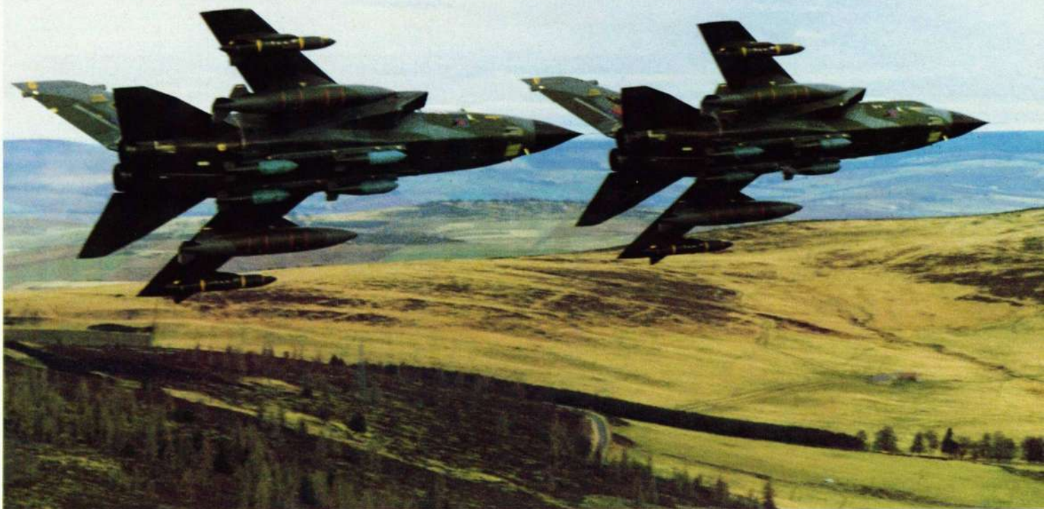
Photographed on a training mission from RAF Honington, each of these Tornado GR Mk 1s (above and bottom right) carry a typical load comprising four 1,000-lb (454-kg) retarded bombs, two 330-lmp gal (1 500-l) drop tanks and two Marconi Sky Shadow electronic countermeasures pods.
