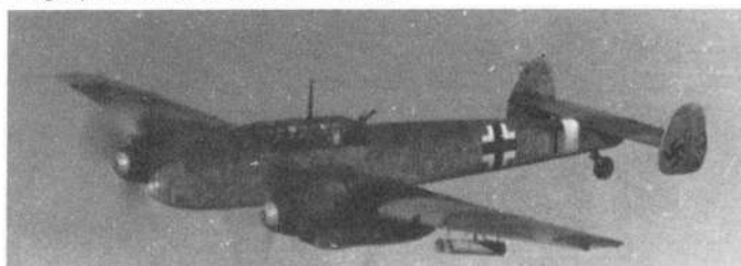
One of the German developments to counter the Allied bombing formations, and especially those of the USAAF's 8th Air Force, was the "Pulk-Zerstörer" (Formation Destroyer), a Wfr.Gr.21 mortar. The Bf 109G-6/R2s (above) carry one of these weapons beneath each wing; the Bf 110G-2/R3 of 9.Staffel of ZG26 (below right) has two beneath each wing.
