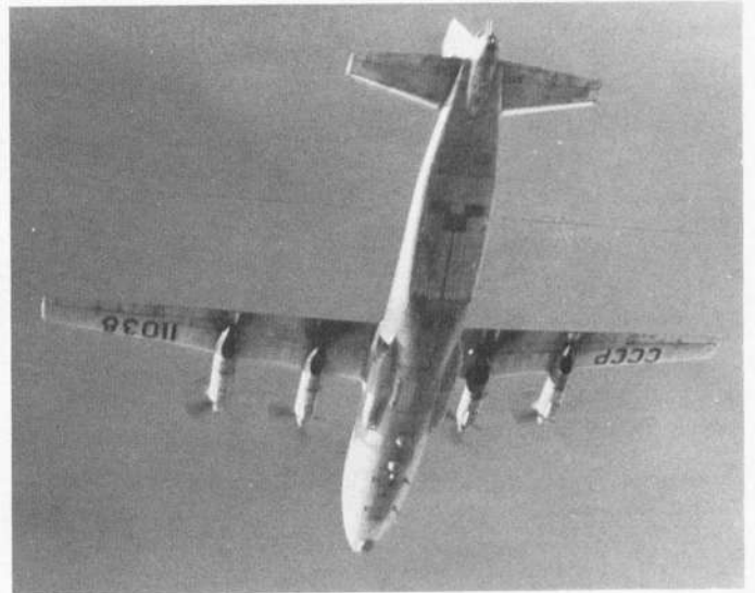
Several versions of the An-12BP Cub military transport adapted for electronic intelligence and electronic countermeasures tasks are in service, usually carrying civil registrations, one such being the Cub-B Elint aircraft illustrated above.
