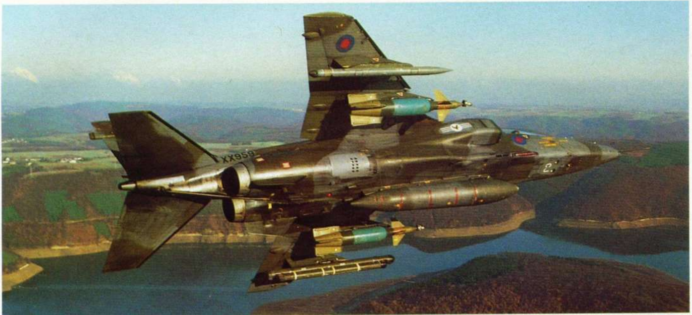
(Above) Jaguar GR Mk 1s operating in RAF Germany have been progressively modified at Bruggen to permit the carriage of additional wing-mounted stores, with a consequent significant advance in their operational capability. This Jaguar of No 20 Squadron shows three of the new items — laser-guided bombs, PHIMAT chaff dispenser and AN/ALQ-101-10 ECM pod. The Tracor AN/ALE 40 flare dispenser can also now be carried. (Below left) The BAe 146 entered service with the RAF during June.
