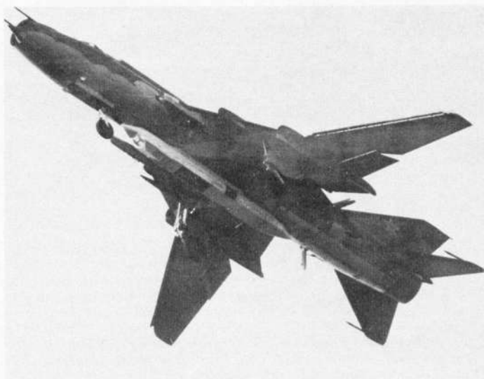
(Above and immediately below) The Sukhoi Su-17 Fitter-H attack aircraft, the example below having a centreline reconnaissance pod which appears to incorporate forward-facing panoramic cameras, an infra-red linescanner and possibly side-looking radar. Some 800 of the variable-geometry Fitter are in Soviet service, together with a similar number of the very much more capable Sukhoi Su-24 Fencer (below right) two-seat deep penetration interdicator and strike aircraft.
