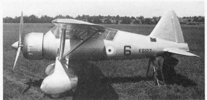
Photographs of the prototype Westland Lysander, for the flight development of which Penrose was responsible. In its first form, above, the tailplane was not adjustable, leading to some handling problems on the approach; after a period of intensive investigation, the tailplane was made variable through a large angle, as shown below.
