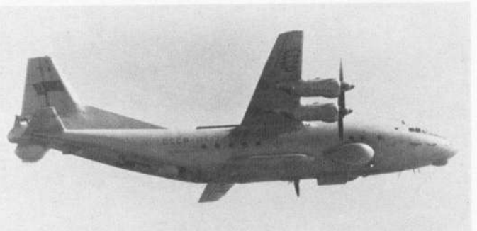
Other variants of the An-12 include the Cub-D electronic countermeasures aircraft, illustrated above, and what appears to be a test and evaluation anti-submarine warfare model, seen below, with electronic extensions forward of the nose and aft of the tail.
