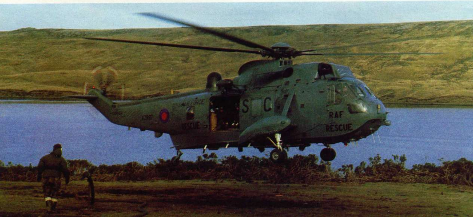
(Below) Detached as "C" Flight from No 202 Squadron in the UK, the SAR Sea King HAR Mk 3s now sport an overall grey finish, unlike their canary-yellow home-based counterparts, and form No 1564 Flight at Stanley. RWR equipment, on the nose and under the tailboom, is an addition for Falklands operations.
