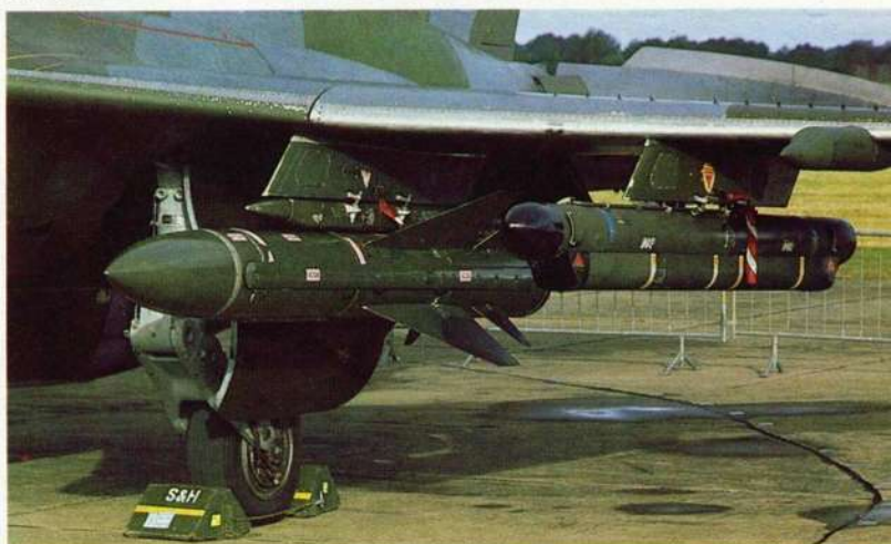
(Above) The Buccaneer, no longer in service in RAF Germany, is expected to continue to play a significant rôle in No 18 Group's inventory for a number of years yet, with the addition of Sea Eagle to its armament fit. (Below) The anti-radar Martel ASM and AN/ALQ-101 jamming pod on a Buccaneer.
