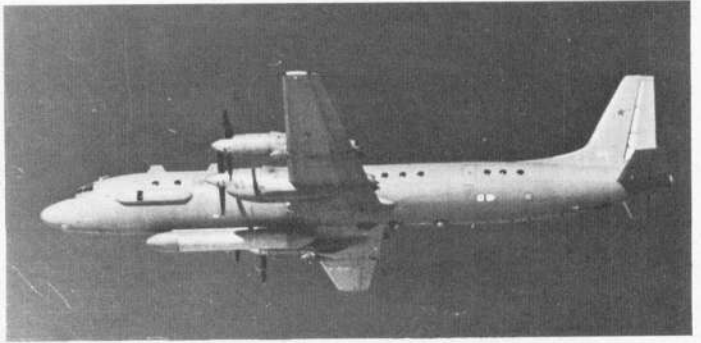
Two derivatives of the mid-'fifties vintage Il-18 Coot medium-range airliner currently perform important rôles in the Soviet Air Force and Soviet Naval Aviation, these being the Il-20 Coot-A (above) and the Il-38 May (left). Coot-A is a conversion of the standard airliner for electronic countermeasures and electronic intelligence tasks. May is a maritime surveillance derivative of the airliner and is seen (immediately left) in its initial May-A form and (above left) in its more recent May-B version with an additional radome under the forward fuselage. The Soviet Navy is believed to be deploying about 60 May maritime surveillance aircraft.
