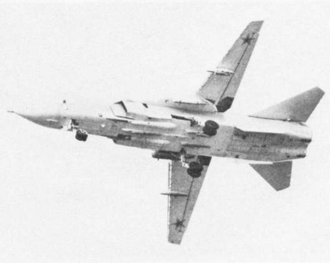
(Above and immediately below) The Sukhoi Su-17 Fitter-H attack aircraft, the example below having a centreline reconnaissance pod which appears to incorporate forward-facing panoramic cameras, an infra-red linescanner and possibly side-looking radar. Some 800 of the variable-geometry Fitter are in Soviet service, together with a similar number of the very much more capable Sukhoi Su-24 Fencer (below right) two-seat deep penetration interdicator and strike aircraft.
