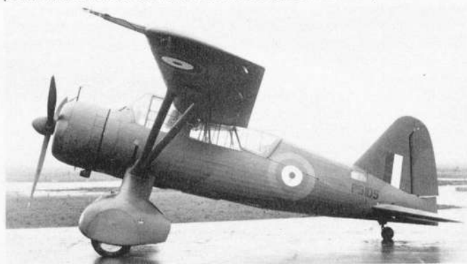
Two extreme modifications of the Lysander with the testing of which the author was concerned — (above) with the Stieger monospar wing fitted by Blackburn Aircraft, and (below) with Delanne tandem wing layout and a tail turret.
