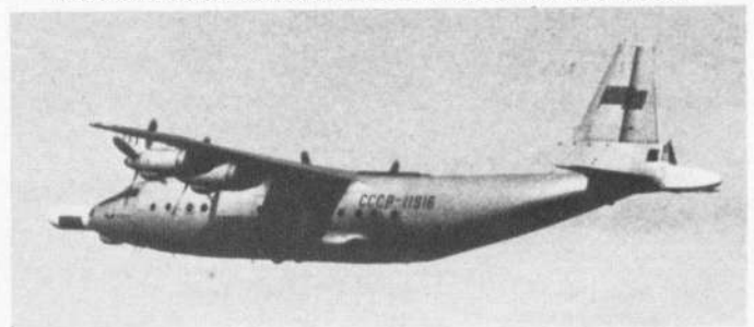
Other variants of the An-12 include the Cub-D electronic countermeasures aircraft, illustrated above, and what appears to be a test and evaluation anti-submarine warfare model, seen below, with electronic extensions forward of the nose and aft of the tail.
