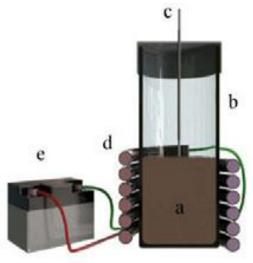
Schematic representation of a simple non-adiabatic measurement setup with a) ferrofluid sample; b) sample holder; c) temperature sensor; d) coil system; and e) power supply.
