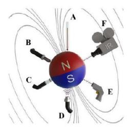
Schematic representation of used calorimetric temperature sensors. Probes which require contact with the sample are A) Alcohol thermometer, B) Thermocouple, C) Fiber-optic cable, and D) Ultrasonic sensor. Contactless sensors are E) Pyrometer and F) IR camera
