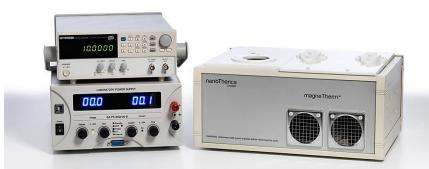
Frequency range: 0.1-1 MHz Coils: 2-70 loops Field Strength up to 64 kA/m
