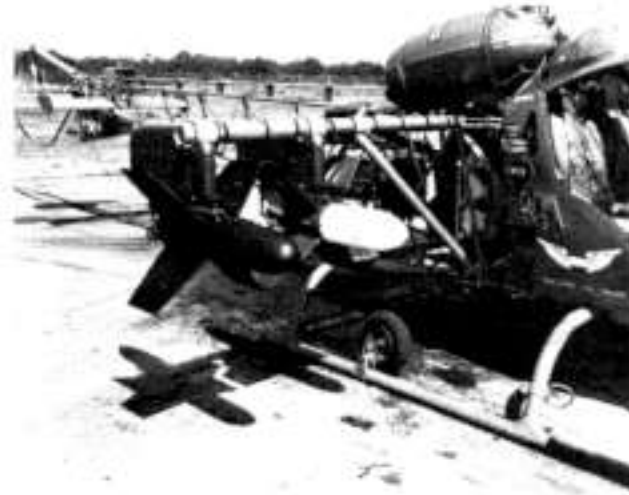
The Oh-13, testbed for SS-10 anti-tank guided missiles, paved the way for today's anti-armor helicopters.
