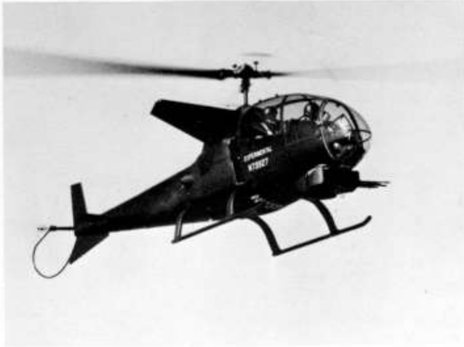
In 1963 the company sponsored Sioux Scout demonstrated the benefits of tandem seating, slim silhouette and a chain mounted turret.
