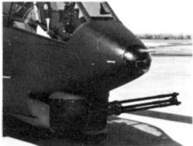
Originally qualified on the AH-1G, the XM-97 20mm turret is standard on the U.S. Marine's AH-1J SeaCobra.
