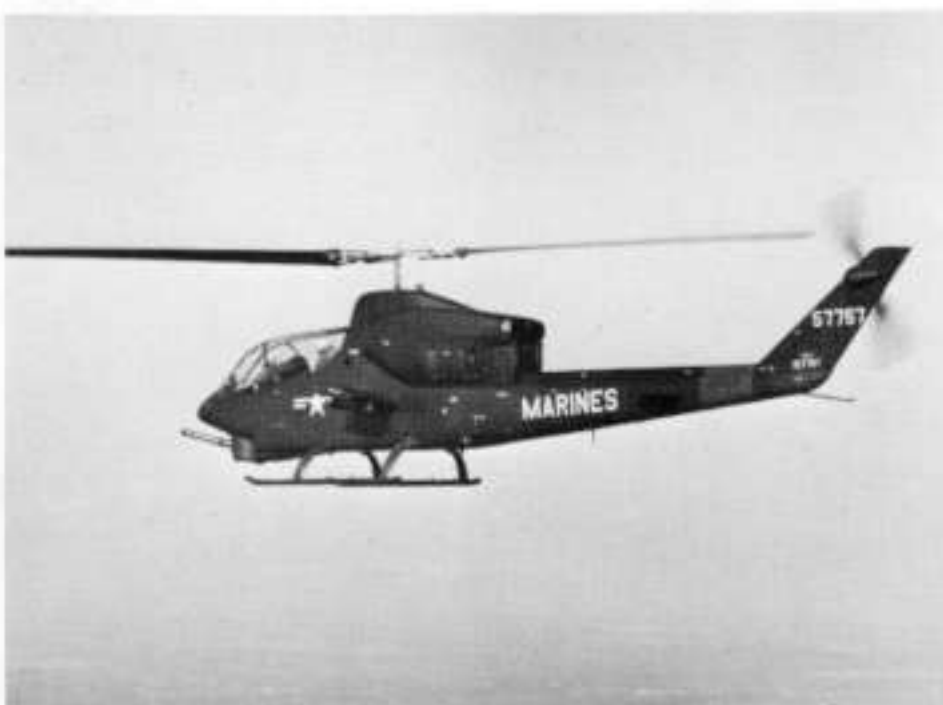
The twin engine AH-1J SeaCobra was developed to meet U.S. Marine requirements. Deliveries started in June 1969, six months after first flight.
