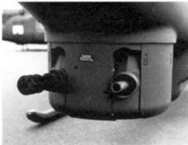
Operational in late 1967, the XM-28 turret replaced the single gun TAT-102 with a 7.62mm mini-gun and a 40mm grenade launcher.
