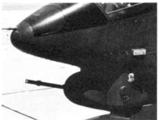
In 1970 Bell confirmed the airframe-systems compatibility of the AH-1G and the XM-102 turret with its XM-140 30mm gun.
