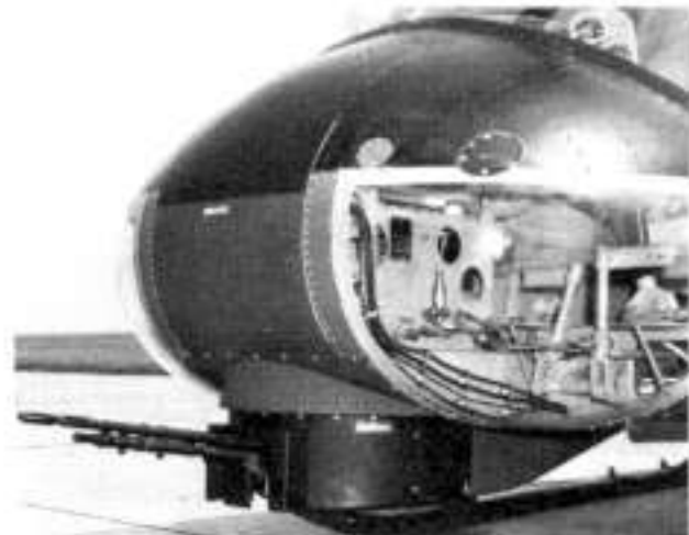
Mounting two M-60 machine guns, the TAT-101 was the first operational chin turret developed for Hueys.
