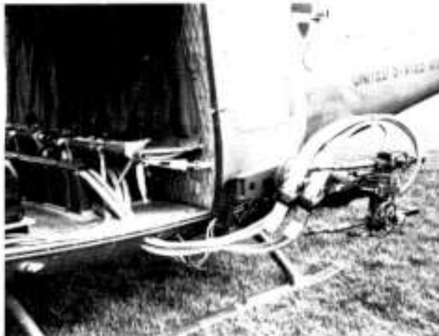
In 1962 the M-6 with its flexible quad machine guns, provided suppressive fire for UH-1B's and UH-1D's.
