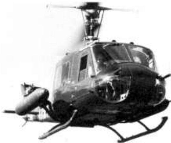
The Army/Bell team developed this XM-14 fifty caliber machine gun installation.
