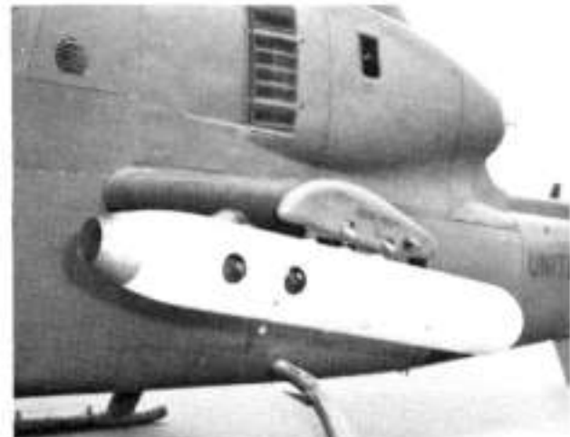
The XM-18E1 7.62mm minigun pod with 1500 RDS of ammunition is just one of the HueyCobra's wing stores.
