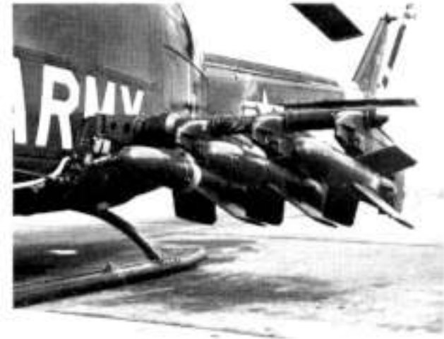
The M-22 missile system (SS-11 missiles) was mounted on the Huey to deliver highly mobile fire power against hard point targets.
