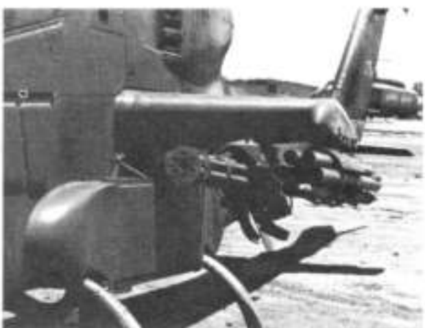
The wing mounted company sponsored XM-35 20mm system became operational in 1969. Ammunition capacity is 1000 rounds.
