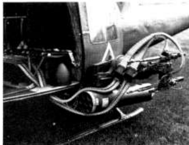
As a result of field experience 2.75" rocket pods were combined with the XM-6 quad gun kit to form the M-16 armament subsystem.
