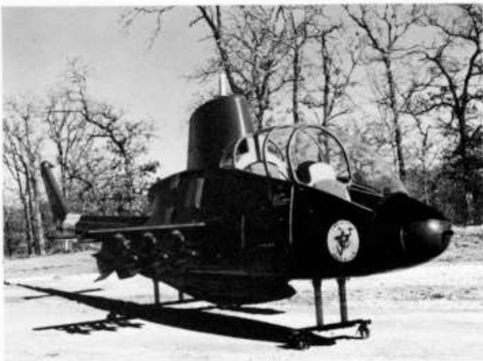
The Bell Warrior, proposed in 1962, was a high performance weapons system designed around UH-1 components for mid-intensity missions.
