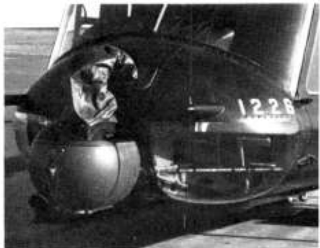
Developed in 1964, the M-5 system with 40mm grenade launcher proved to be an effective means of delivering anti-personnel fire.
