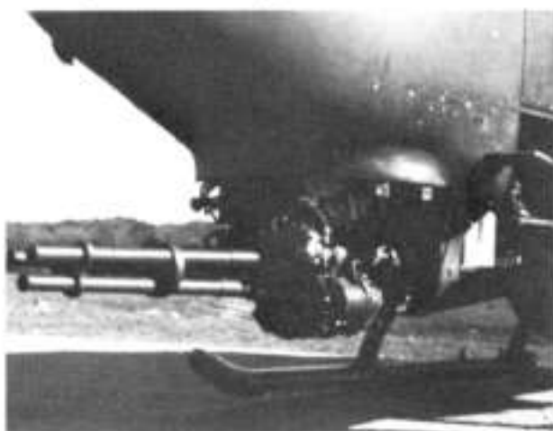
A company sponsored 30mm gatling gun, the XM-188, was tested in 1967. Another example of company sponsored weapon R&D.
