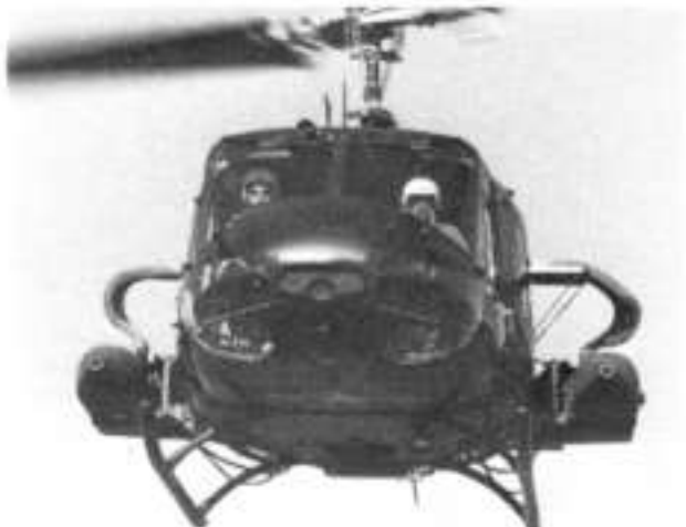
The twin gun XM-30 system was used to develop and qualify the XM-140 30mm cannon.
