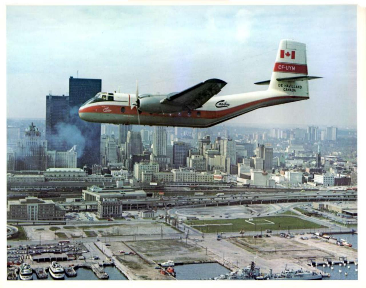
The DHC-4 Caribou transport developed and produced by de Havilland Canada was the first STOL aircraft in the world able to operate from 1,000 ft. strips with a four ton payload. First produced in 1958 more than 300 Caribou are used around the world from the arctic to the tropics. The Caribou is powered by two R.2000 Pratt & Whitney radial engines.
