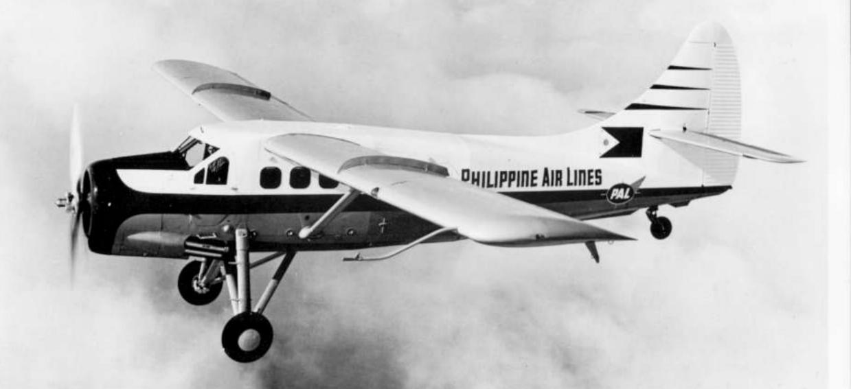
The DHC-3 Otter developed in 1951 was de Havilland Canada's 'stretched version' of the former DHC-2 Beaver. Seen here in Philippine Air Lines markings the Otter has the same STOL (short take-off and landing) characteristics as the Beaver, yet carries twice the payload. The Otter carries 11 passengers or one ton of cargo and is powered by a Pratt & Whitney R.1340 radial engine.
