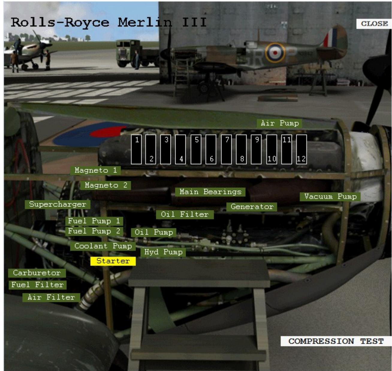
At the lower right is a “Compression Test” button, which tells your mechanic to run a high-pressure air test on the engine cylinders, checking for leaks past the cylinder rings. A civilian may choose to replace a cylinder that is only showing modest wear, perhaps in the 50-60psi range, whereas the military could allow a plane to fly with a cylinder as low as 30 psi.
