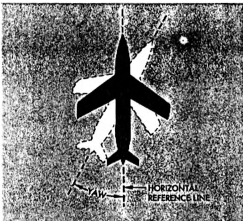
Figure 5-10. Horizontal Reference Line Showing Deviation about Yaw Axis
