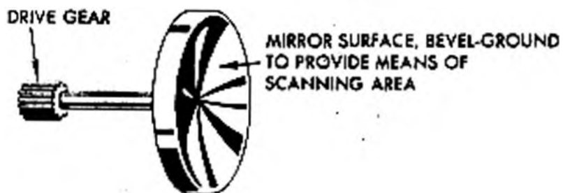
Figure 6-35. Vibrating Mirror used for Scanning
