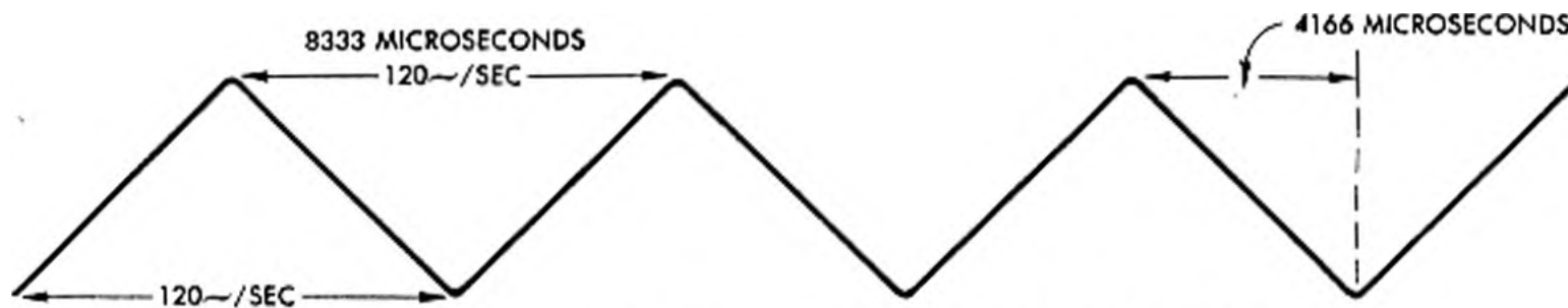
Figure 4-105. Time Relationship of 120 Hz Triangular Wave
