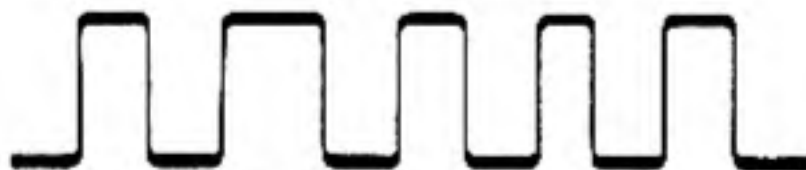
Figure 4-98. Amplified Output of Limiter and Clipper
