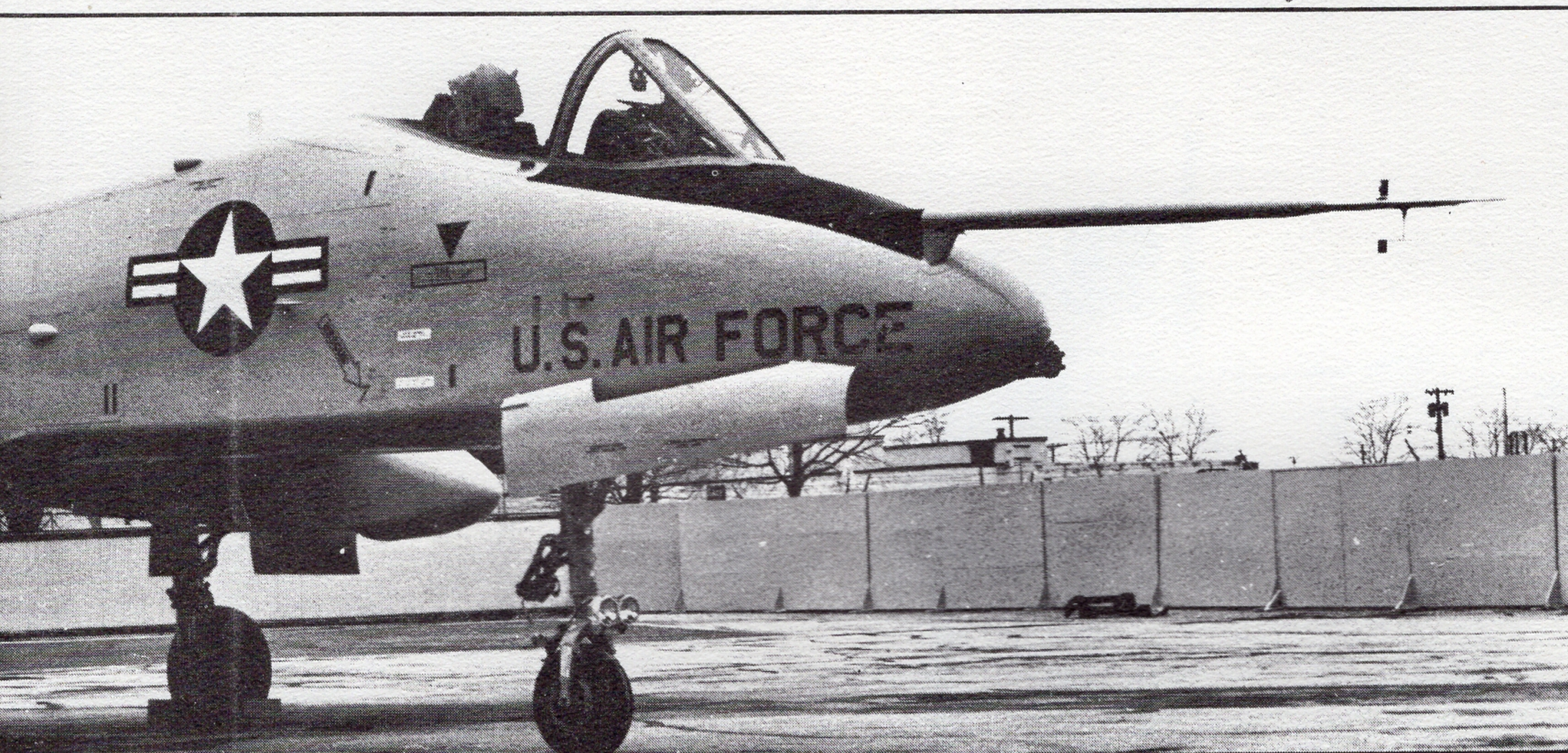
USAF's A-10 close-support aircraft, now in preproduction, is a single-seat, twin-engine design optimized for survivability, weapons delivery, and long loiter time.
