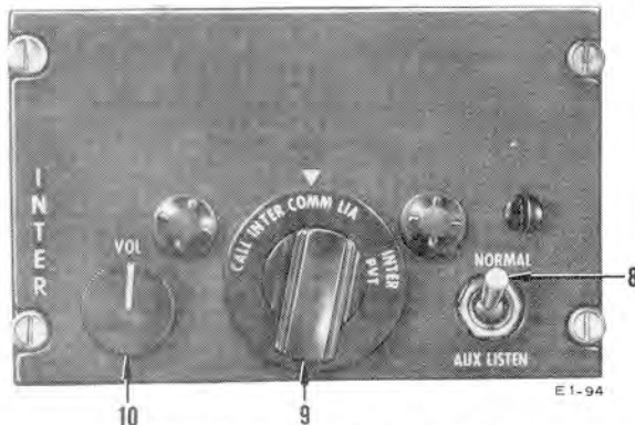
INTERPHONE CONTROL PANEL (CELESTIAL NAVIGATION STATION B-52C)
