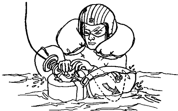
3 Sit on seat facing flotation collar. Using elbows, separate LPU waist lobes and pull shaft of penetrator close to chest.
