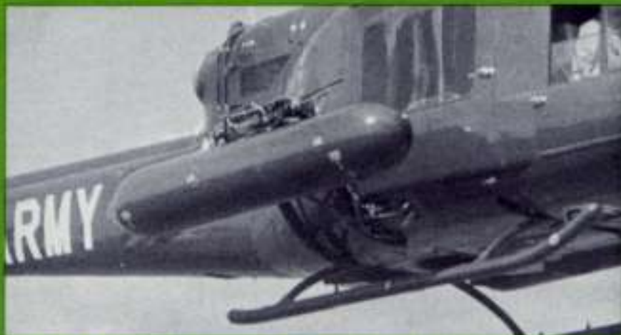
Both 60 and 100-gallon external fuel tanks are being qualified for HU-1B and HU-1D helicopters.
