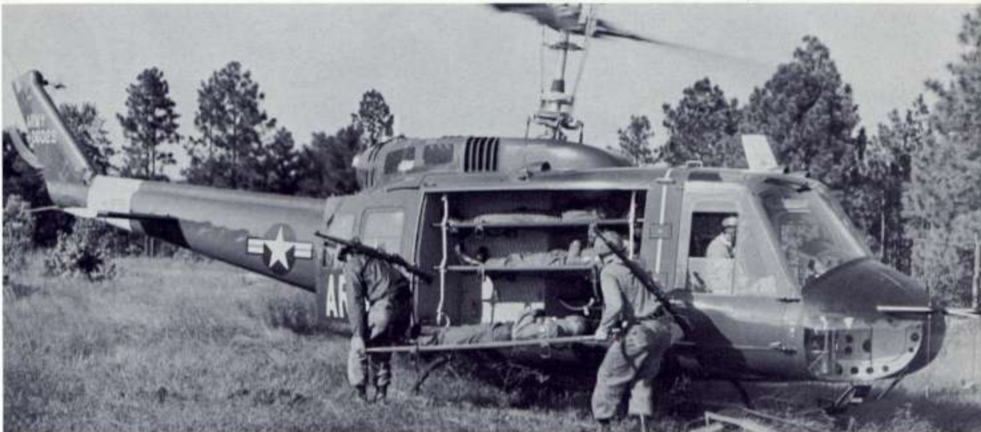
With six litters, HU-1D carries twice as many wounded as other Iroquois models. Wide cabin doors simplify simultaneous loading from both sides.
