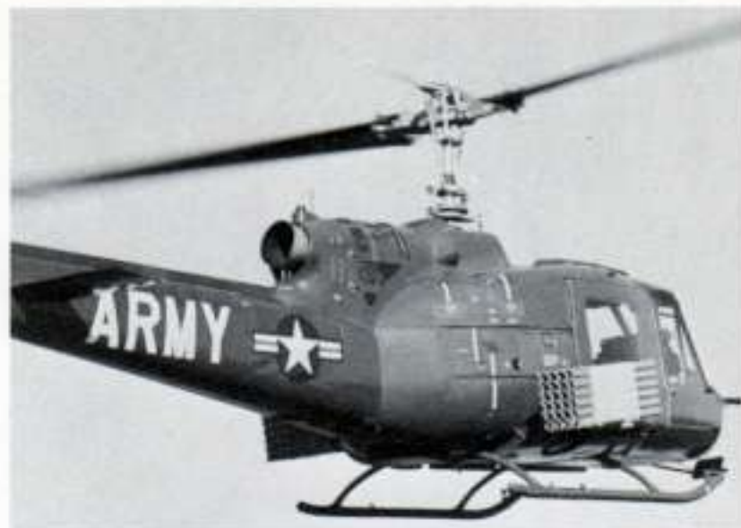
Twin pods holding total of 48 2.75-inch folding fin aircraft rockets provide lethal punch for HU-1B.
