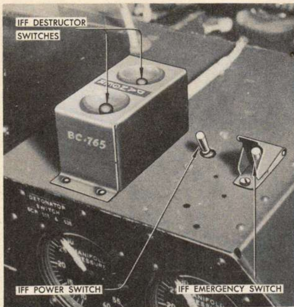
Figure 87 — IFF Control Switches Above Pilot's Instrument Panel
