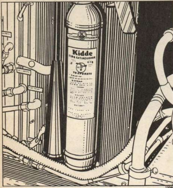
Figure 56 — Hand Type Fire Extinguisher
