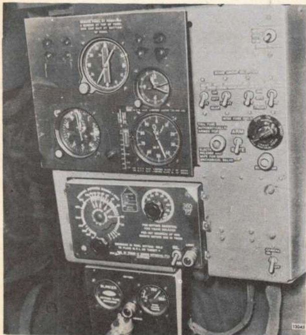
Figure 94—Bombardier's Control Panel— Early Airplanes.
