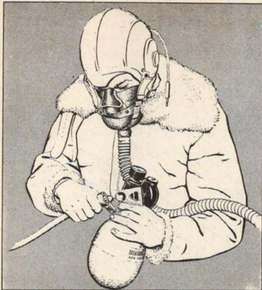
Figure 75 — Filling Portable Bottle
