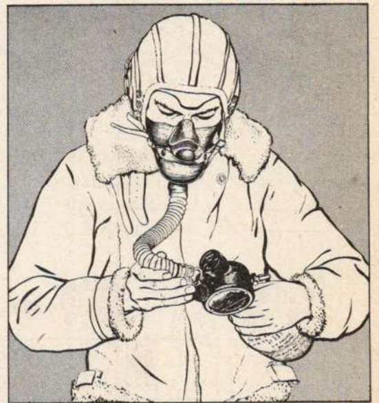
Figure 77 — Connecting Portable Bottle
