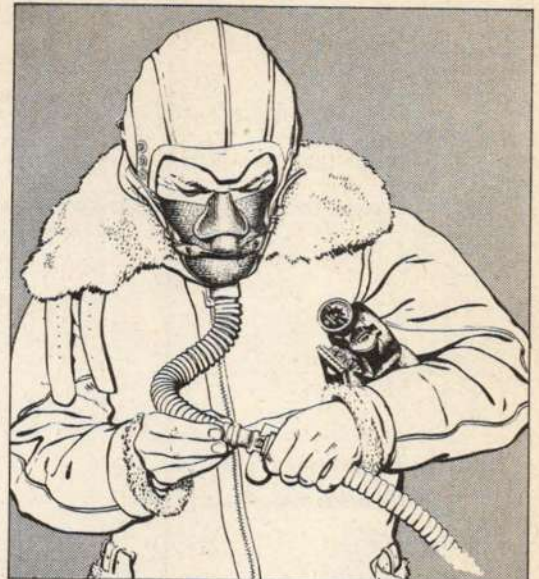
Figure 76 — Disconnecting from Regulator
