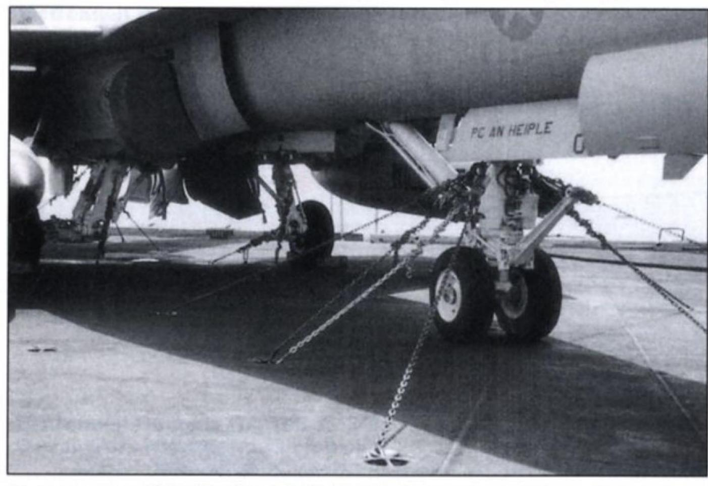
A close-up shot showing details of the nosewheel undercarriage unit and its tie-downs. (Andy Sheppard)
