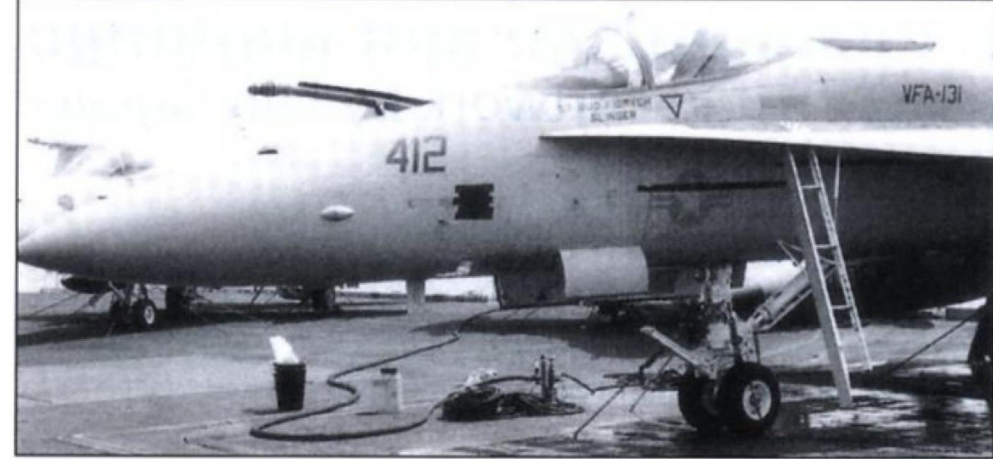
The forward fuselage of an F/A-18C, showing the inflight refuelling probe, boarding ladder, and various antennae. Note the black tape over the rescue panel and other panel edges. (Andy Sheppard)
