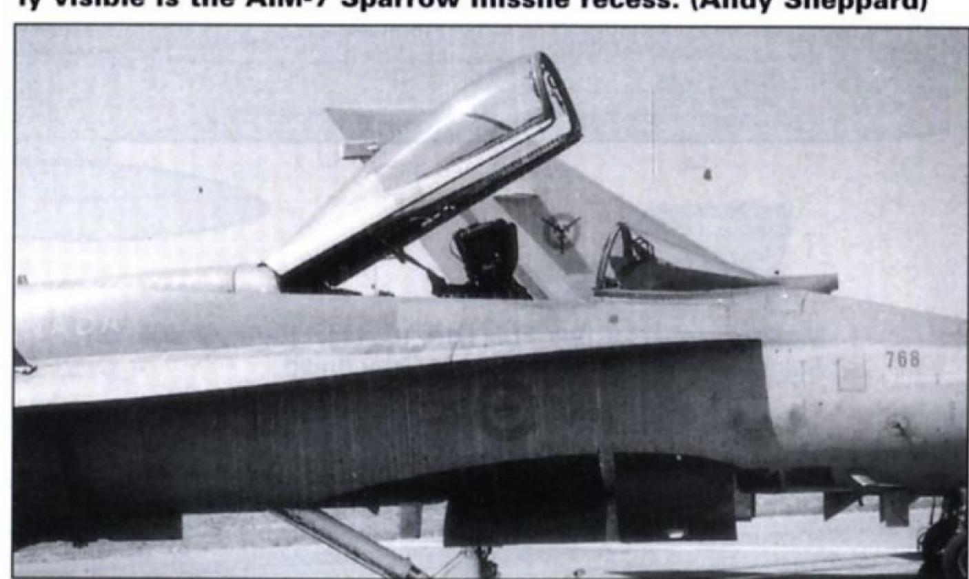
This close-up of a Canadian machine shows not only the canopy in the open position, but also the 'false' painted one underneath.
