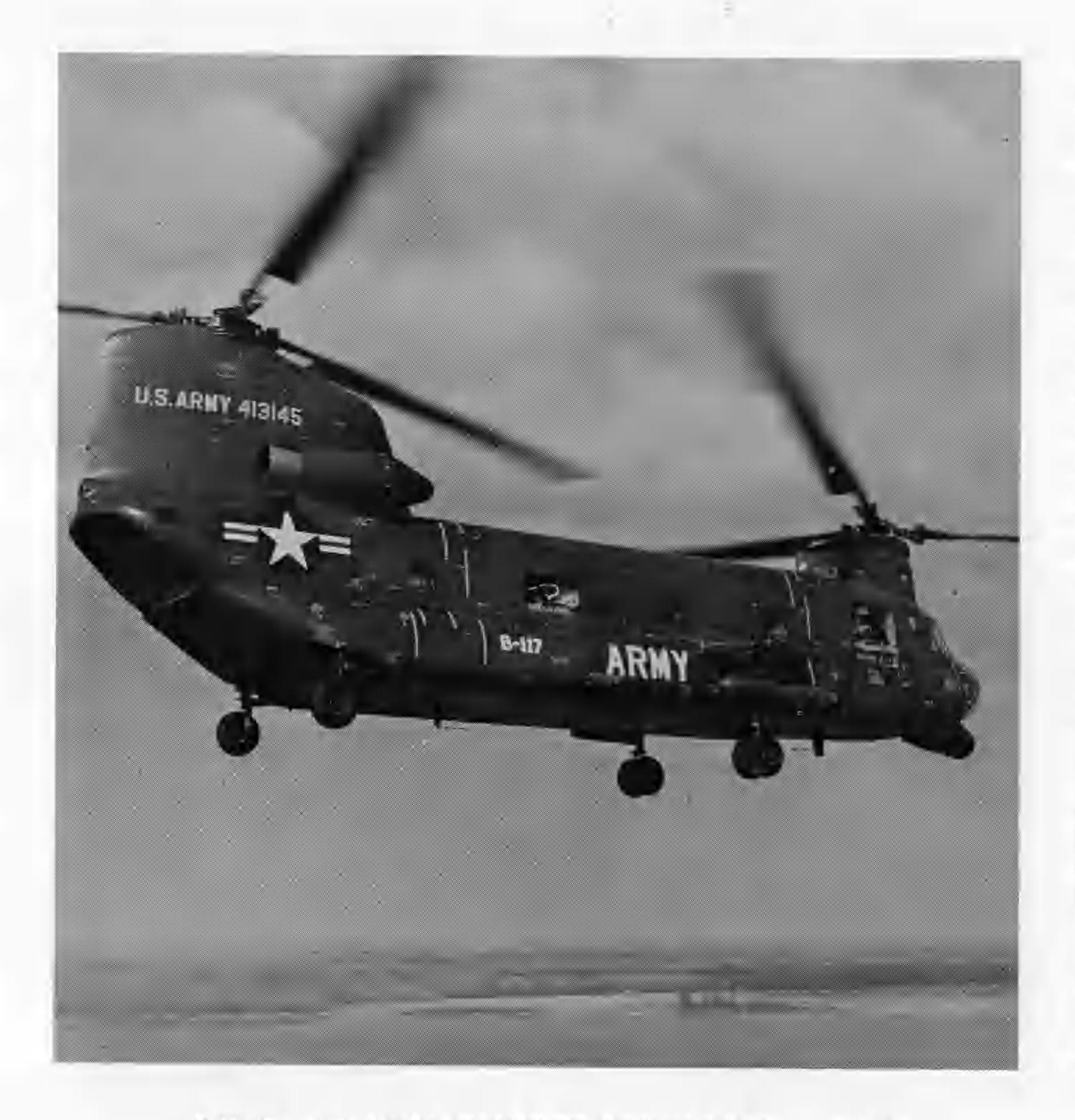
/Armored Chinook uses its payload capability to advantage by mounting an extensive array of armament, as well as armor to protect the crew and vital parts of the aircraft against heavy caliber ground fire.
