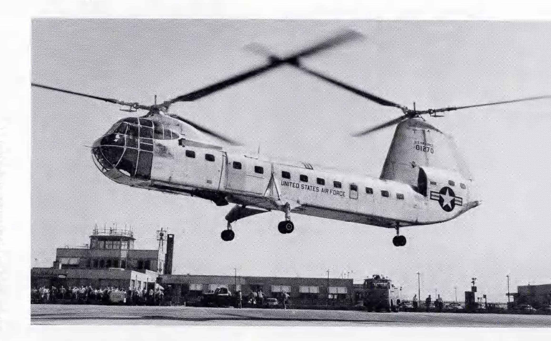
The YH-16A unofficially broke the existing helicopter record in 1956 with a speed of 166 miles per hour. Its service ceiling was over 18,000 feet. Data gathered from ground and flight tests of the YH-16A were instrumental in the further development of large turbine-powered, tandem-rotor helicopters.
