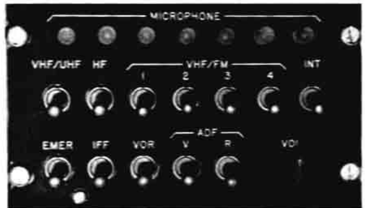
Fig. 1-36 Signal Distribution Panel
