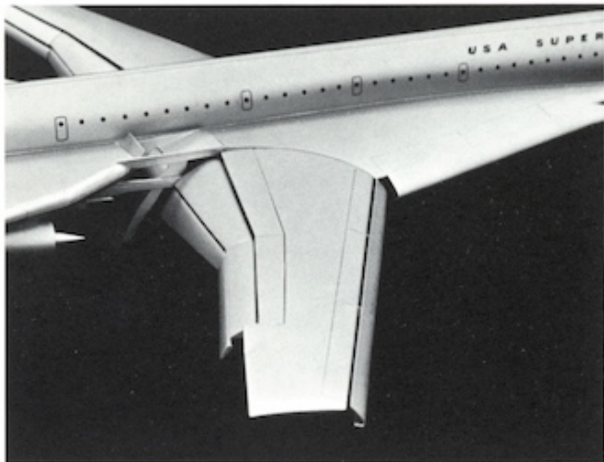
High-lift devices make the airplane stable and easy to handle during low-speed takeoff, approach and landing.
