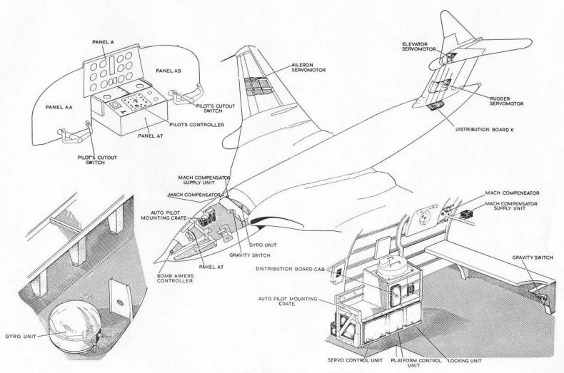
Fig. 2 Auto-pilot components location
