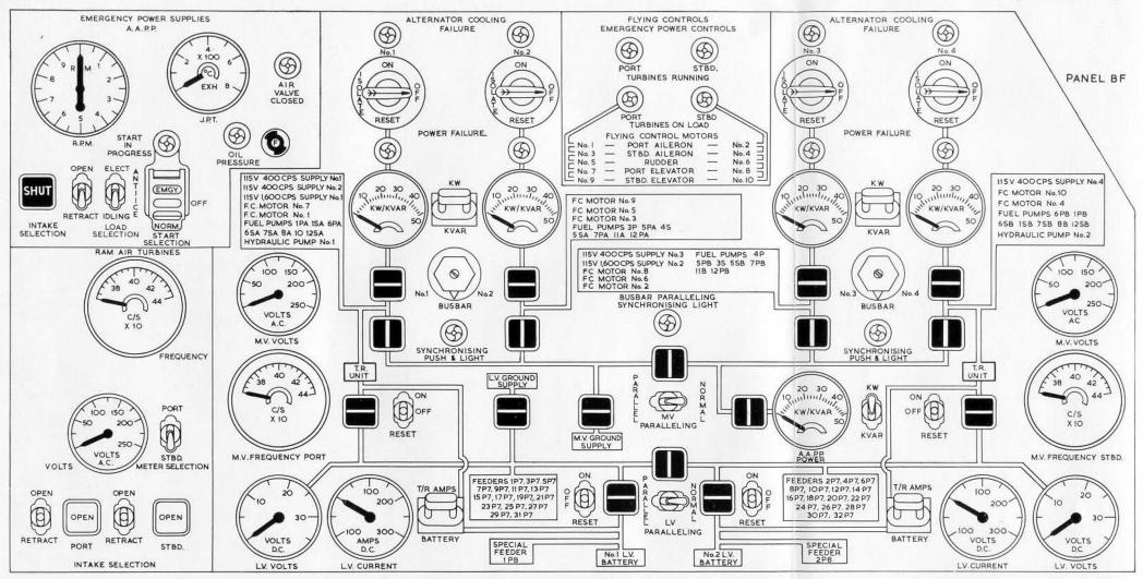
Fig. 1 Generating system, controls and indicators (Pre-Mod. 3904)
