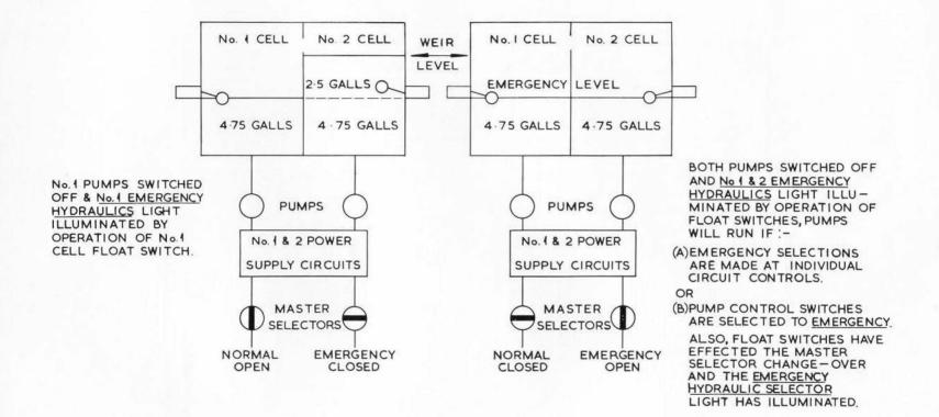
Fig. 2 Hydraulic fluid levels under fault conditions
