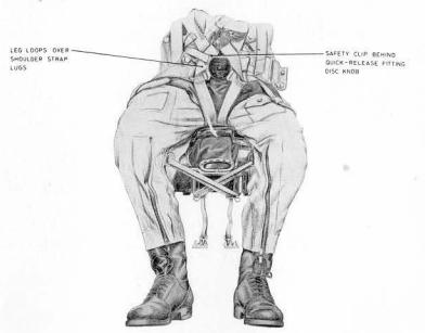
Fig. 4 Leg restraint
