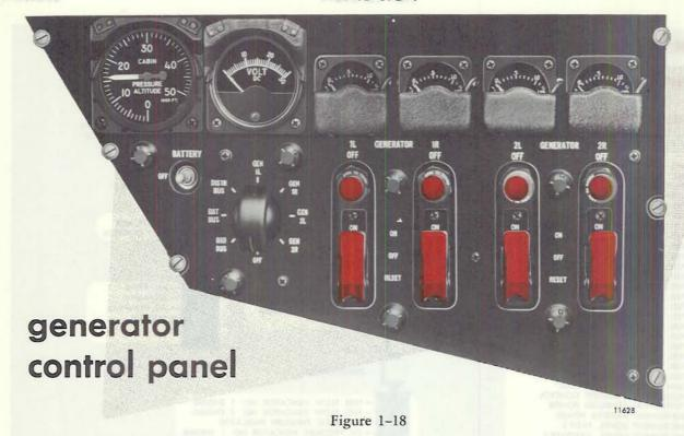
is connected to the airplane. The generator field excitation circuit incorporates a trip relay (circuit breaker) which protects the circuit against overvoltage and shorting. Placing the generator switch in RESET closes the trip relay. If, upon placing the generator control switch in ON, there is no indication on the generator loadmeter, hold the switch in RESET
