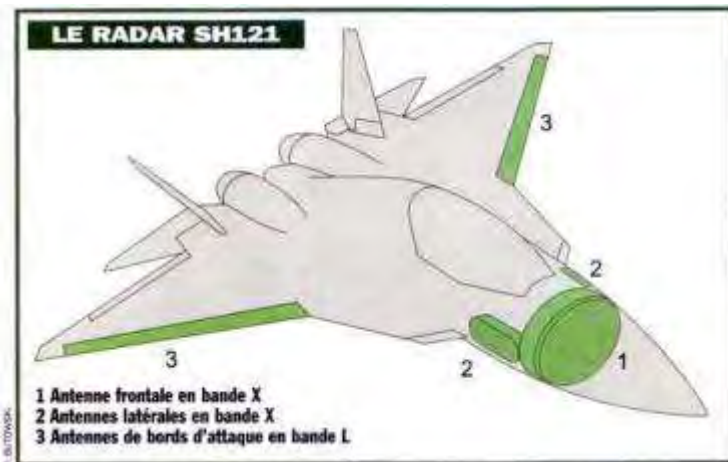
NIIP L-band AESA Radar for PAK-FA and Su-35
