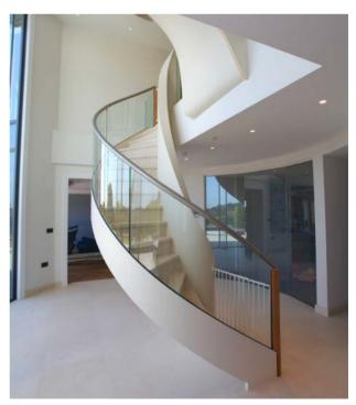
This seamless arc was really worth the extra time and effort put into designing and making it, fabricated in steel for strength and clad in specially imported Pietra Plana stone that match the floor tiles Spiral supplied for that flawless finish. This kind of attention to detail doesn't come cheap, with a guide price of around £95k, but the beauty of bespoke is your staircase can be matched to your budget as well as your dreams.
