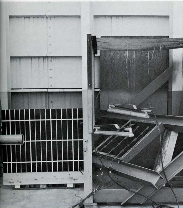
Chicken's speed as it contacts the frame-mounted test windshields is computed by analysis of high-speed films.
