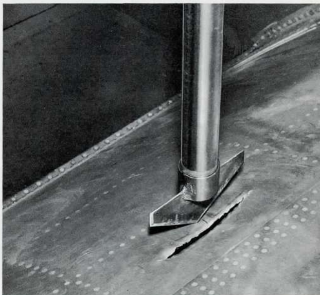
A test section of fuselage skin under pressure is subjected to the javelin test.
