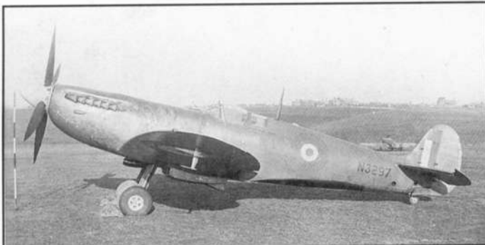
Development aircraft N3297 here fitted with the Merlin 61 engine, and extended nose and retractable tailwheel, configured as a Mk VIII. Crown copyright
