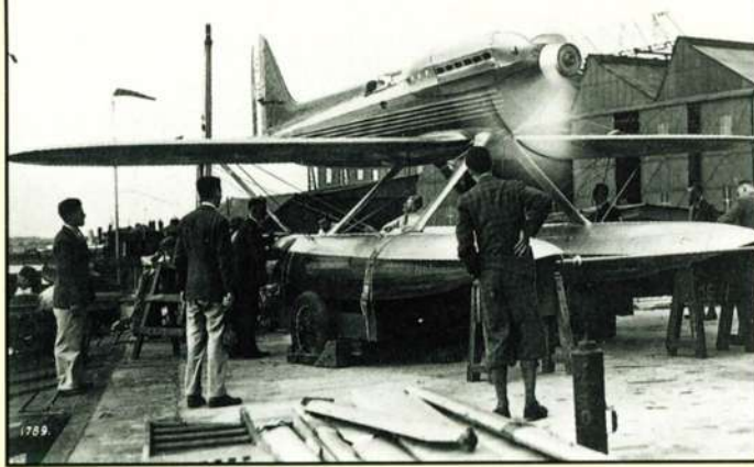
▲ R. J. Mitchell's Schneider Trophy racing seaplanes contributed greatly to the advance of aerodynamics and to the Spitfire design. Supermarine S6B S1595 was used by Flt Lt J. W. Boothman to win the Trophy outright, and then by Flt Lt G. H. Stainforth who, on 29th September 1931, established a World Speed Record at the then unbelievable speed of 407.5mph. Real Photographs
