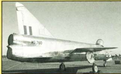
The forerunner of the Lightning — English Electric P1 WG760. Peter R. March
