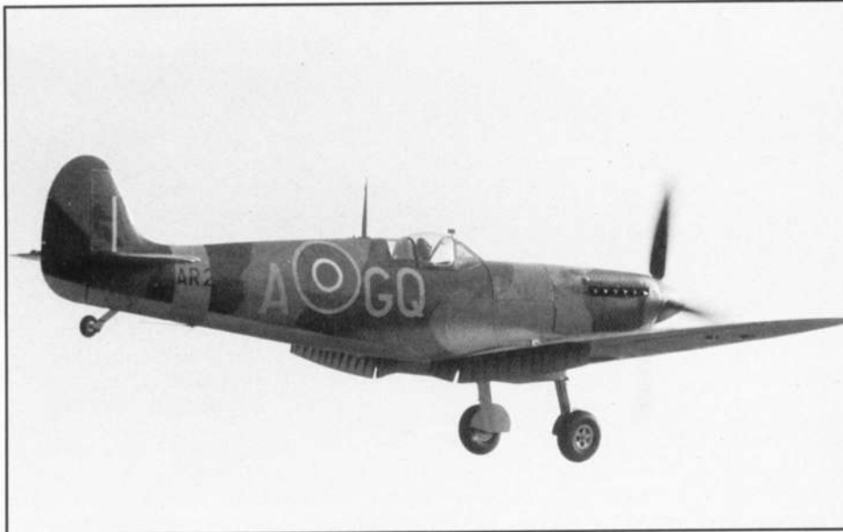
This landing Spitfire IA shows the type's narrow stalky undercarriage. Peter R. March
