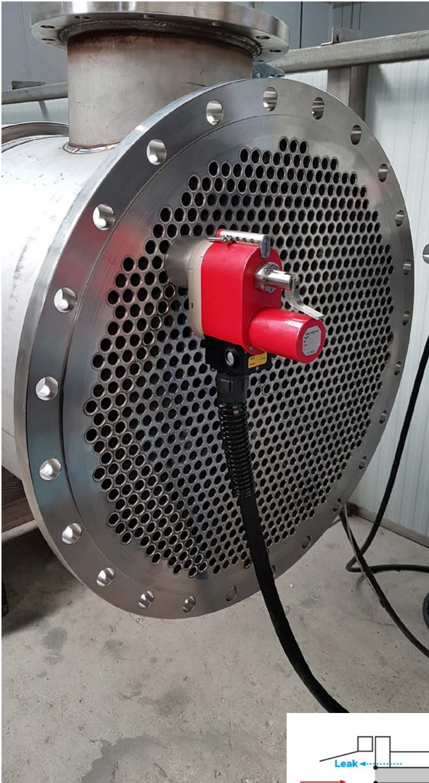
The tube plate (or tube sheet) is the point at which the tubes in the heat exchanger are welded to the end of the vessel
