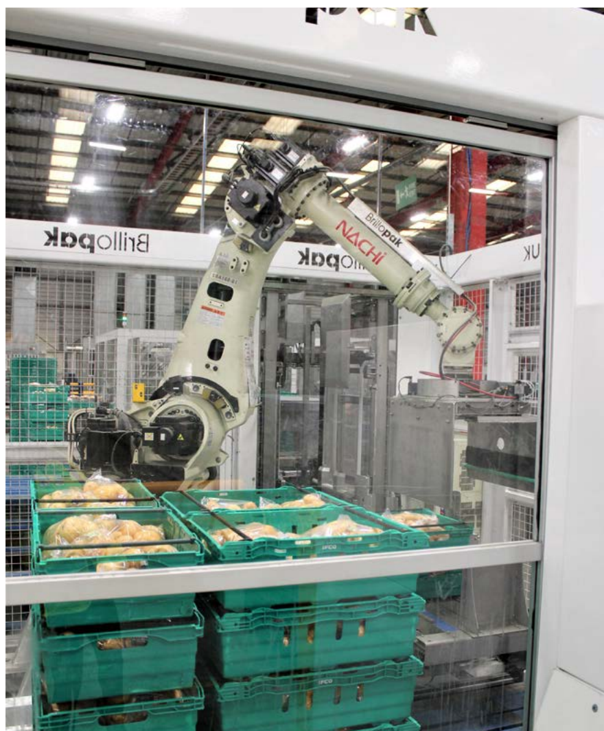
Robot palletisers handle the heavy lifting and stacking of crates
