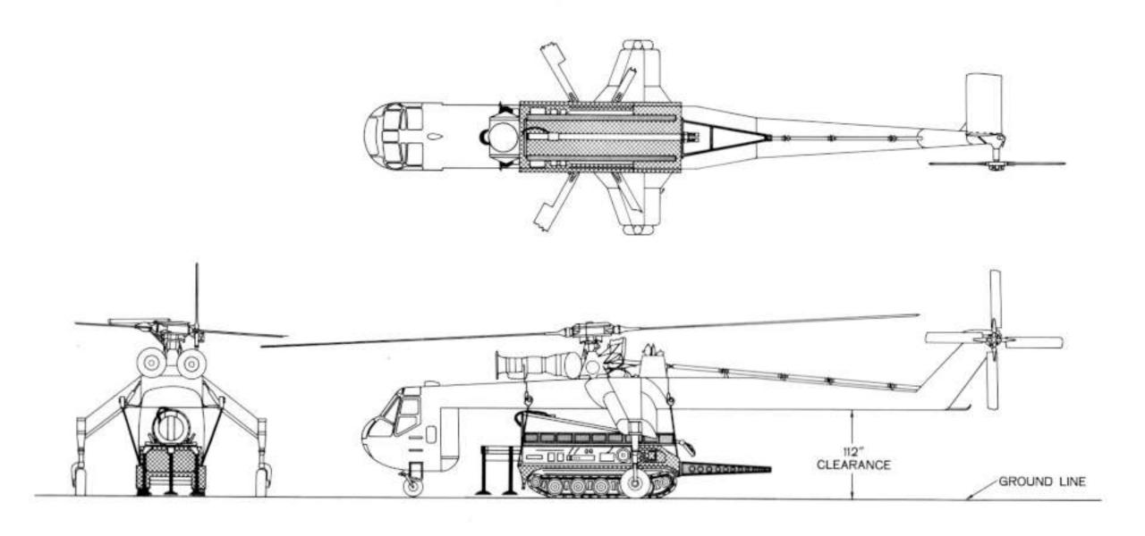
XM474E2 TRACKED CARRIER WITH T.E.L. ERECTOR LAUNCHER
