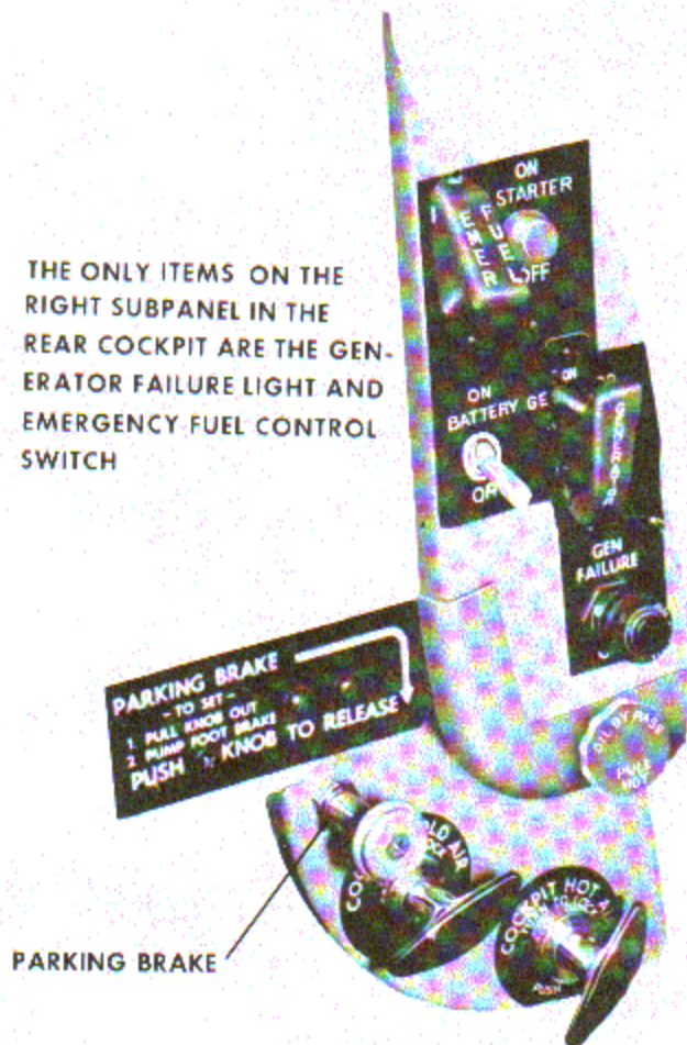
Figure 1-15. Right Subpanel Front Cockpit
